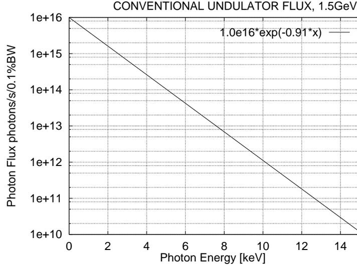
**Figure 8.2.1:** Fit to flux from conventional wiggler<sup>13</sup> operating with 5 mm gap and beam energy  $E = 1.5$  GeV. The straight line crudely approximates 8 diffraction maxima in the range up to 10 keV and extrapolates to 15 keV. Integrating over the distribution given in the key yields a total beam power  $\mathcal{P} \approx 10^{19}$  keV/s.
