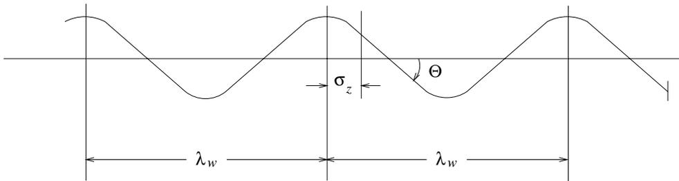
**Figure 6.2.1:** The electron orbit through the undulator is treated as a sequence of impulses, each bending through  $2\Theta$ . In the “ideal undulator limit”,  $\Theta = K/\gamma \ll 1/\gamma$ , i.e. small compared to the half-angle of a cone containing most of the synchrotron radiation.
