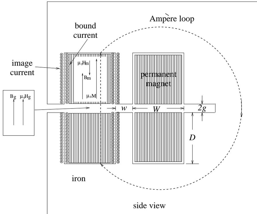
**Figure 7.5.1:** Two adjacent permanent magnet sections, separated by an iron pole, are shown. The Ampère loop links the “bound” current of the permanent magnet and the “image” current in the iron, but no “free” current.
