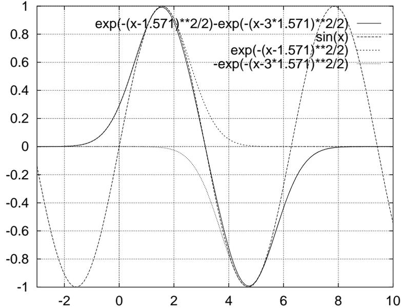
**Figure 6.2.2:** Plot illustrating a sinusoid matched by a series of alternate sign Gaussians, of which only two are shown. See key in upper right for analytic forms. The standard deviations are related to undulator wavelength by  $2\pi\sigma_z = \lambda_w$  in order to match curvatures at the peaks. Though the true trajectory is sinusoidal, radiation integrals will be based on the Gaussian pulses, so radiation deficiency or excess from the tail regions will require (modest) correction.
