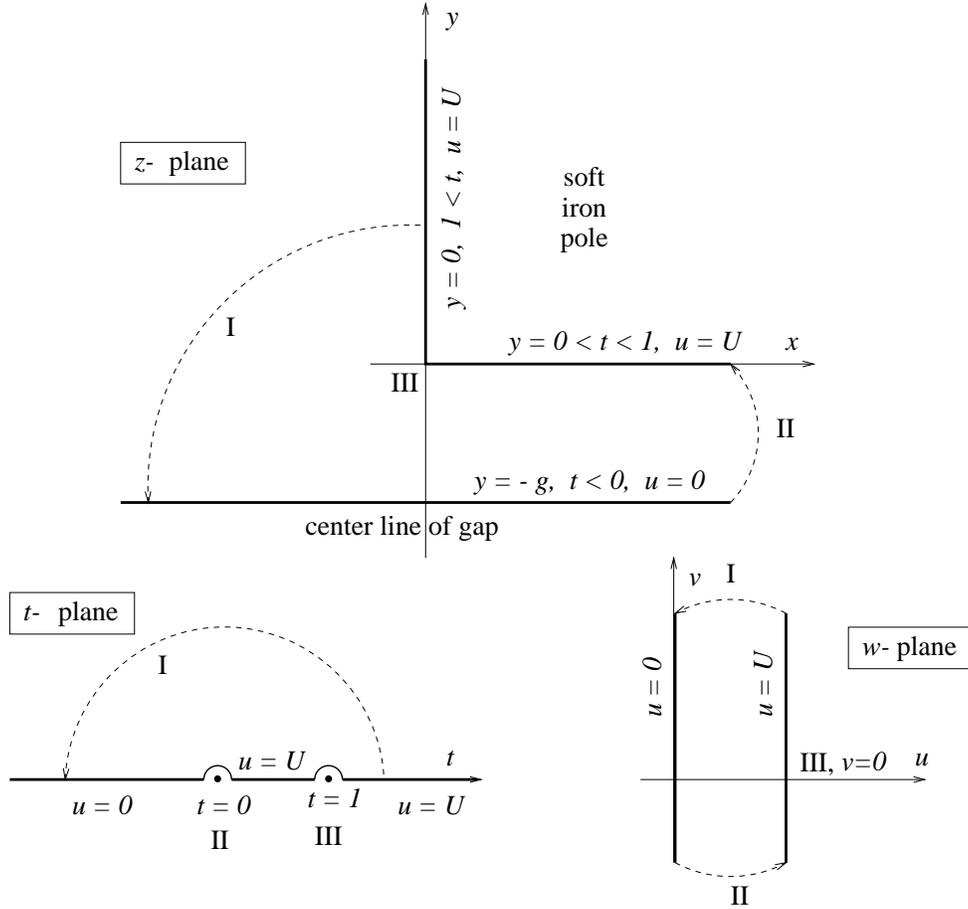
**Figure 7.4.1:** Complex planes used to determine the magnetic field in the region between one half pole and the centerline of the gap. At point III, the corner of the pole,  $t = 1$  and  $x = y = v = 0$ .
