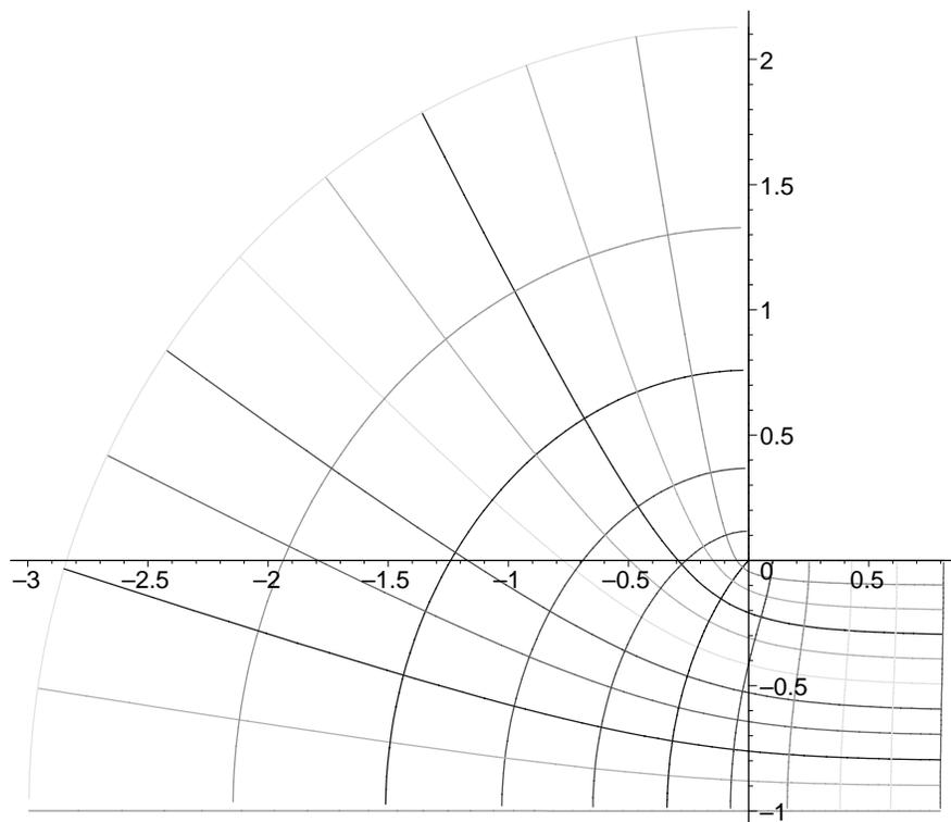
**Figure 7.4.3:** Field plot for the ranges  $0 < u < 1$ ,  $-1 < v < 1$ . By the spacing between curves of constant  $v$  the field magnitude at  $(0, 2g)$  is roughly one fifth of the field in the gap. This suggests that  $D/g$  should be at least 2 or  $g/D$  should be less than 0.5.
