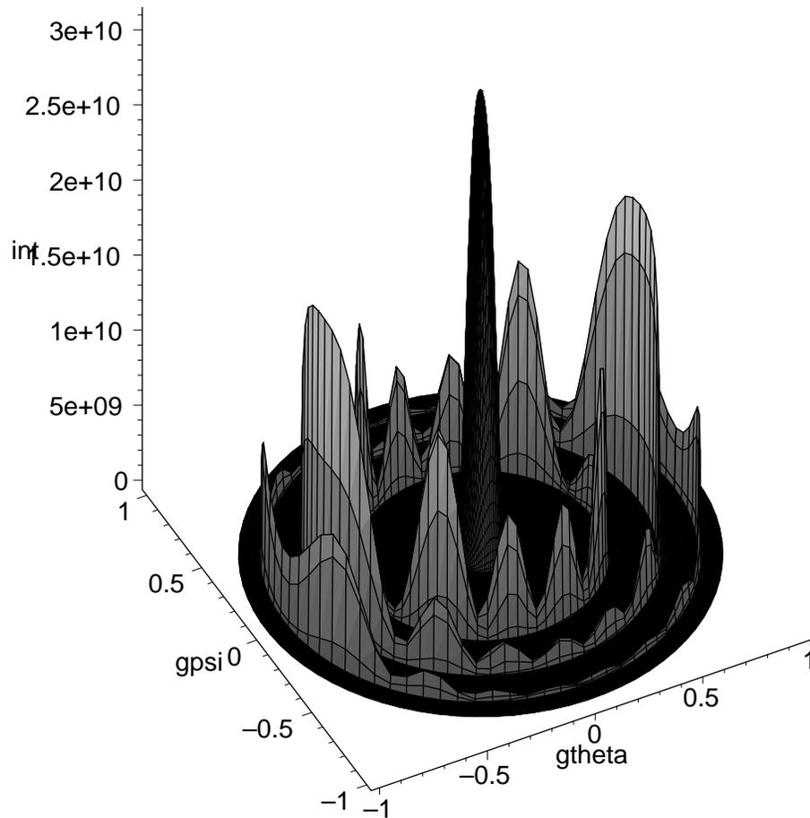
**Figure 6.8.1:** Spectrum for published ESRF configuration as recalculated using Eq. (6.6.4). Physical parameters were  $E = 6$  GeV,  $N_w = 20$ ,  $\lambda_w = 46$  mm,  $E_\gamma = 27$  keV. Computational parameters are  $N_w = 19$ ,  $i_{\max} = 14$ ,  $n_{\text{mono.}} = 7$ . This result can be directly compared with another calculation: [www.esrf.fr/machine/support/ids/Public/CentralCone/CentralCone.html](http://www.esrf.fr/machine/support/ids/Public/CentralCone/CentralCone.html)
