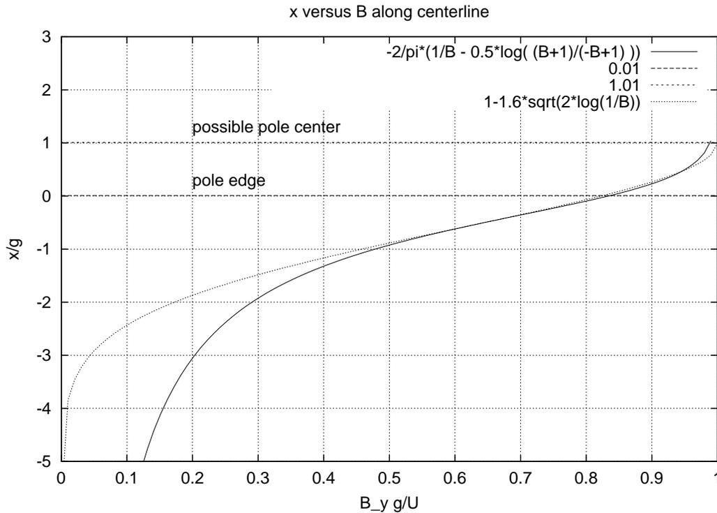
**Figure 7.4.4:** Magnetic field profile along the centerline due to one half pole. The pole edge is at  $x = 0$ . The pole width can be as little as  $2g$  (the case shown) with only 2% field reduction from the nominal (thick pole) value. Also shown is a Gaussian fit that applies for this particular choice of pole width.
