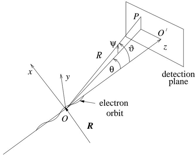
**Figure 6.2.3:** Orbit geometry and definition of horizontal angle  $\theta$  and vertical angle  $\psi$  locating the detector position  $P$  relative to the  $t = t_r = 0$  orbit position.
