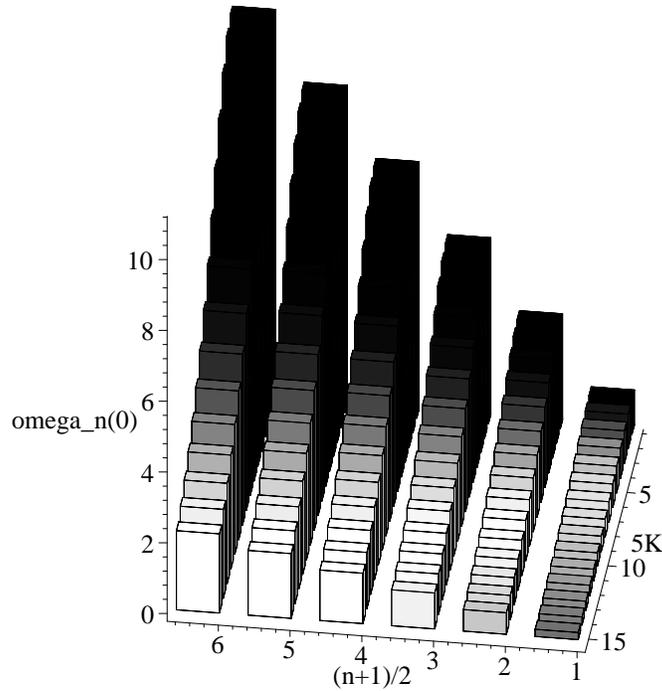
**Figure 6.5.3:** Histograms illustrating the dependence of undulator frequency (indicated by tower height) and intensity on resonance (indicated by tower grayscale) on undulator parameter  $0 < K < 3.0$  and resonance order  $n = 1, 3, 5, 7, 9, 11$ . The grayscale is the same as in Fig. 6.5.1 and is normalized to 1 (white) in the lower left hand corner. Black regions have negligible flux.
