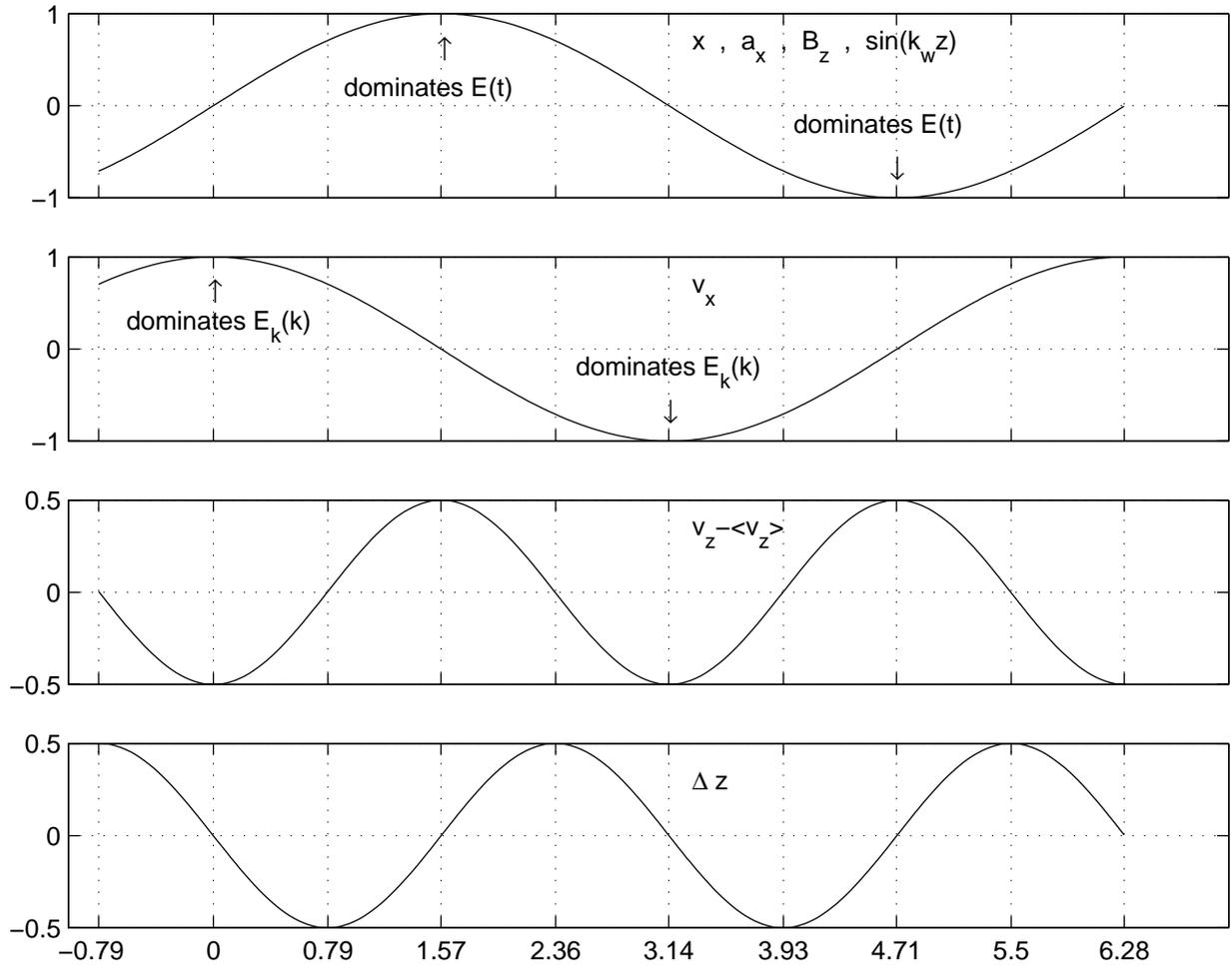
**Figure 6.4.1:** Graphs showing the correlations among various quantities as a function of longitudinal position in the undulator. Vertical scales can be reconstructed using formulas in the text.
