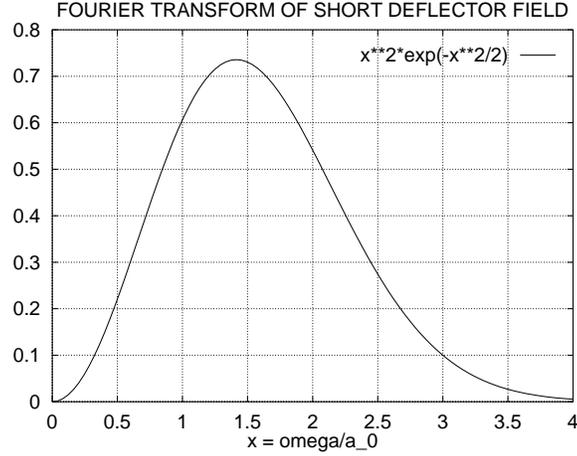
**Figure 6.2.4:** Fourier transform (Eq. (6.2.25)) of deflecting force due to a short Gaussian deflecting element for  $\vartheta = 0$ . The horizontal axis is  $\omega/a_0$ . According to Eq. (6.2.25), the spectral shape for  $\vartheta \neq 0$  is the same, provided the horizontal axis is interpreted as  $\omega/a_\vartheta$ .
