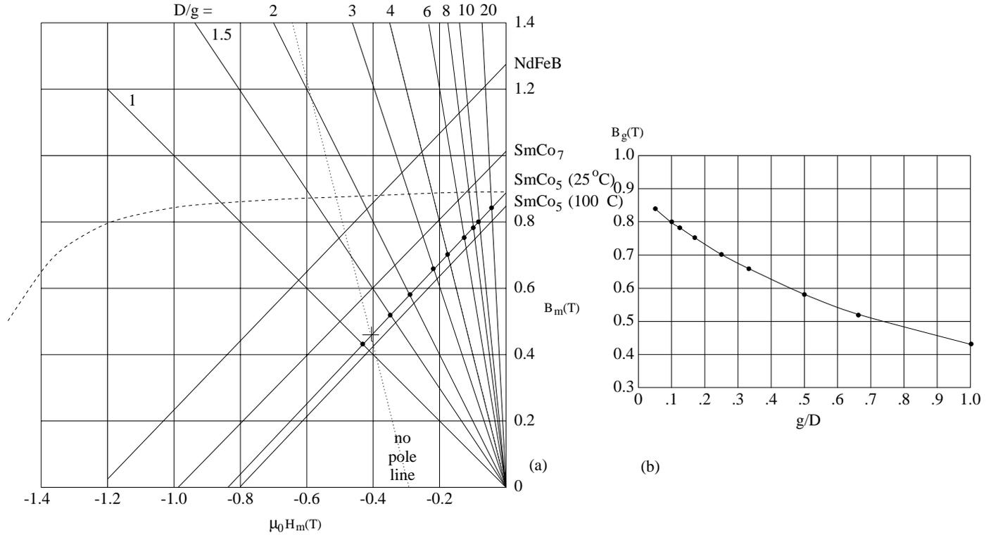
**Figure 7.5.2:** (a) Demagnetization curves for various permanent magnet materials. From P. Campbell, *Permanent Magnet Materials and Their Application*, Cambridge University Press, 1994. Also shown are load lines given by Eq. (7.5.2) and their intersections with the  $\text{SmCo}_5$  load line for various values of  $D/g$ . The dashed curve gives the magnetization  $\mu_0 M$ . (b) The corresponding dependence of  $B_g$ , the field in the gap, on  $g/D$ .
