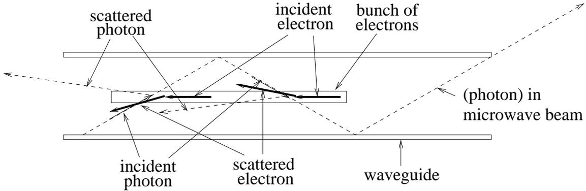
**Figure 8.1.2:** Microwave undulator configuration. An electron beam collides with a traveling (or standing) microwave beam. The microwave beam can be thought of as a superposition of plane waves that reflect repeatedly off the conducting walls of the waveguide.
