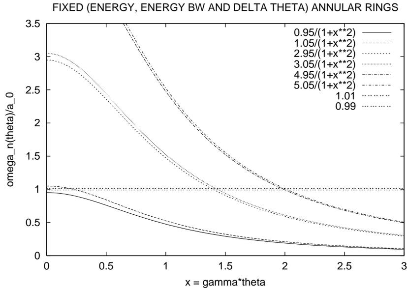
**Figure 6.3.1:** The photon flux into a detector having fixed central energy, fixed energy acceptance and full angular acceptance is proportional to the areas of the little parallelograms whose sides are contours of constant  $n$  resonance (Eq. (6.2.33)) and whose bottoms and tops are contours of constant photon energy. There is no significance to the solid, broken, etc. curves other than to correlate with the mathematical form shown in the key.
