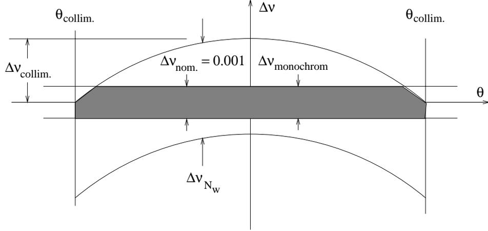
**Figure 6.3.3:** In the  $\nu_J, \vartheta$  plane apertures are defined by monochromatization, by collimation, and by the undulator characteristics (i.e. number of poles  $N_w$ .) For the relative sizes of these apertures suggested in the text as typical, useful photons populate the shaded region.
