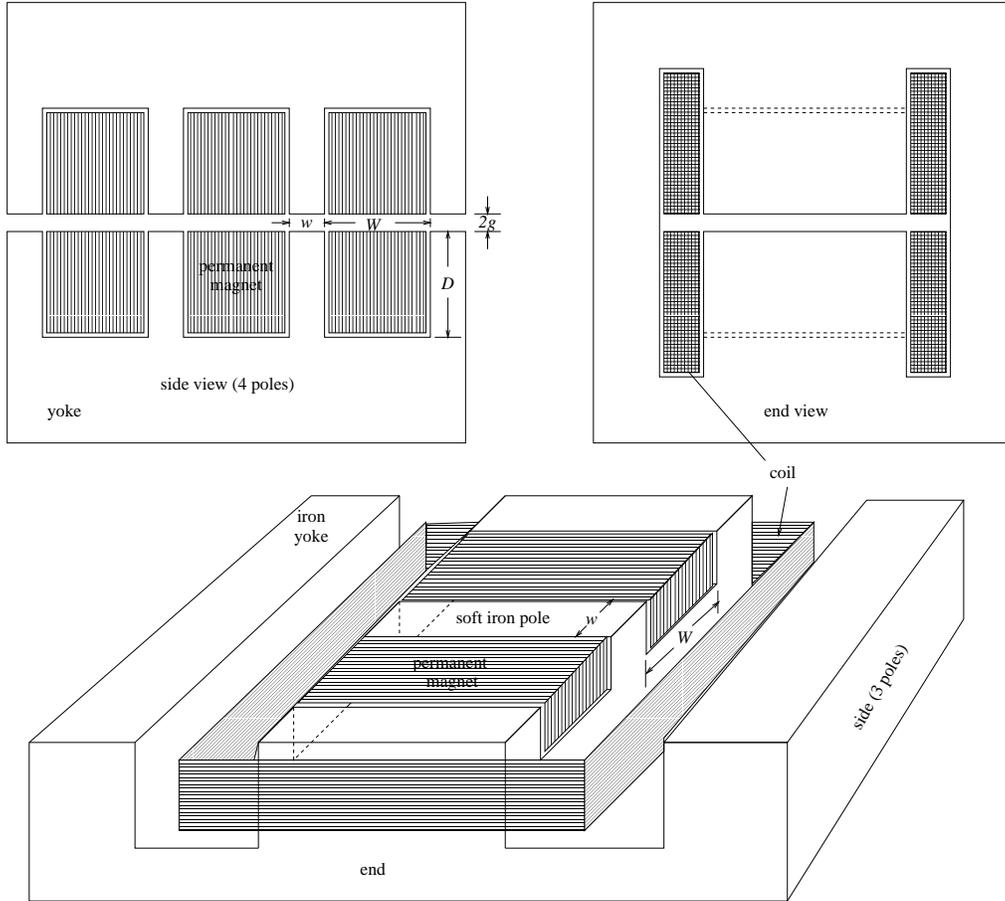
**Figure 7.1.1:** Schematic illustration of coil, yoke, and permanent magnetic material in a hybrid, electro-/permanent-magnet, asymmetric undulator. The mechanism to vary the gap height  $2g$  is not shown; it will represent quite a design challenge.
