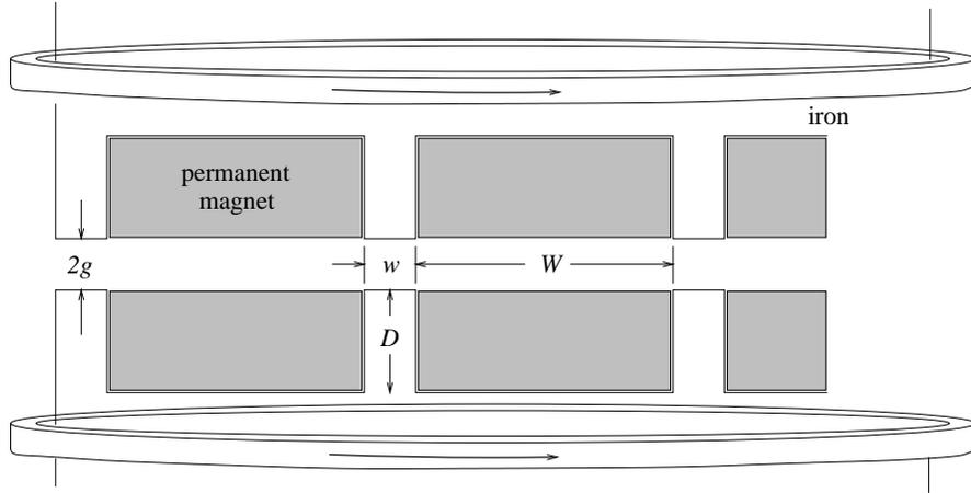
**Figure 7.6.1:** Pole profile of the asymmetric undulator. The relative dimensions shown are a tentative starting point for a more careful analysis that accounts for the interaction of electro and permanent magnet effects. The electromagnet coils are shown schematically only as a reminder of their presence.
