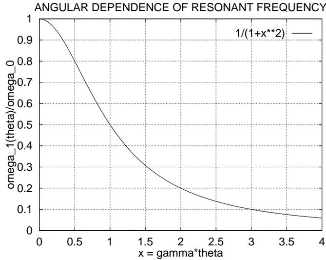
**Figure 6.2.6:** Angular dependence  $\omega_1(\vartheta)|_{K \ll 1}$ , the frequency of the fundamental undulator line with  $K \ll 1$ . The horizontal axis is  $\gamma\vartheta$ . Some people refer to this as a “Doppler shift”, based on an analysis in which the radiation is first evaluated in the rest frame of the electron, and then transformed to the laboratory frame.
