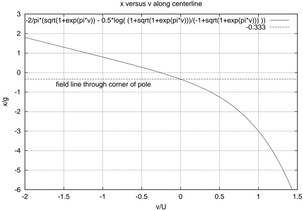
**Figure 7.4.2:** Relation between  $x$  and  $v$  along the centerline. Note that the  $v = 0$  contour (the one leaving the corner of the pole) intersects the centerline at a slightly negative value of  $x = -0.333g$ . As  $v$  becomes more positive, the constant  $v$  contour bulges out more and more (i.e.  $x$  becomes increasingly negative.)
