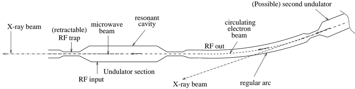
**Figure 8.1.1:** Microwaves in the “undulator” collide with circulating electrons. The useful microwaves propagate approximately anti-parallel to the electrons.
