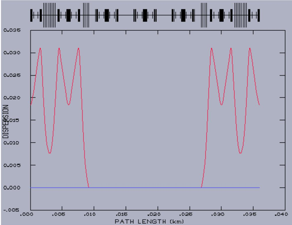
**Figure 8.3.1:** Six consecutive minimum emittance cells, with the second and fifth cells modified to provide zero dispersion in the third and fourth cells. Bending magnets, quadrupoles, and sextupoles are indicated by long medium and short hatch marks in the schematic above the graph.
