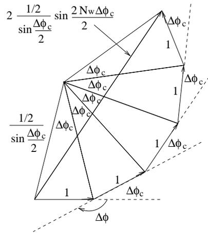
**Figure 6.2.7:** Phasor diagram with  $2N_w$  arrows to calculate the coherent sum of waves from  $2N_w$  sources, or  $N_w$  undulator periods. The directions of alternate phasors are reversed to account for the half period phase shift.  $\Delta\phi_c = \pi - \Delta\phi$  where  $\Delta\phi$  is the phase advance per half period of the undulator. Though  $2N_w$  is necessarily even, the total number of deflections can actually be odd, as in the figure,
