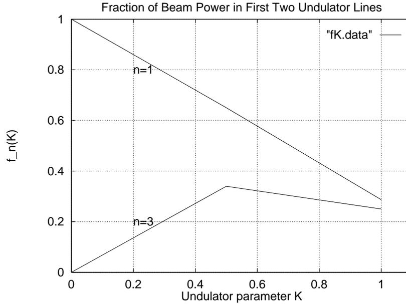
**Figure 6.9.1:** Plot of  $f_1(K)$  and  $F_3(K)$ , the fraction of power radiated into the first two undulator lines, as a function of undulator parameter. Crudely extracted from figure 3 of the Wiedemann article in the Chao-Tigner handbook. ( $f_1(K)$  has a different meaning in that article, and it is possible I am misinterpreting the data.)
