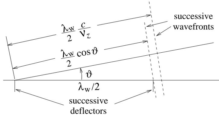
**Figure 6.2.5:** Geometry illustrating the condition for interference maxima observed at vertical angle  $\vartheta$ .
