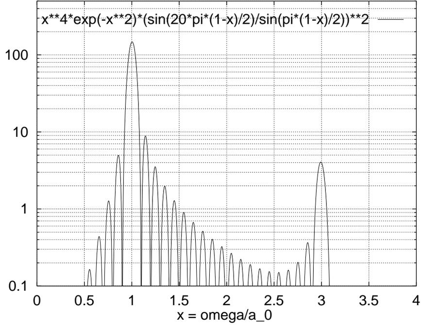
**Figure 6.2.8:** Energy spectrum for  $N_w = 10$  undulator periods, with  $\vartheta = \Theta = 0$ . The horizontal axis is  $\omega/a_0$ .
