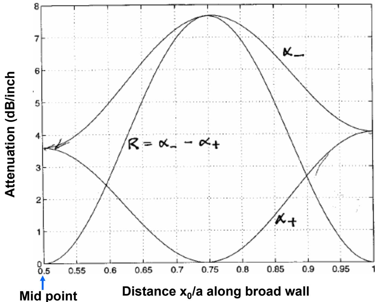
The maximum reverse attenuation  $\alpha_-$  is approximately 7.75 dB/inch. Thus the necessary ferrite length is  $L = 25\text{dB} / 7.75\text{dB/in} = 3.23''$
