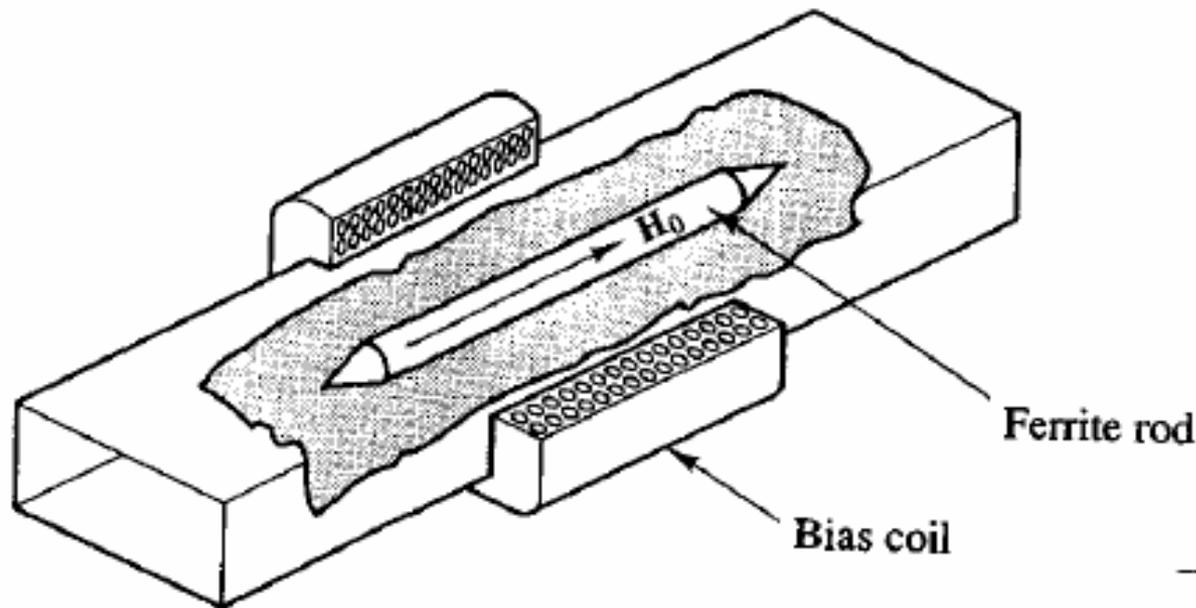
Reciprocal phase shifters are required in scanning antenna phase arrays used in radar or communication systems, where both transmitting and receiving functions are required for any given beam position. The Reggia-spencer phase shifter is such that a reciprocal device. The phase delay through the waveguide is proportional to the d.c. current through the coil, but independent of the direction of the propagation through the guide.
