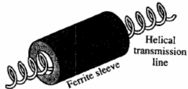
Ferrite loading of helical T.L.
