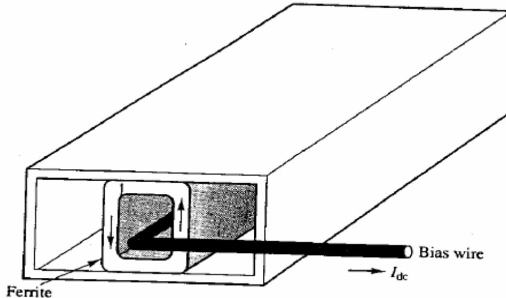
Or a simpler version using 2 ferrite slabs:
