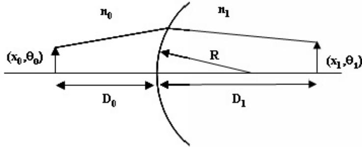
FIGURE 19. Quantities used in the relations for refraction at and indexed boundary
