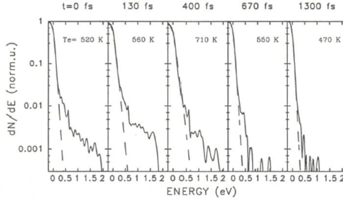
Fig. 1: Electron energy distribution function vs. energy with  $120 \mu\text{J}/\text{cm}^2$  absorbed laser fluence at 5 time delays. The dashed line is the best Fermi-Dirac fit and the corresponding electron temperature,  $T_e$ , is shown. The vertical scale is in units of density of states.
