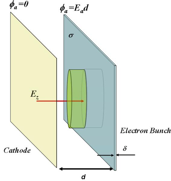
FIGURE 20. The cathode and electron bunch shortly after emission. The electron bunch is typically 10's of microns long when the laser pulse ends and the last electron is emitted.  $d$  is the distance from the cathode to the tail of a bunch which is  $\delta$  long.
