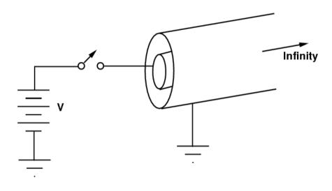
Take an infinitely long coaxial cable and suddenly apply a voltage V to it. A current I
