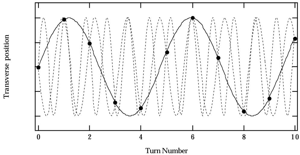
The above shows a simplified betatron oscillation around a ring and the bar shows that sampled transverse position at a single point in the ring. The lower picture shows the sampled signal (as dots) and that an infinite series of frequencies fits the sampled data. This set of frequencies corresponds to the set of upper and lower sidebands of the rotation harmonics observed on a spectrum analyzer.
