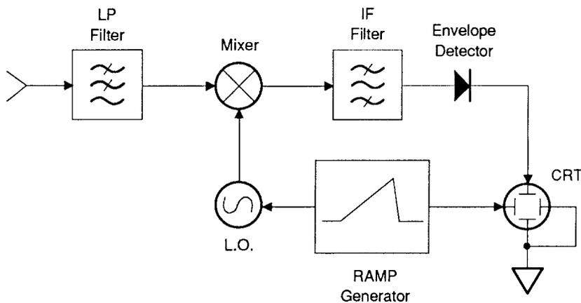
The analog spectrum analyzer works by demodulating a high frequency signal, similar to the operation of a simple car radio. However, the spectrum analyzer has much more control over the demodulation process. For example, a less simplified diagram of the spectrum analyzer shown below has multiple LO stages, each with its own IF filter of variable bandwidth.
