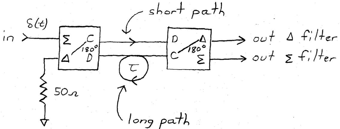
If  $\tau$  is the difference in time delays between the two cables connecting the hybrids, the impulse responses of the  $\Sigma$  and  $\Delta$  filters, apart from an overall time delay, are given by:
