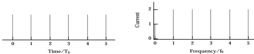
(Negative frequency components can be folded onto positive frequency. AC components are 2X DC component.)
