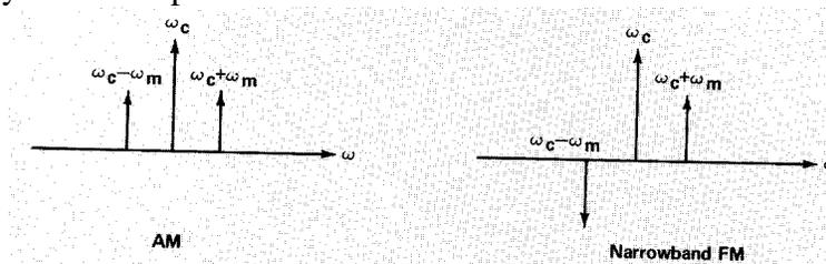
The relative phase of the upper and lower sidebands for the PM results from the choice of the phase of the modulation (i.e.  $\sin$  rather than  $\cos$ ).
