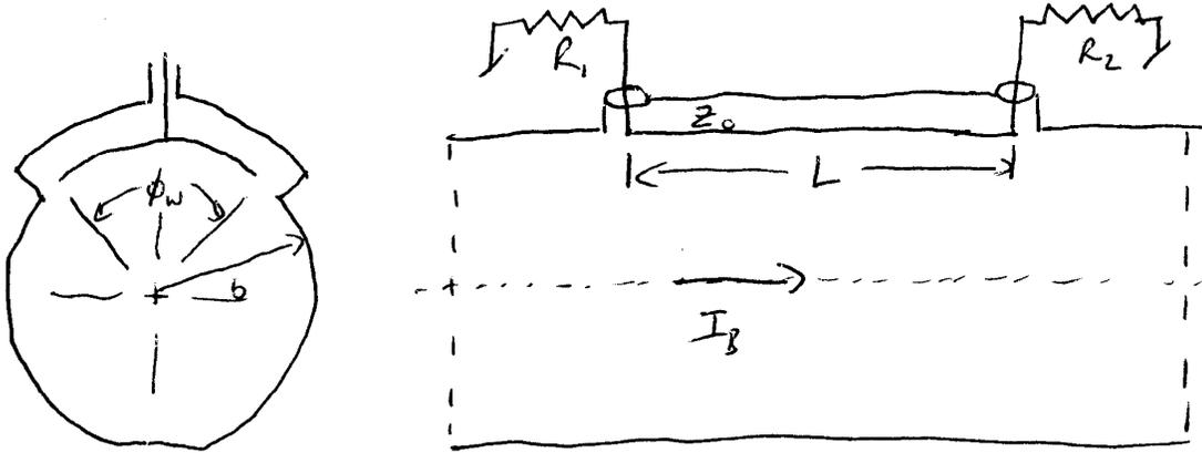
Assuming that the upstream terminal impedance  $R_1$  is matched to the stripline impedance  $Z_0$ , half of the current exits the upstream ( $gI_b/2$ ) terminal and half travels down the stripline with velocity  $c$ . As the beam passes the downstream port, the current on the inner electrode plate,  $-gI_b$ , combines with the current of the outer side of the plate. A current of  $-gI_b/2$  travels back towards the upstream port and exits.
