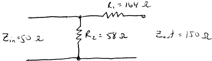
One of the disadvantages of resistive matching is that the signal levels can be considerably attenuated by the resistors, complicating the analysis. However, impedance transformers are somewhat impractical at lower frequencies where resistive matching is ideal. The attenuation for the resistive matching at ports 1 and 2 has been found to be  $A_1=0.14$  and  $A_2=0.54$ .
