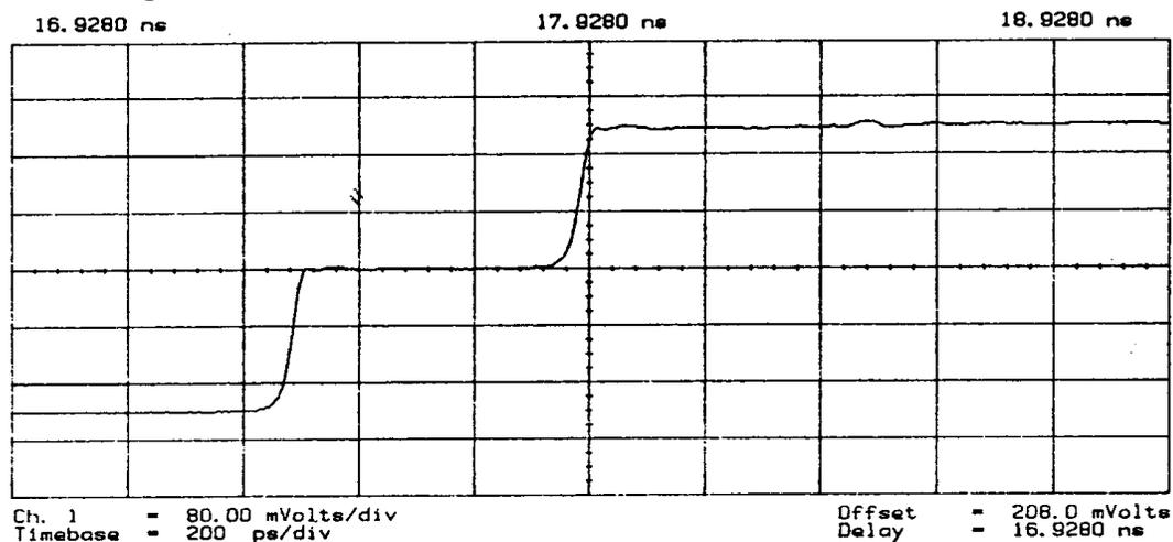
Note the position (in time) of the incident step and the reflected step coming from the open circuit at the output of the step generator. Connect a length of 50Ω cable (cable "A"), open circuited at one end. The step now travels along the length of the cable, is reflected by the mismatch at the (open circuit) end of the cable, and travels back into the sampling head where it is detected. The timebase should be about 1 ns/div to get the display on screen, then 500 ps/div for the measurements.
