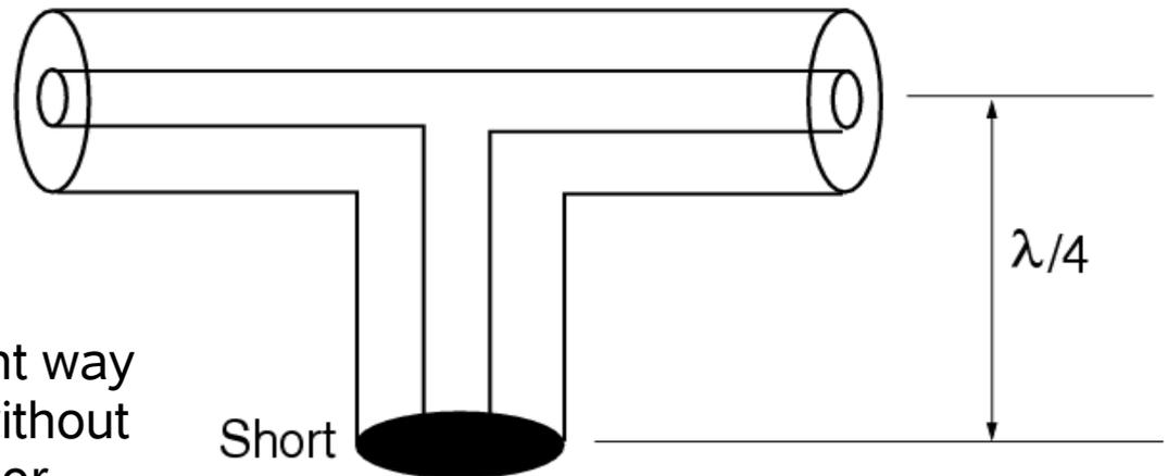
A quarter-wave stub is a convenient way of supporting an inner conductor without an insulator, and accessing the inner conductor with water cooling, for example.
