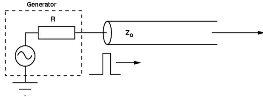
Even though the transmission line itself has no ohmic resistance, a definite current  $I$  is measured passing into the line by during the period of the pulse with voltage  $V$ .
