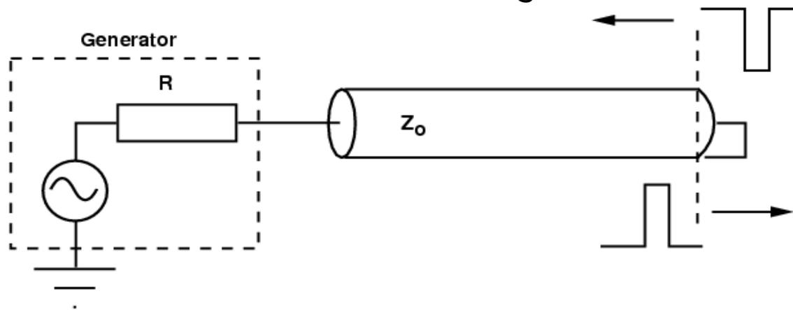
If the time it takes to propagate the pulse down the line is  $t_p$ , then the inverted pulse arrives back at the generator at time  $2 t_p$ .
