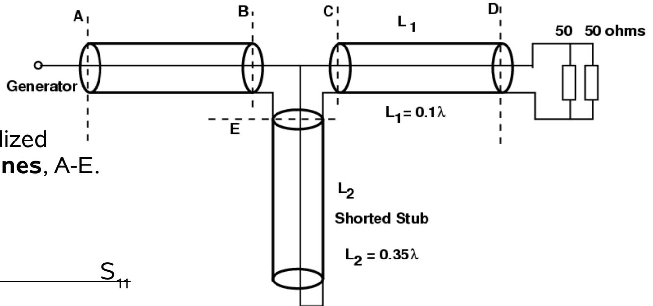
This problem can be broken down to calculating the normalized impedance at 5 **reference planes**, A-E.
