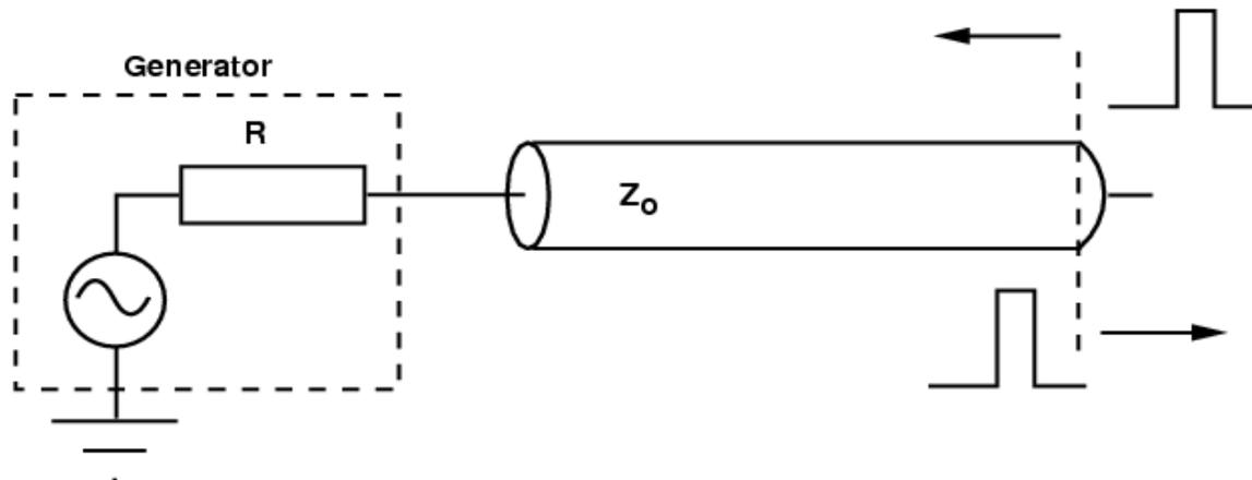
Imagine the two pulses overlap as two batteries of identical voltage:
