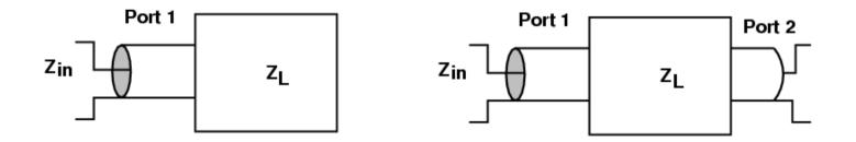
A wave may enter a port and be reflected back from that port, or may be transmitted through the DUT and exit from the other port.
