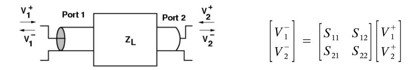
Note that currents are not involved directly, but inferred from the impedance of the network analyzer, the cables and the terminations, normally 50 ohms.
