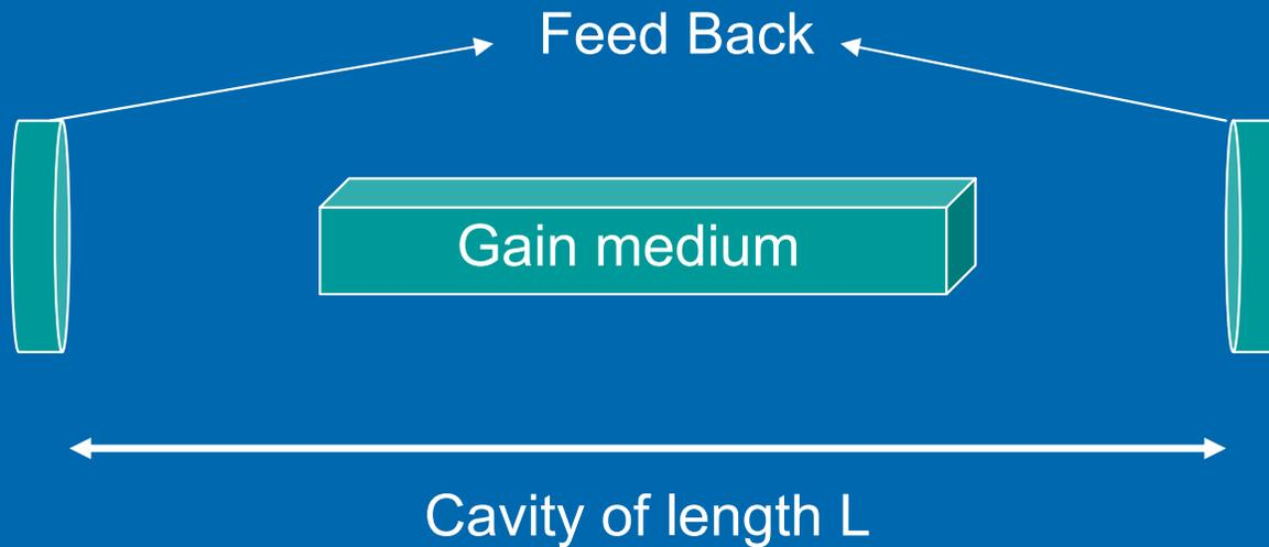
Cavity supports transverse (spatial profile) and longitudinal (frequency spectrum) modes
