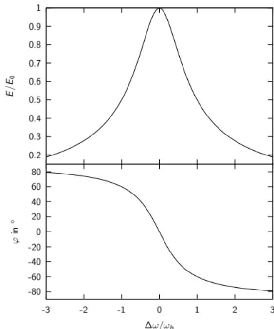
$$E(\omega) = \frac{E_0}{\sqrt{1+4Q_L^2\left(\frac{\omega-\omega_0}{\omega_0}\right)^2}}$$
