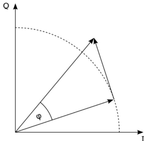
$$\begin{pmatrix} I' \\ Q' \end{pmatrix} = \left[ \begin{pmatrix} 1 & 0 \\ 0 & 1 \end{pmatrix} + p_{\text{err}} k_p \begin{pmatrix} 0 & -1 \\ 1 & 0 \end{pmatrix} \right] \begin{pmatrix} I \\ Q \end{pmatrix}$$
