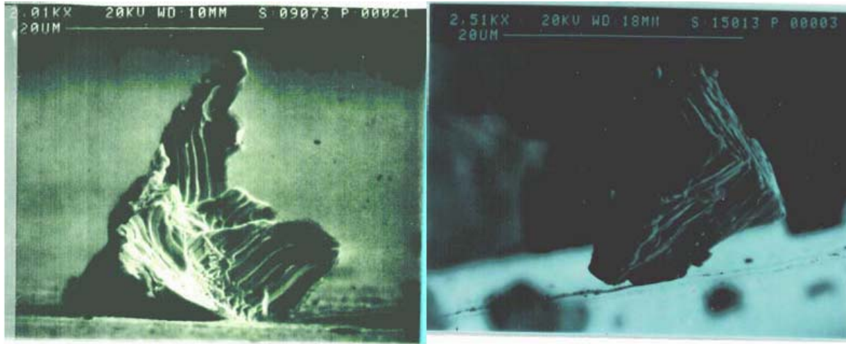
Fig. 11 Example of a scratch and a particle on a niobium surface.
