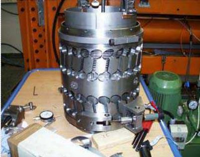
*Blade tuner occupies no beam line space: it is mounted on top of the He vessel. Can be used where beam line real estate is at premium.*
