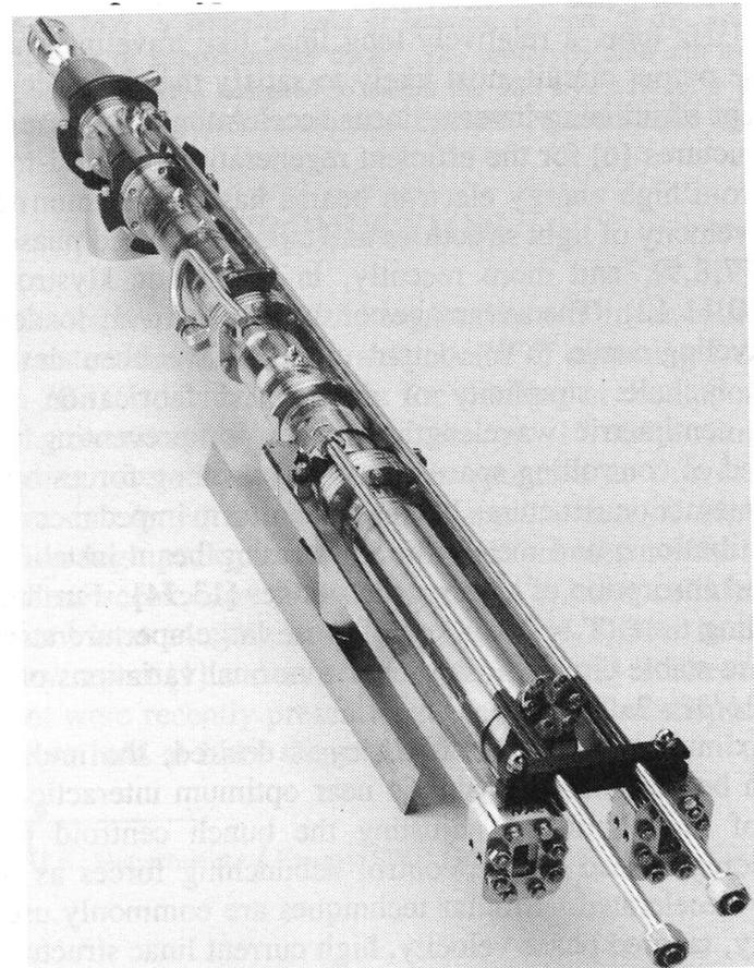
**FIGURE 1.** Model X7100 17 GHz TWRK showing the WR62 rectangular waveguide and body water-cooling connections, and the high vacuum port for the independently pumped, electrically isolated beam collector.
