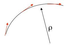
In beam physics, we are generally interested in deviations from the reference trajectory. Therefore it is most convenient to place the coordinate system origin on the reference trajectory, and align one (the longitudinal) coordinate axis with the reference trajectory. Remaining (transverse) axes are chosen perpendicular to the longitudinal axis.
