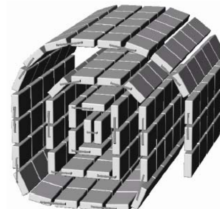
Solid model of the 500 kV hard switch – note the spiral wrap of the series string of switch modules to reduce effective parasitic capacitance. The output (pulsed) end of the modulator is on the axis, and the input (DC) end is on the outer surface.
