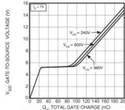
Figure 7, Gate Charge vs Gate-to-Source Voltage
