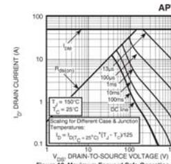
Figure 10, Maximum Forward Safe Operating Area
