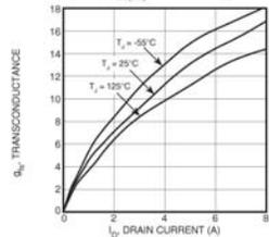
Figure 5, Gain vs Drain Current
