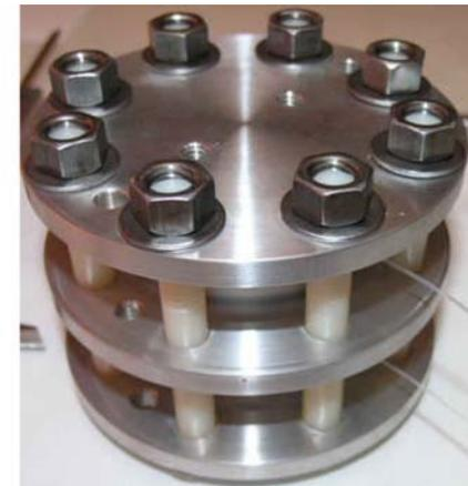
Fig. 4. Photograph of Two-Switch Electrode assembly.
