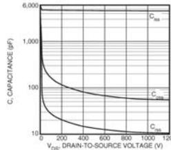
Figure 6, Capacitance vs Drain-to-Source Voltage
