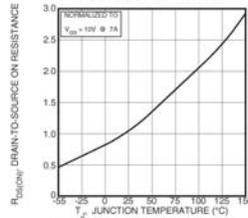
Figure 3,  $R_{DS(on)}$  vs Junction Temperature
