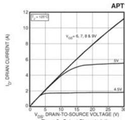
Figure 2, Output Characteristics
