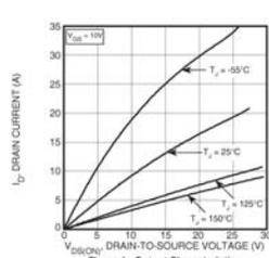
Figure 1, Output Characteristics
