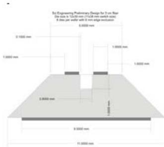
Fig. 2. End view drawings of optical thyristor
