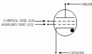
Figure 1. Thyratron with auxiliary grid (heater detail not shown)
