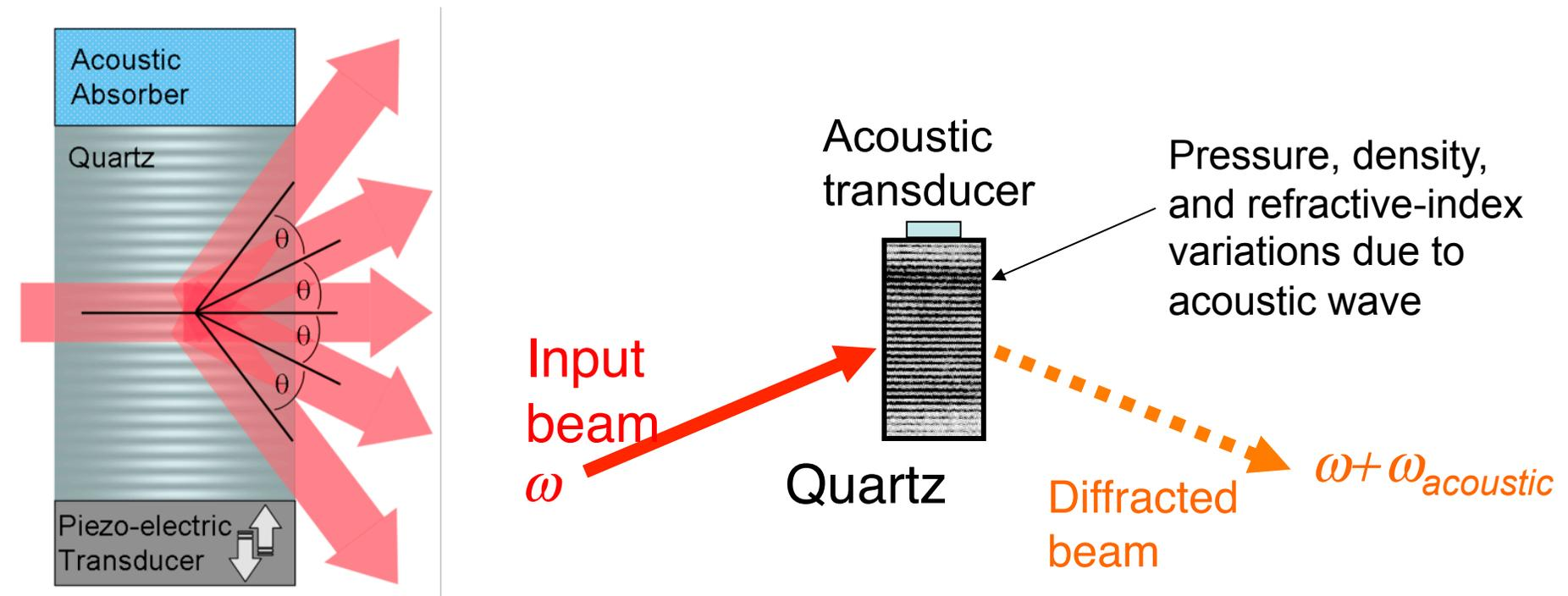
Acousto-optics works because acoustic waves have about the same wavelengths as (visible) light waves. Such diffraction can be quite strong:  $\sim 70\%$ . Acousto-optics is the basis of useful devices.
