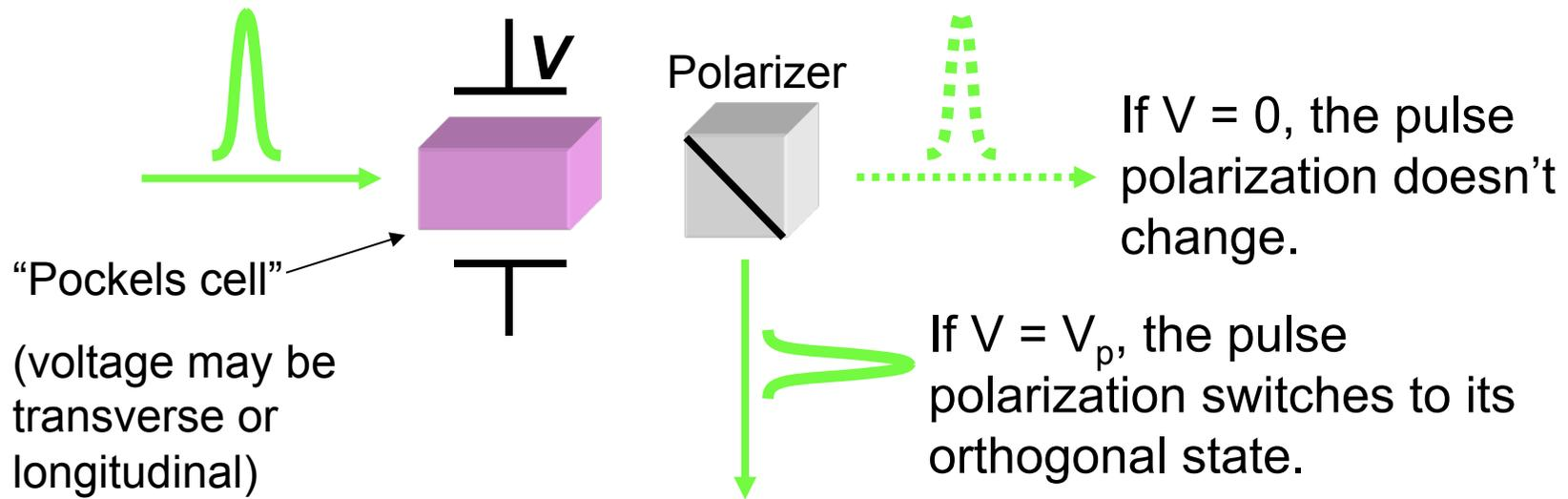
Abruptly switching a Pockels cell allows us to switch a pulse into or out of a laser.
