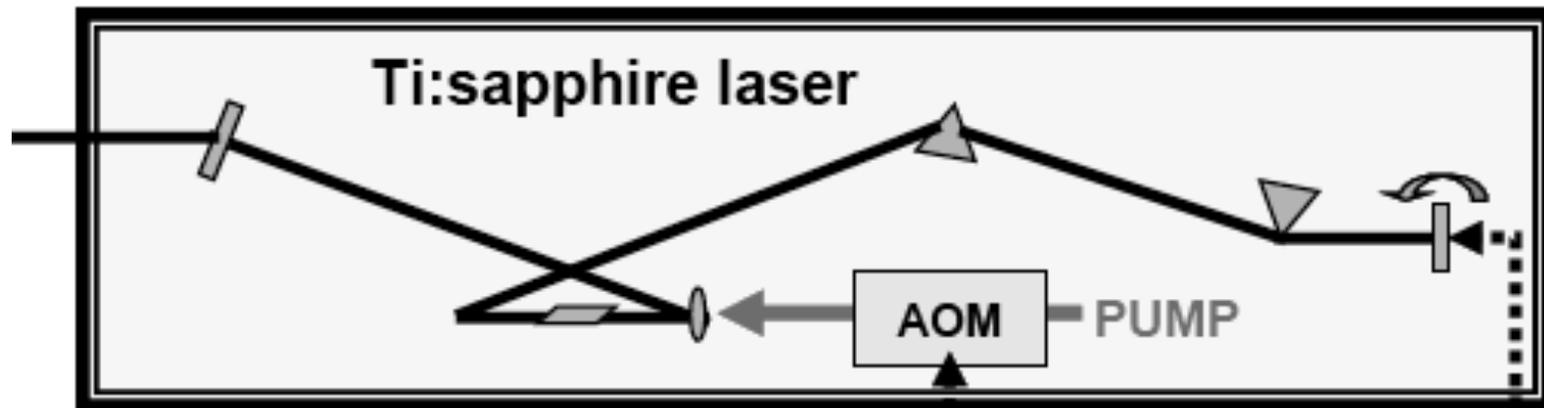
Repetition rate given by round trip travel time in cavity. Modulated by piezo adjustment of cavity mirror.
