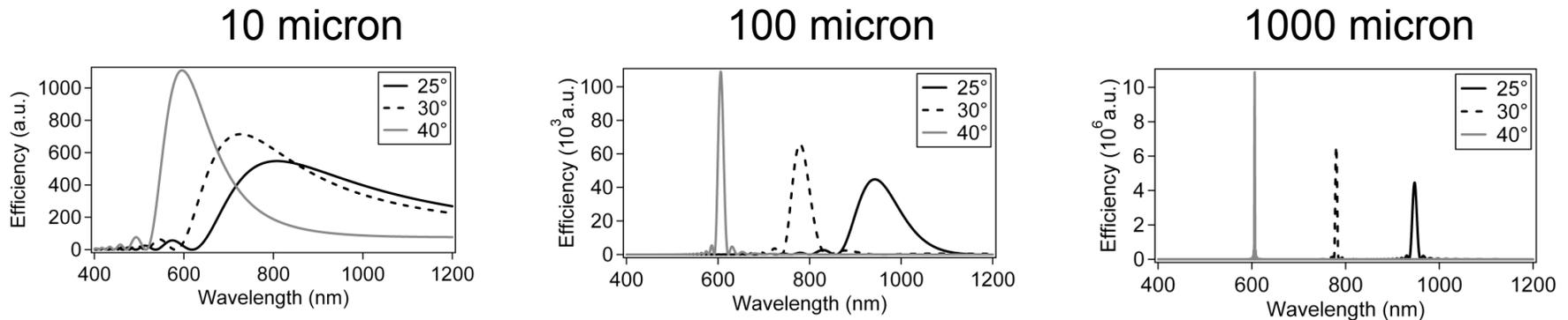
Note the huge differences in phase-matching bandwidth and efficiency with crystal thickness.
