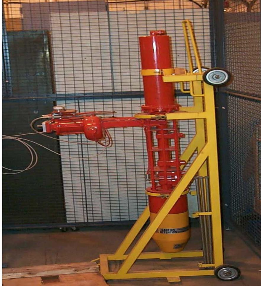
**S-Band 35 MW Klystron (TH2128)**
