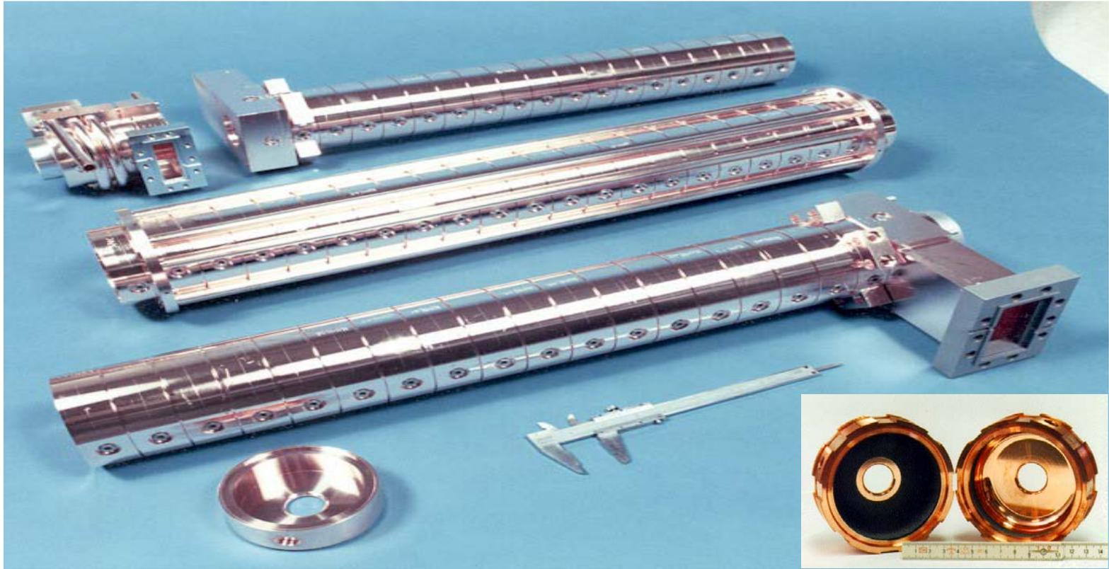
Disk-Loaded Constant Gradient S-Band Structure
