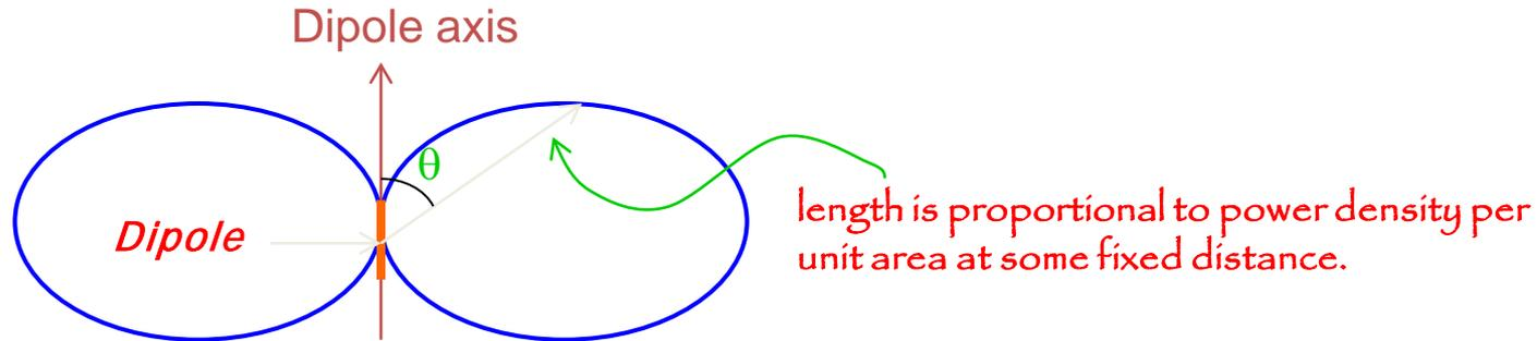
Note: No radiation takes place along the dipole axis, and the radiation pattern has axial symmetry, with maximum radiation being in the equatorial plane.
