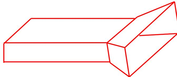
Waveguide fed horn
