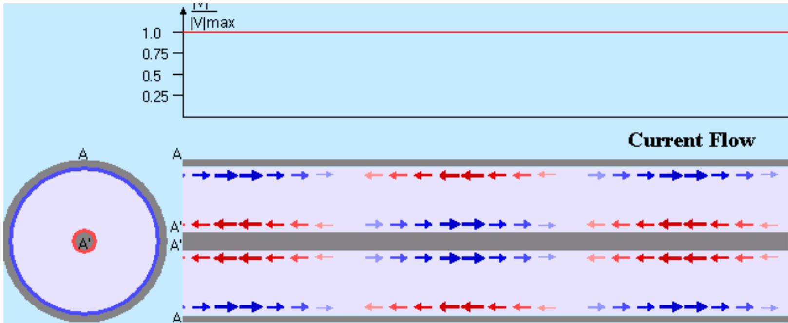
Surface current in coaxial line. Orientation depends on phase - position along the line.
