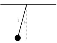
A pendulum is made up of a massless rigid rod of length l, and a bob of mass m. The equation of motion of the pendulum bob swinging in a gravitational field is  $\tau = -\vec{r} \times \vec{F} = I \frac{d^2\theta}{dt^2}$ , which may also be written  $-l \sin \theta m g = m l^2 (\frac{d^2\theta}{dt^2})$ , where the moment of inertia is  $I = m l^2$  since the rod is massless. Then the equation of motion is  $\ddot{\theta} + \frac{g}{l} \sin \theta = \ddot{\theta} + \omega_0^2 \sin \theta = 0$ .
