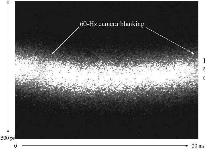
Bowed envelope: 60-Hz harmonic on the trigger?
