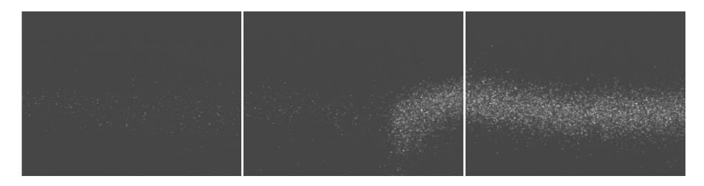
After first injection. Dim image:  $\approx 0.1$  mA in bunch. Second injection enters, a bit late in phase.
