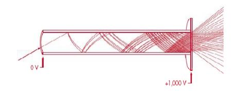
Fiber coupling from fluorescent screen to CCD
