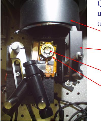
Quick proof-of-principle test in 2004, using the PEP-II low-energy ring and an ordinary supermarket scanner.
