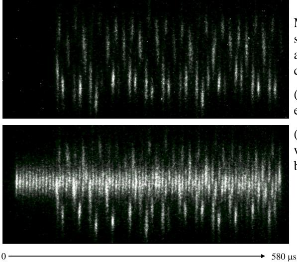
Minor-axis projection showing injected charge arriving on the 13th of 80 consecutive turns.
