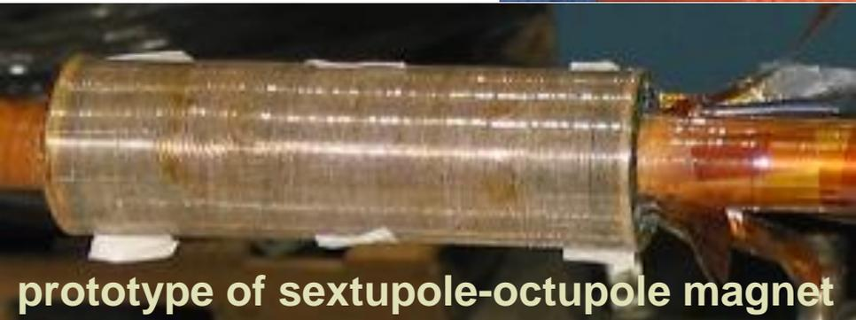
prototype of sextupole-octupole magnet
