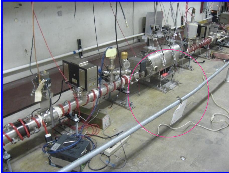
Newly built and installed (Summer 2009) vertical goniometer at E0. It is ~ 4m upstream of the Horizontal one.
