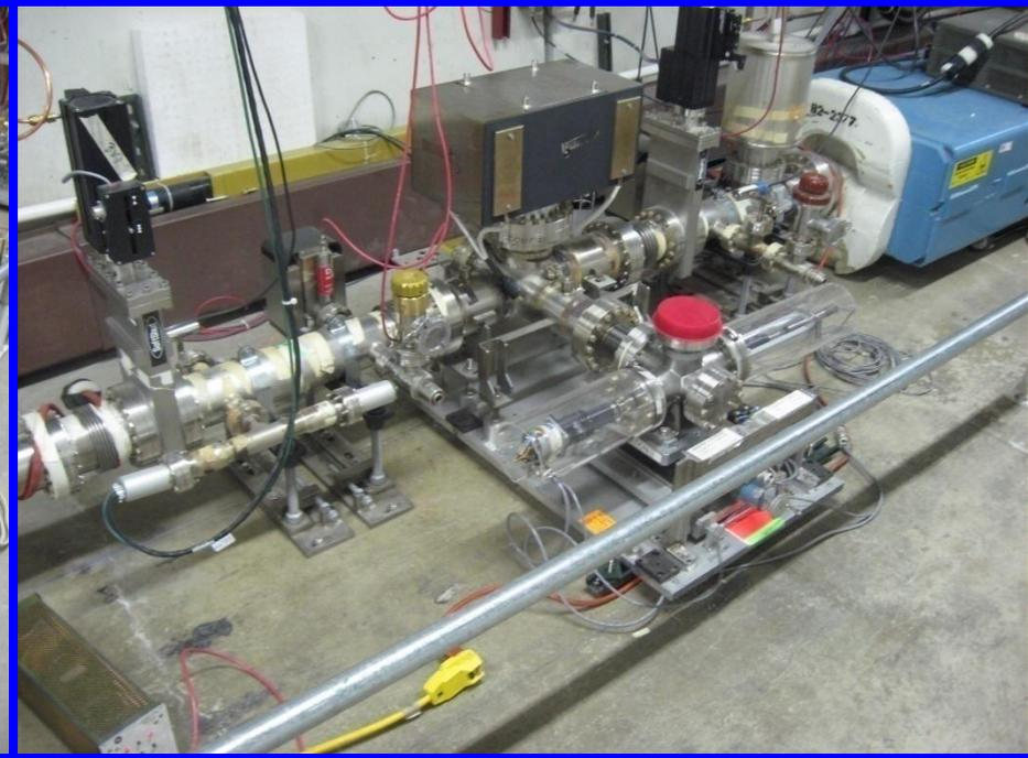
Modified horizontal goniometer. Replaced old large miscut positive angle O-shaped crystal with new small negative miscut angle O-shaped during Summer 2009.
