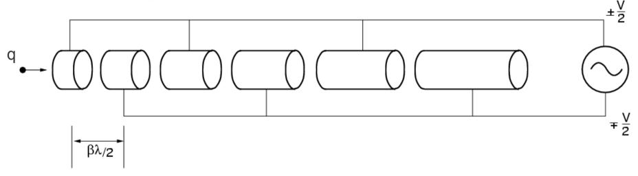
Alternate drift tubes are connected to a voltage generator providing a peak-to-peak voltage V across the gaps with angular frequency  $\omega = 2\pi f$ .
