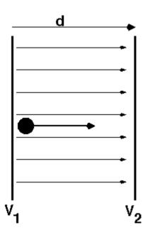
If a particle with charge q leaves the plate with potential  $V_1$ , when it reaches the plate with potential  $V_2$  has gained (or lost) energy
