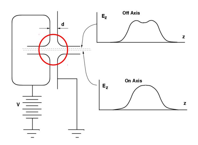
The kinetic energy is increased by the voltage drop across the gap. (Is this relativistically correct?)
