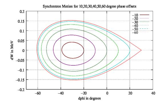
The limiting orbit defines the **separatrix**, outside of which the orbit is unstable and diverges in phase space away from the stable fixed point. The separatrix defines the maximum energy deviation any particle in the bunch may have and still stay captured within the bunch.
