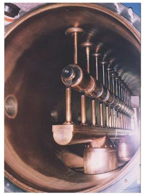
Drift tubes alternate between an excited coaxial line and the grounded outer wall.
