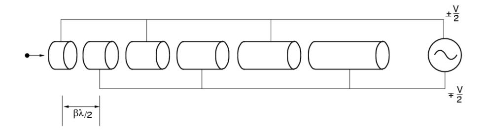
For the ion to remain synchronous as it accelerates, the distance between the gaps must be  $\frac{1}{2}$  an RF cycle, or more generally,  $(n + \frac{1}{2})$  cycles, where n is an integer.
