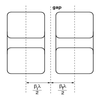
We will derive two first-order difference equations, one for the energy after the accelerating gap, and the other for the change in phase relative to the stable phase after the gap. From these difference equations, we can derive the equation of motion of particles in the bunch.
