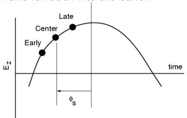
By convention, the phase of the center of the bunch is referred to the point in the RF cycle where the field is maximum. The phase which produces longitudinal focusing is negative.
