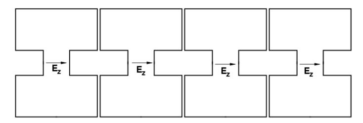
If we phase the RF fields in all the cavities to be identical in time, then the spacing between the gaps is  $\beta\lambda$ , or more generally,  $n\beta\lambda$ , where n is an integer: n = 1, 2, 3,....
