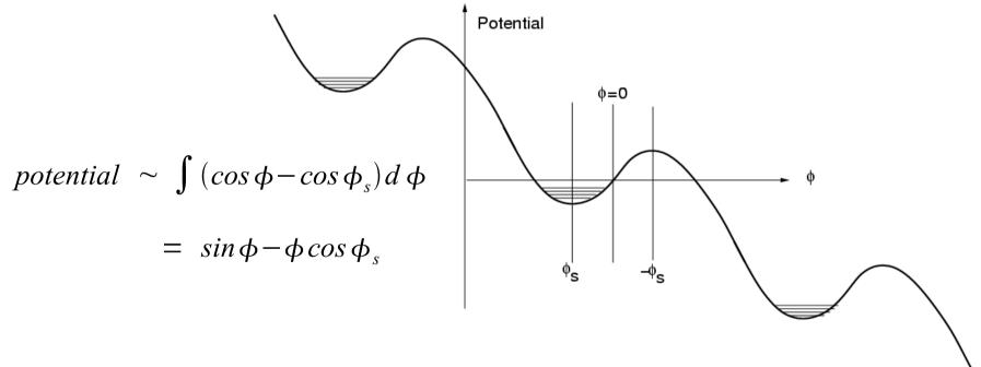
The ions reside in and oscillate around the bottoms of the potential wells. lons with energy greater than the well depth can spill out of the well (separatrix), and will have the wrong energy to settle down in an adjacent potential well.
