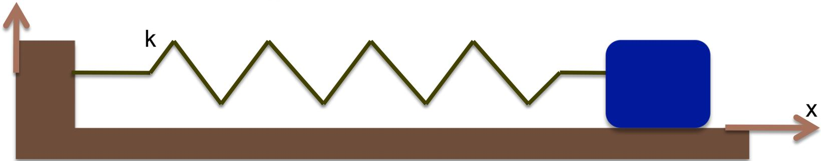
$$x(t) = x_0 \cos(\omega t + \chi) \quad \frac{dx(t)}{dt} = -x_0 \omega \sin(\omega t + \chi)$$
