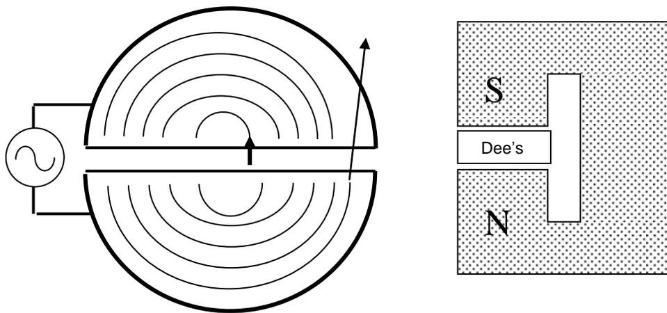
Figure 6 The cyclotron : top view (left) and side view (right)
