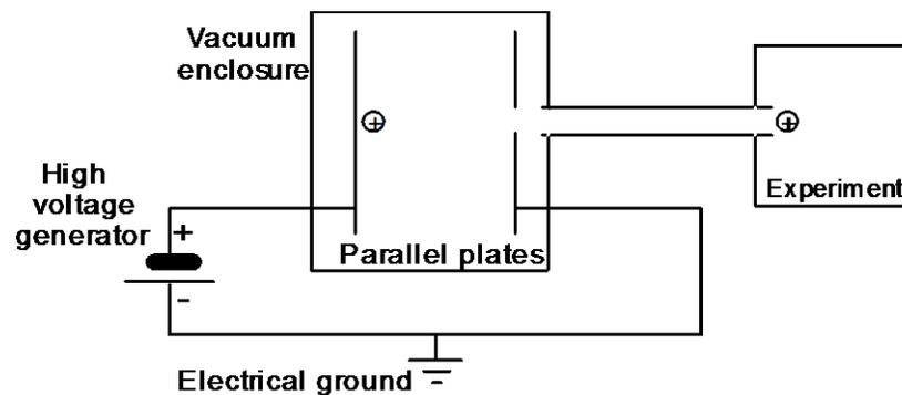
Figure 1. The DC accelerator
