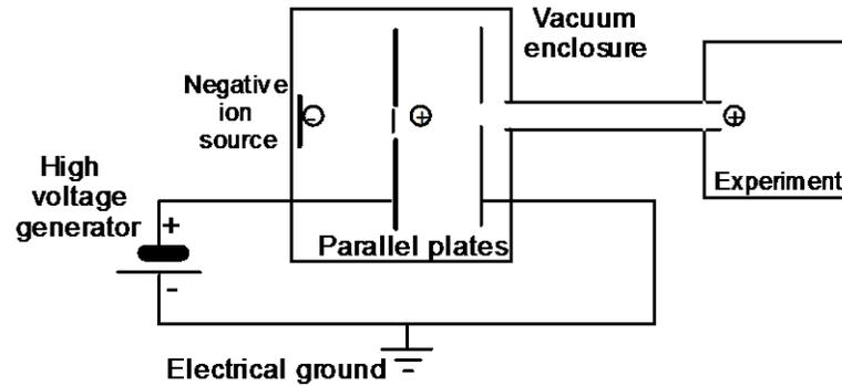
Figure 2. The Tandem accelerator
