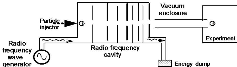
Figure 4. Accelerator with rf-cavities
