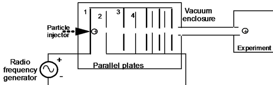
Figure 3. A multi-cavity radio frequency accelerator
