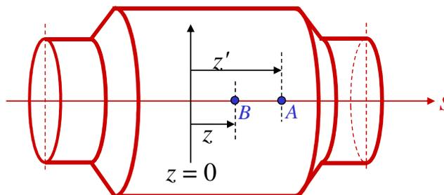
For example, the change in energy of particle *B* from the wake field of particle *A* in the figure, when the particles move through a given accelerator component, can be written:
