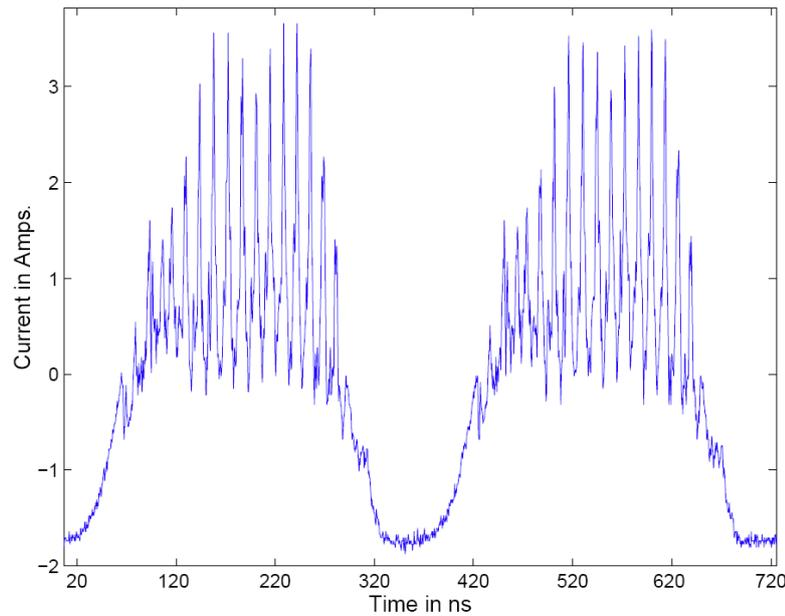
Observation of single-bunch longitudinal instability in the Los Alamos PSR, caused by an inductive impedance. From C. Beltran, A.A. Browman and R.J. Macek, "Calculations and observations of the longitudinal instability caused by the ferrite inductors at the Los Alamos Proton Storage Ring", Proceedings of the 2003 Particle Accelerator Conference, Portland, Oregon (2003).
