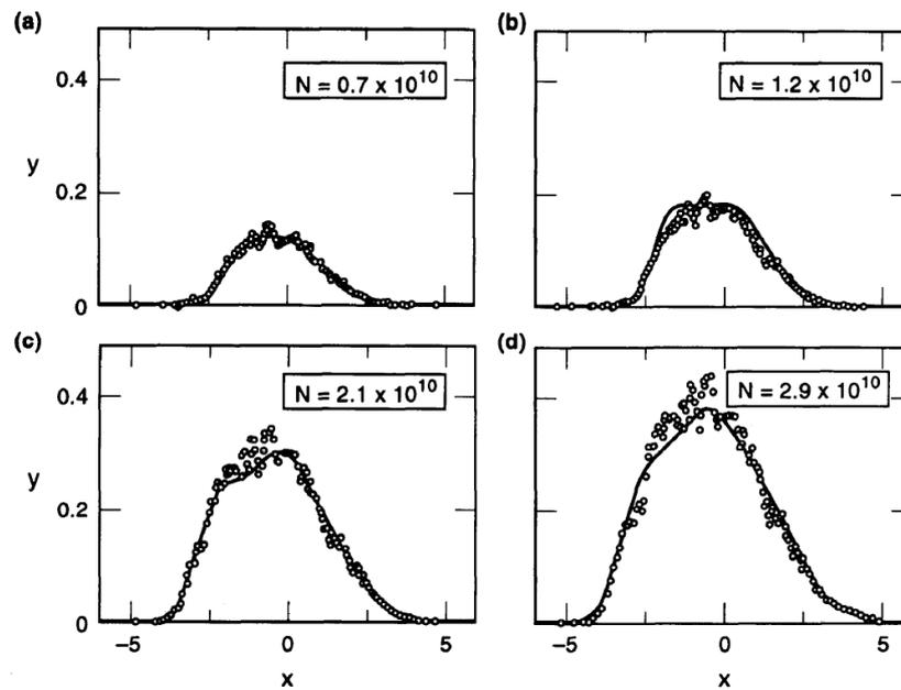
**Figure 6.4.** Potential-well distortion of bunch shape for various beam intensities for the SLC damping ring. The open circles are the measured results. The horizontal axis is  $x = -z / \sigma_{z0}$ , where  $\sigma_{z0}$  is the unperturbed rms bunch length. The vertical scale gives  $y = 4\pi e\rho(z) / V'_1(0)\sigma_{z0}$ . (Courtesy Karl Bane, 1992.)
