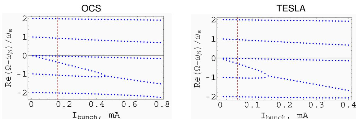
Calculations of TMCI thresholds in two designs for the ILC damping rings (by Sam Heifets). The bunch current at the nominal maximum bunch population of  $2 \times 10^{10}$  particles is shown by a red line in each case.
