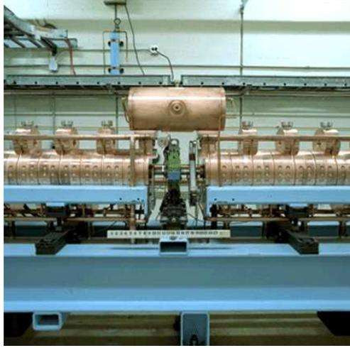
Figure 4: Fermilab 800 MHz side coupled cavities, used in the high energy end of the Linac. Accelerating gradient  $\sim 7.5$  MV/m. Courtesy Fermilab visual media services.
