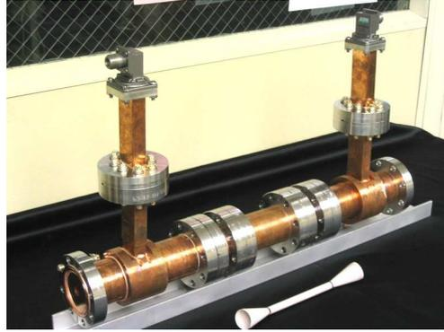
Figure 6: Dielectric-loaded waveguide (11 GHz). Courtesy Sergey Antipov and Chunguang Jing, <http://www.hep.anl.gov/awa/links/dla.htm>. The figure includes sections of waveguide and RF couplers that convert between the  $TE_{10}$  mode in the rectangular waveguide to the  $TM_{01}$  mode in the dielectric loaded accelerating structure. The accelerating gradient is estimated to be greater than 60 MV/m.
