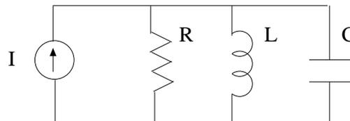
Accelerating cavities are resonators, and are sometimes modeled by resonant circuits, such as the one shown in the figure above.
