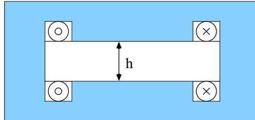
The transverse cross-section of a simple bending magnet is shown in the figure above. There are  $N$  turns of conductor carrying current  $I$  wound about each pole of the iron magnet. The poles are separated by a distance  $h$ . Assuming the permeability of the iron to be infinite, show that the field in the gap of the magnet is given by
