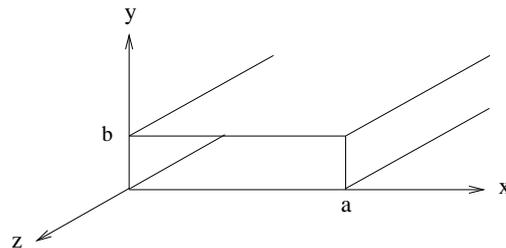
The longitudinal electric field  $E_z$  is zero for TE modes in an evacuated waveguide. The longitudinal magnetic field has the form  $B_z = B(x, y) \exp i(kz - \omega t)$ . The wave equation can be solved using the separation of variables method, i.e. assuming a solution of the form  $B_z = X(x)Y(y) \exp i(kz - \omega t)$ .
