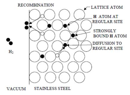
Fig. 3. Schematic diagram of a recombination process at the SS surface.
