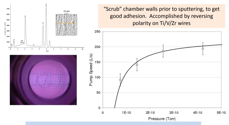
NEG coating turns a gas source into pump ~0.02 L/s·cm<sup>2</sup> : Modest pump speed can be improved Literature reports ~1 L/s·cm<sup>2</sup>
