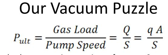
Q= gas load, q= outgassing rate, A = surface area, S = pump speed
