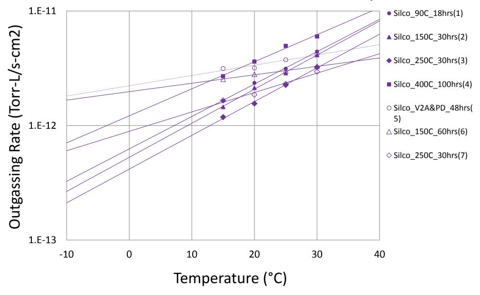
Amorphous silicon coating: hydrophobic and likely a good H2 barrier
