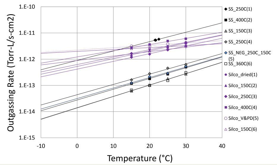
Now, coat bare chamber with Silco following 400C bakeout Then only low temp bakeout required
