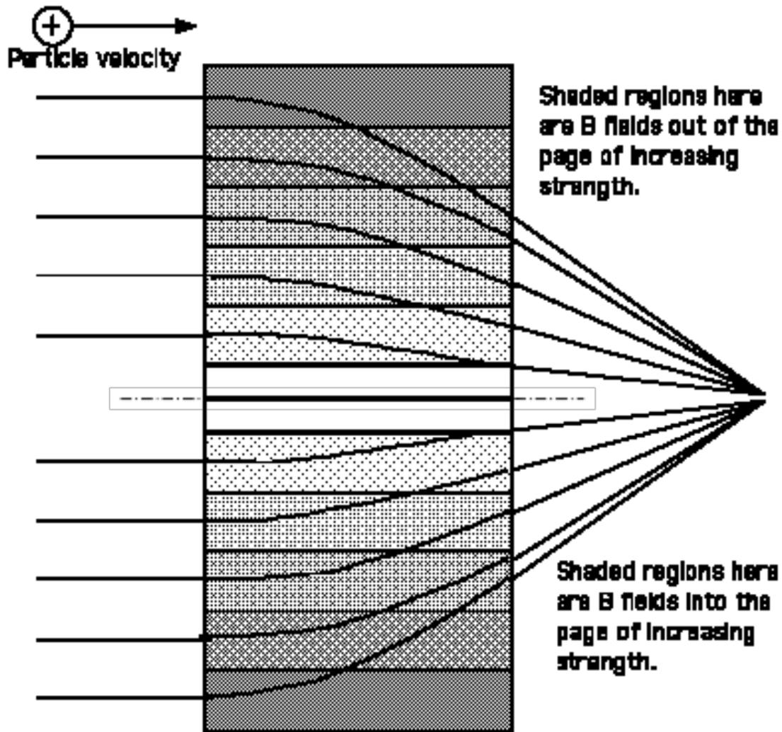
**Magnetic focusing 'lens'.** The diagram shows the type of magnetic focusing fields we would like to create. Particles found further from the design orbit travel through a stronger magnetic field and therefore feel a stronger restorative force.
