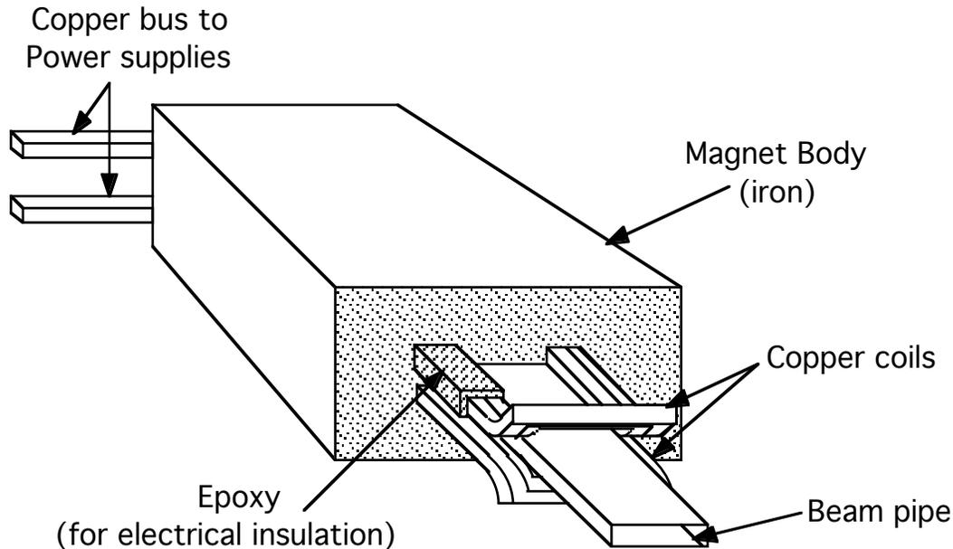
Specially treated cooling water (called LCW, which stands for Low Conductivity Water) flows through the passage inside the bus to carry away the large amounts of heat generated by the high current flow. Also notice that an iron magnet body, which concentrates and shapes the magnetic field, surrounds the coils. Finally, notice how the beam pipe inside the magnet is placed very close to the coils themselves. This maximizes the magnetic field “felt” by the beam passing through.
