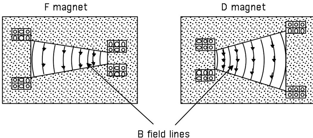
those of the bend field and quadrupole field shown in the previous sections, which we will leave as an exercise for the reader. Permanent (non-powered) gradient magnets are also used in the Recycler and the MI-8 line.
