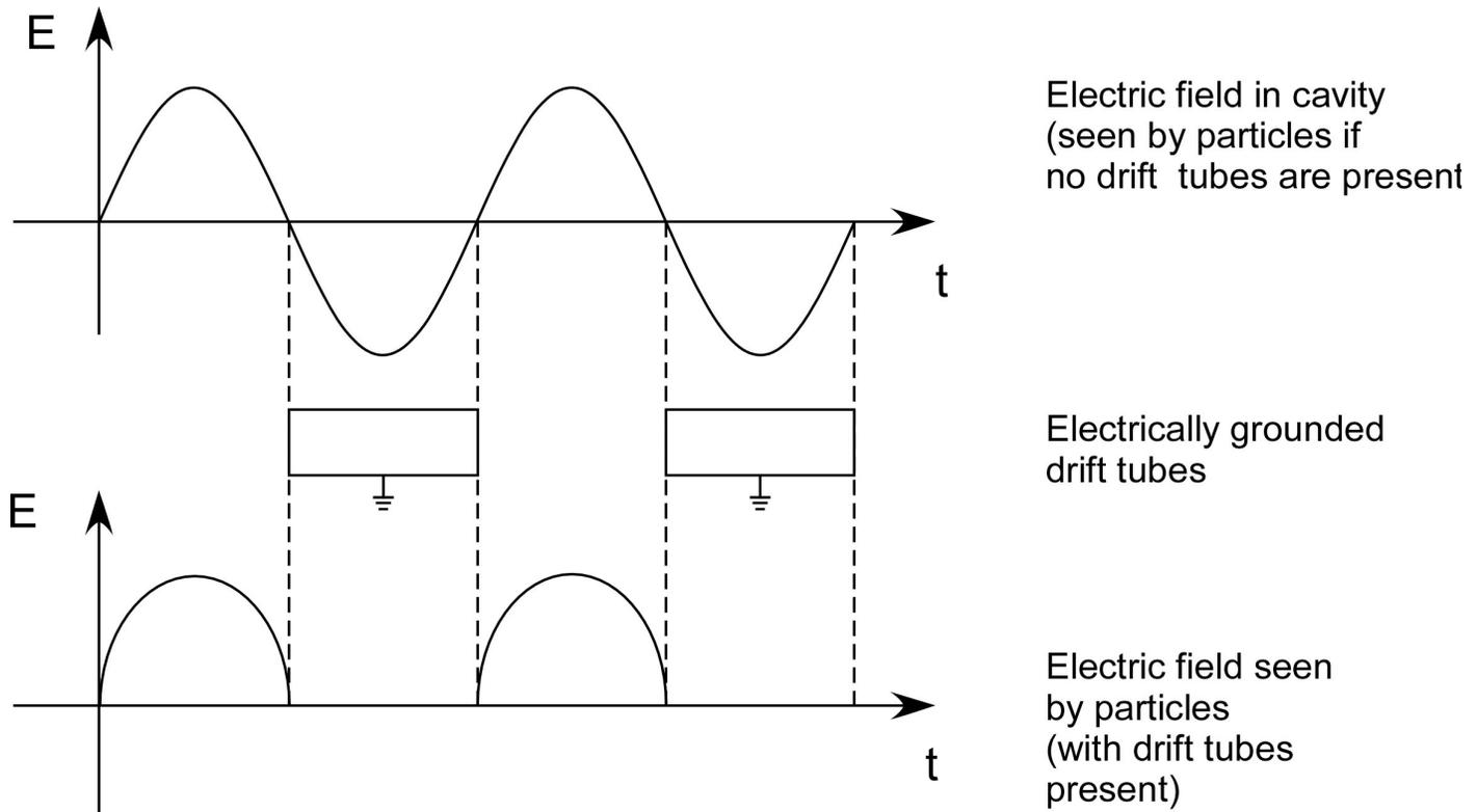
**Electric fields with drift tubes.** The graph on top represents the magnitude of the accelerating electric field in a RF cavity versus time. The bottom graph shows only that portion of the electric field seen by particles in a cavity equipped with drift tubes.
