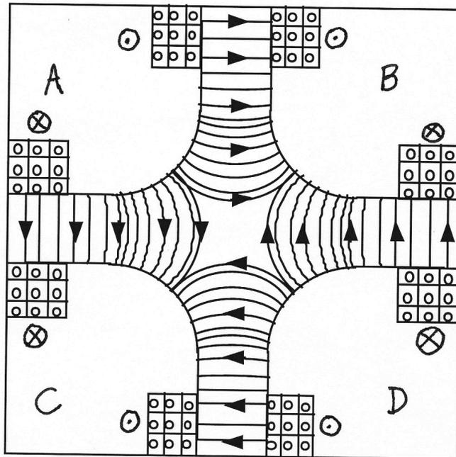
**Quadrupole magnet.** The four (usually iron) magnetic pole faces are labeled A, B, C, and D. The arrowed lines indicate the magnetic field. The direction of current flow, which is into or out of the page, is labeled near the square bus work. Notice the holes in the bus for cooling LCW. A given quadrupole can only focus the beam in one plane—while defocusing the beam in the other.
