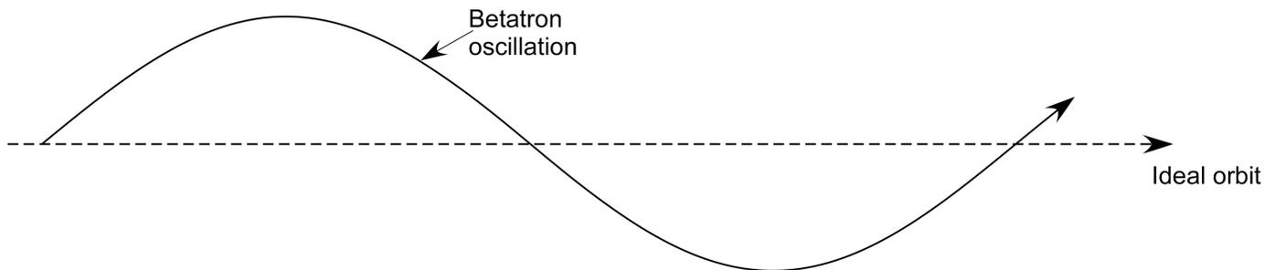
**Betatron Oscillations.** Quadrupole focusing forces particles into transverse oscillations about the ideal orbit. The particle's path is shown as the solid line above.
