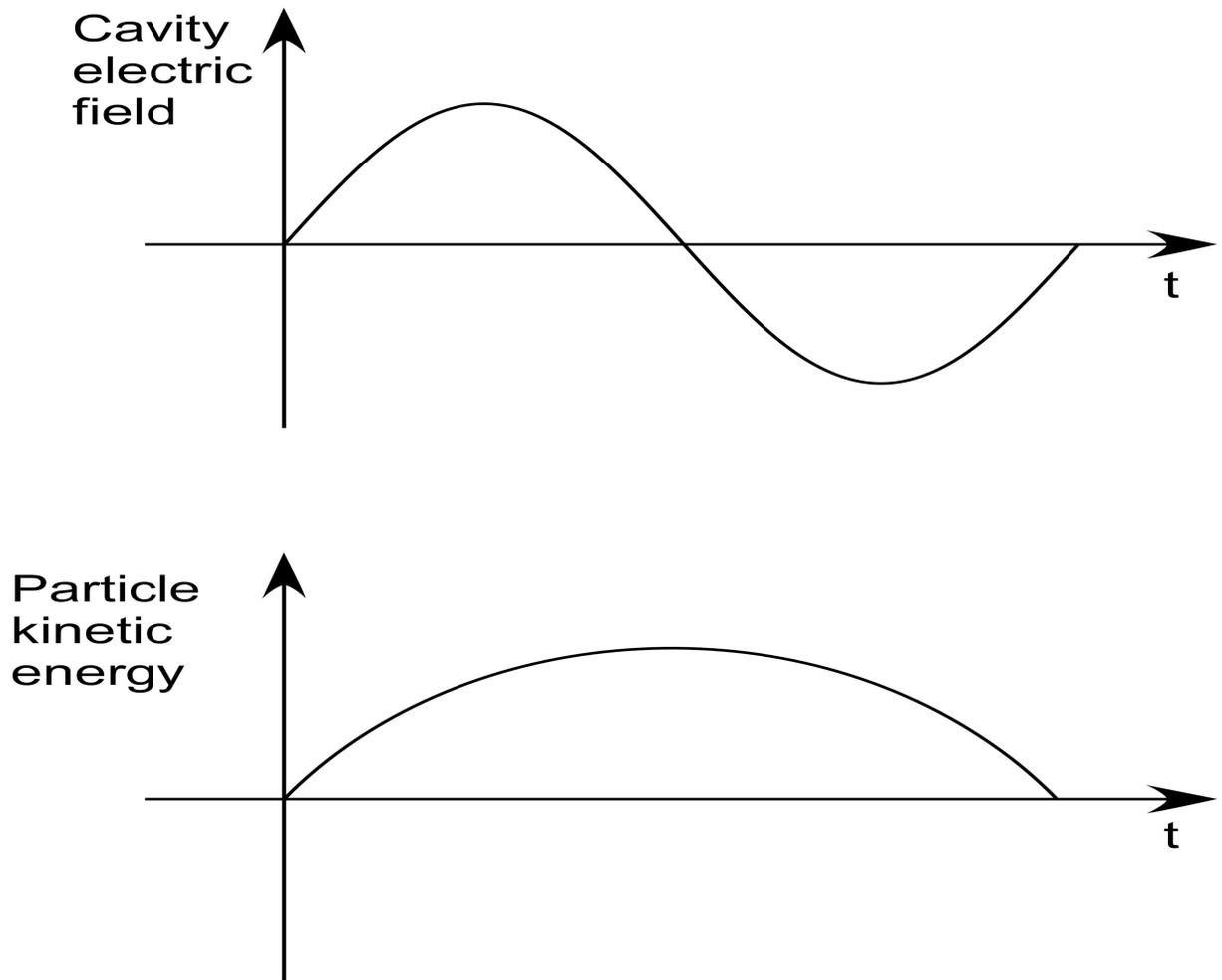
**No kinetic energy gained.** The sinusoidal curve on top represents the magnitude of the accelerating electric field in a RF cavity versus time. The other graph shows the change in particle kinetic energy versus time if the particle is present in the RF cavity for both accelerating and decelerating fields (net kinetic energy gain equals zero).
