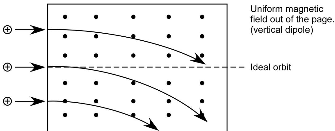
**Attempt at vertical focusing.** The three arrows at the left represent three different particles within a bunch. The top most is the imperfect particle in the example in that has drifted upwards. The center arrow is a perfect particle initially traveling on the design orbit. The bottom arrow is another imperfect particle that has drifted downwards. When all three particles enter the field created by the vertical dipole, they are deflected downwards.
