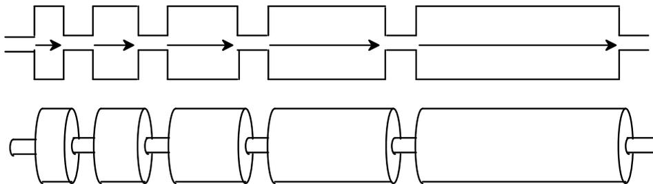
Constant Frequency with an Increasing Acceleration Gap Length
