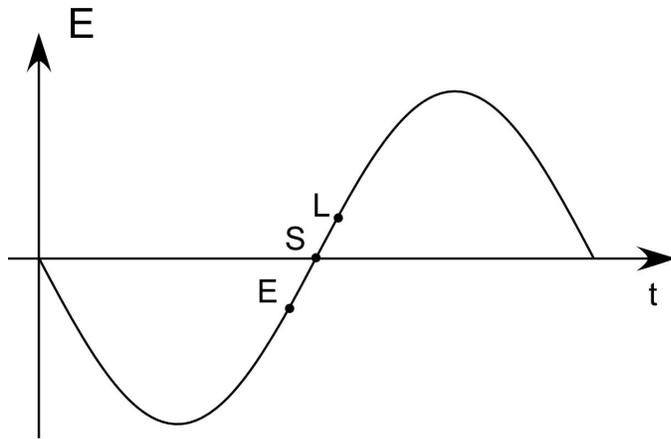
**Injection.** The sinusoidal curve represents the magnitude of the accelerating electric field in a RF cavity versus time. The labeled points represent various beam phases.
