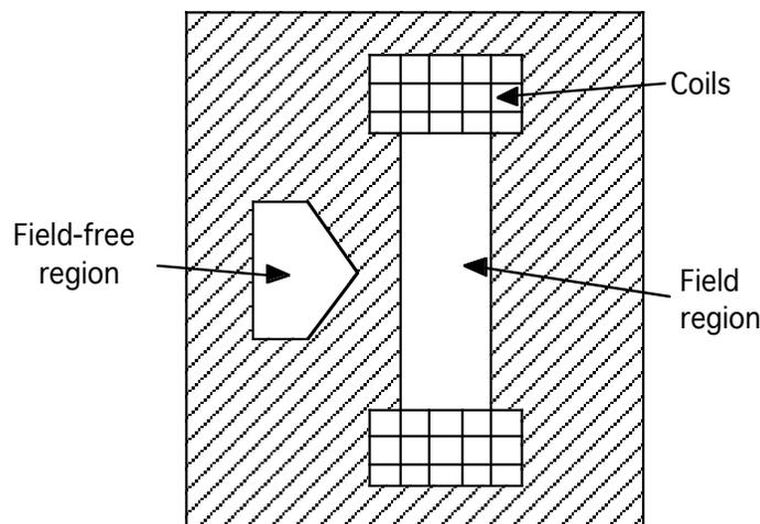
**Lambertson.** This magnet has two apertures: a magnetic field region (like a dipole), and a field free region. It's used as an injection or extraction device in circular accelerators or as a way to separate beams in a beam line.
