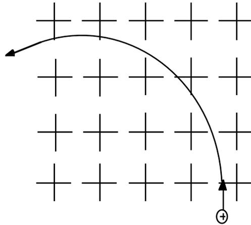
**Bend Field.** The crosses indicate a magnetic field pointing into the page. Given the positively charged particle initially traveling upwards, the right hand rule dictates a force to the left, deflecting the particle from its original path.
