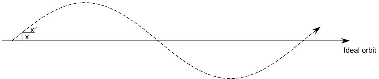
**Position and angle.** A particle's trajectory at any point can be described in terms of its distance from the design orbit,  $x$ , and the angle between its trajectory and the ideal orbit,  $x'$ .
