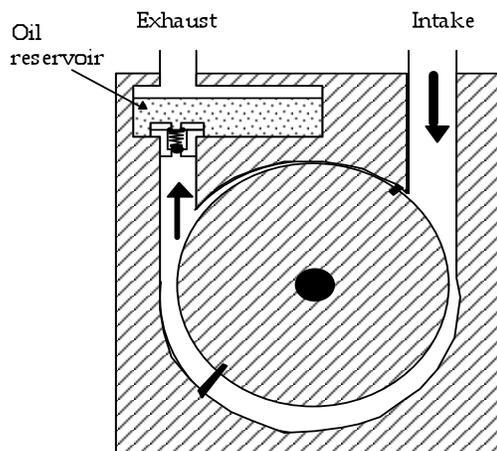
**Roughing Pump.** This pump has rotating vanes that trap air molecules and mechanically force them out the one-way exhaust valve.
