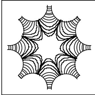
**Octupole magnet.** The octupole has eight magnetic pole faces. The lines indicate magnetic fields. It controls the coupling between betatron tune and betatron oscillation amplitude in an accelerator.
