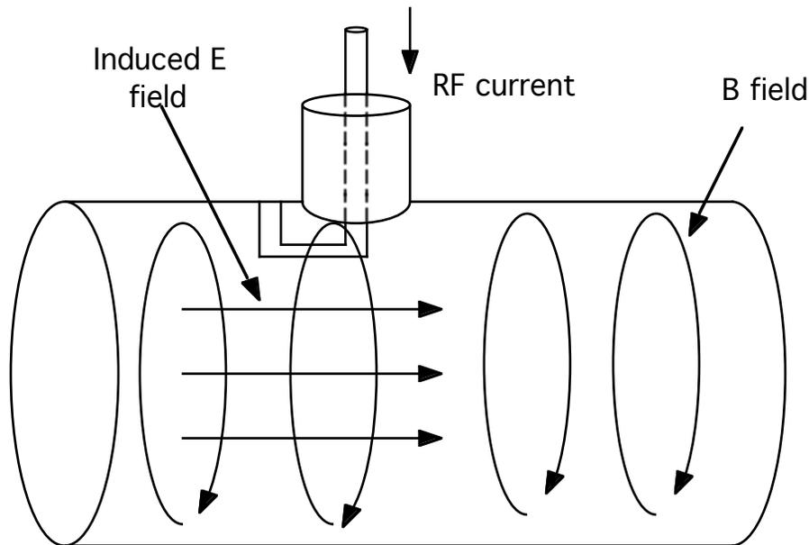
Notice how the magnetic field is in a direction that will not affect beam traveling along the lines of electric field.
