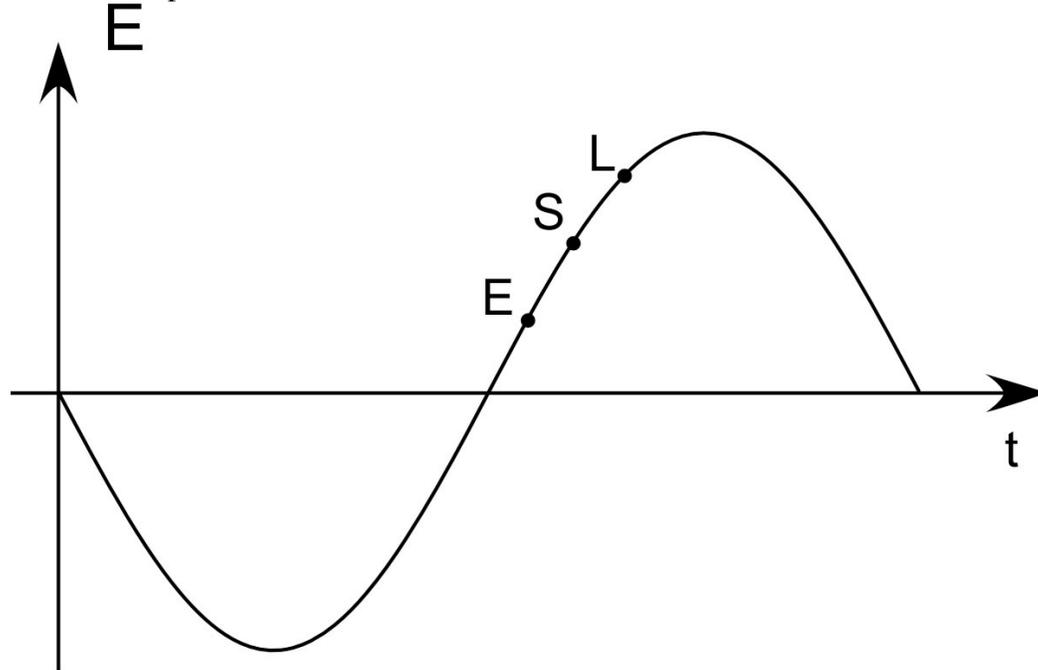
**Acceleration.** The sinusoidal curve represents the magnitude of the accelerating electric field in a RF cavity versus time. The labeled points represent various beam phases.
