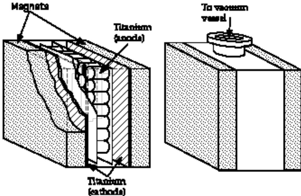
**Ion Pumps.** This pump works by ionizing air molecules then capturing the free electrons on the anode and the ionized molecules on the titanium plates. An electrical current proportional to the number of ions created can be measured, indicating the quality of the vacuum. Molecules trapped in this way no longer contribute to the vacuum pressure inside the beampipe.
