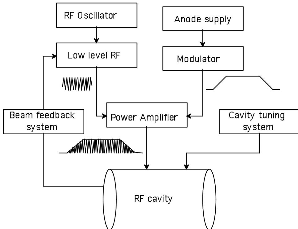
The oscillator is the low power source of the correct frequency signal that drives the cavity. The LLRF system is typically a computer that can adjust the phase of the oscillator's signal as needed.
