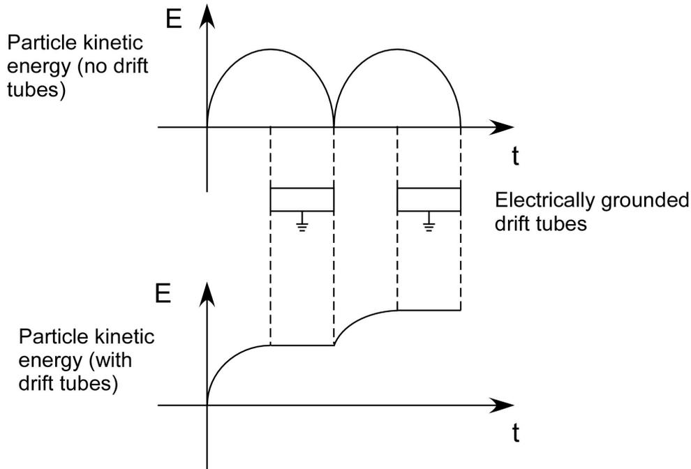
**Kinetic energy gained.** The top graph shows the change in particle kinetic energy versus time if the particle is present in the RF cavity for both accelerating and decelerating fields (net kinetic energy gain equals zero). The bottom graph shows a non-zero net increase in kinetic energy due to the shielding effect of the drift tubes.
