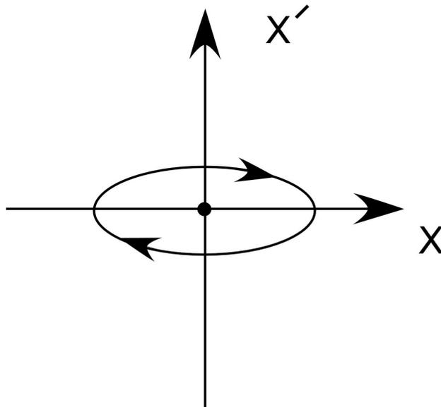
**Phase space diagram.** Here's another way to view betatron oscillations. As the particle travels along the ellipse its distance from the ideal orbit,  $x$ , increases and decreases, as does the angle of the particle's trajectory relative to the ideal orbit,  $x'$ . The ellipse shown is the Separatrix—the boundary between stable particles that stay in the machine and unstable particles that are lost.
