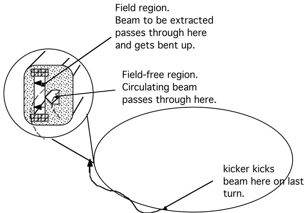
**Beam Extraction.** Beam initially traveling on the closed orbit is given a kick (by a kicker) and is sent into unstable oscillations. Appropriately placing a Lambertson downstream of the kicker allows the field region to be selected, bending the beam away from the plane of the accelerator. For injection, the same events happen in reverse.
