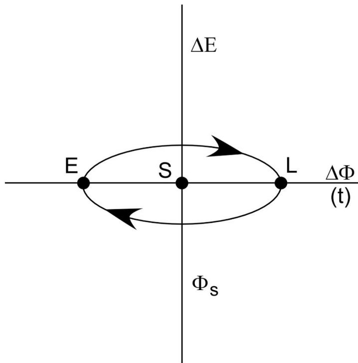
**Phase Space Diagram.** Here is a good way to view synchrotron oscillations—phase errors become energy errors become phase errors and so on. The labeled points represent various initial beam phases.
