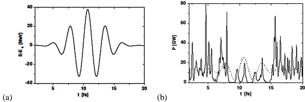
Figure 12 (a) Energy modulation of the electron beam at the exit of the modulator undulator. The laser parameters are wavelength = 800 nm,  $W_{\text{peak}} = 800$  GW, and FWHM pulse duration of 5 fs. (b) Typical single-shot temporal structure of the central part of the radiation pulse. Undulator length is 120 m. Dotted line shows energy modulation of the electron bunch shown in panel (a).
