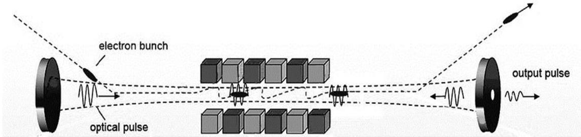
Figure 19. Simplified schematic of a cavity FEL
