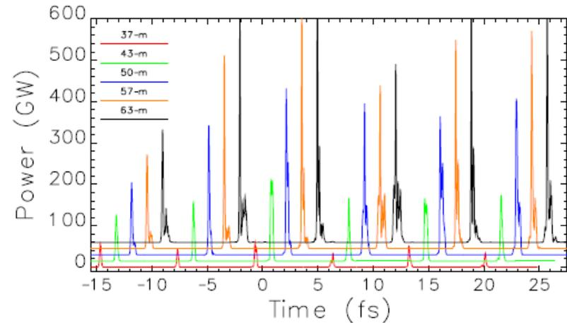
Figure 5:  $P(t)$  snapshots at 5 different  $z$ -locations for a 2.2  $\mu\text{m}$ -energy-modulated ESASE pulse with  $\langle\beta\rangle = 12\text{ m}$ , plotted with staggered offsets of 1.5 fs in time and 15 GW in power. For legibility, the  $z = 37\text{ m}$  data has been multiplied by a factor of 2.0.
