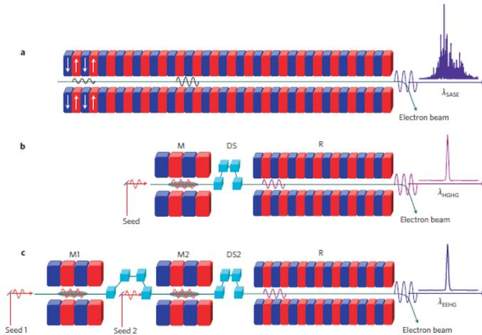
**Figure 1 | Seeded FEL versus SASE FEL.** a, SASE FEL, with poor temporal coherence. b, HGHG FEL, showing full temporal coherence with limited harmonic number ( $N \approx 10$ ) for a single stage. c, EEHG FEL, showing full temporal coherence with a potentially very high harmonic number in a single stage. M, modulator; DS, dispersive section; R, radiator.
