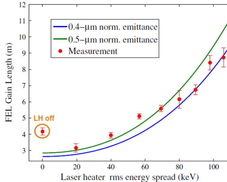
FIG. 16. (Color) FEL gain length at 1.5 Å vs LH-induced energy spread.
