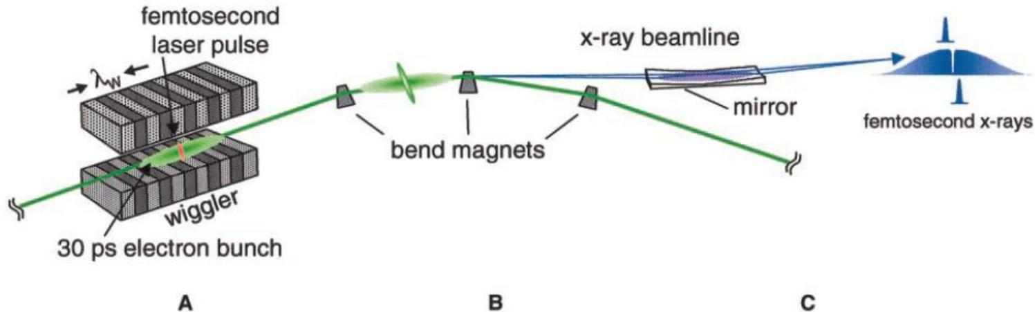
A Overlapping short laser beam with bunch center, meeting the resonance condition,
