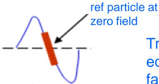
Transit-time cooling: tune bypass so that particle with the equilibrium momentum arrives at zero-field, and faster/slower arrive around it.
