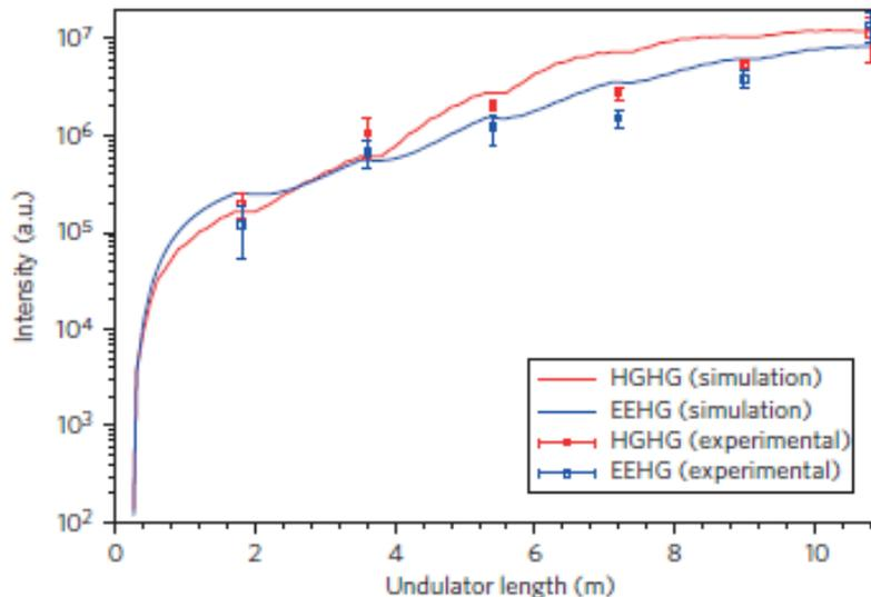
**Figure 5 | Gain curves of the EEHG and HGFG FEL at SDUV-FEL.** Intensity is measured with a calibrated CCD at the end of the radiator (red open squares, HGFG; blue open squares, EEHG). Error bars correspond to the peak-to-peak intensity statistics of 100 measurements. Simulation results are shown as a red line (HGFG) and a blue line (EEHG).
