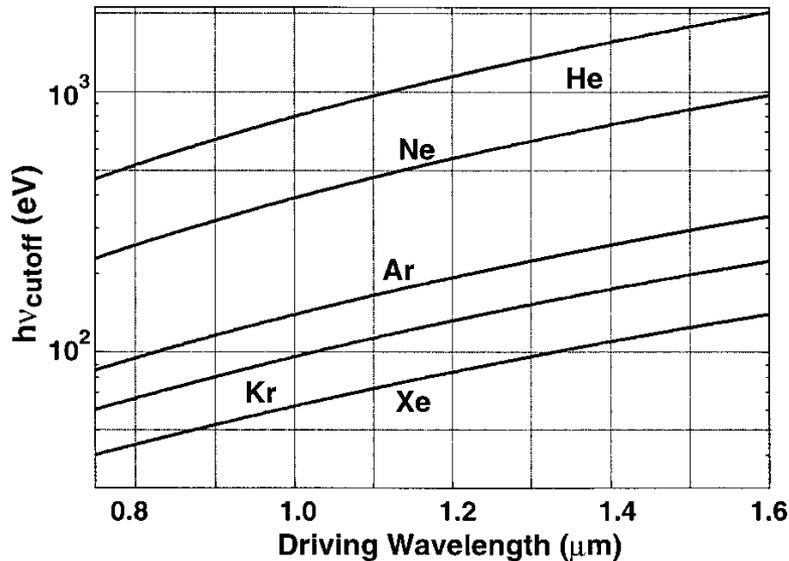
FIG. 1. Calculated relationship between single-atom HHG cutoff photon energy and the driving wavelength.
