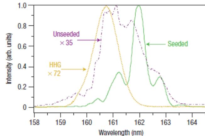
**Figure 5** Spectra of the FEL fundamental emission using the two undulator sections: unseeded (single shot, dash-dot) and seeded (single shot, line) obtained with a 4.3 nJ seed (single shot, dots). The FEL gain is smaller compared with the measurements in Figs 2 and 3, because of the lower electron-beam brightness ( $B_p < 200$  A ( $\pi$  mm mrad)<sup>-2</sup>), transverse misalignment ( $F_f < 1$ ) and spectral detuning ( $\lambda_{\text{seed}} - \lambda_{\text{SE}} \leq 0$ ).
