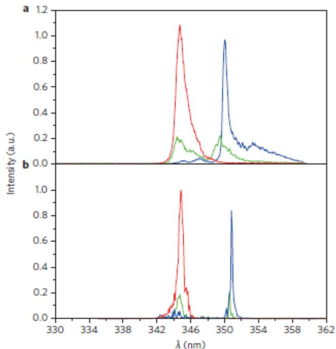
**Figure 3 | Spectra for FEL radiation.** **a**, Experimental results (red line, HGFG; blue line, EEHG; green line, intermediate state between HGFG and EEHG). **b**, Simulation results (red line, HGFG; blue line, EEHG; green line, intermediate state between HGFG and EEHG).
