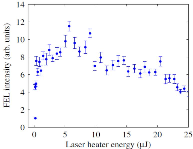
FIG. 15. (Color) FEL intensity at 1.5 Å measured on a downstream YAG screen vs LH energy when 12 undulator sections are inserted.
