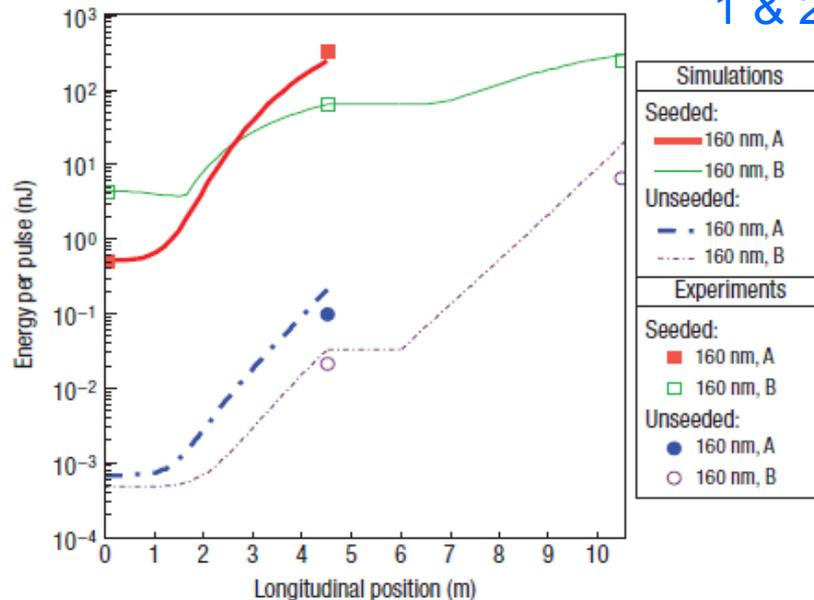
**Figure 4** Evolution of the 160 nm FEL pulse energy along the two undulator sections: comparison of experimental data and simulations using PTD code. The two sections, each of 4.5 m, are separated by a 1.5-m-long drift space. Two cases of amplification are considered, at low and high HHG seed energy, respectively; they also differ slightly in the electron-beam brightness and the spatial/spectral overlaps between the seed and electron beam.
