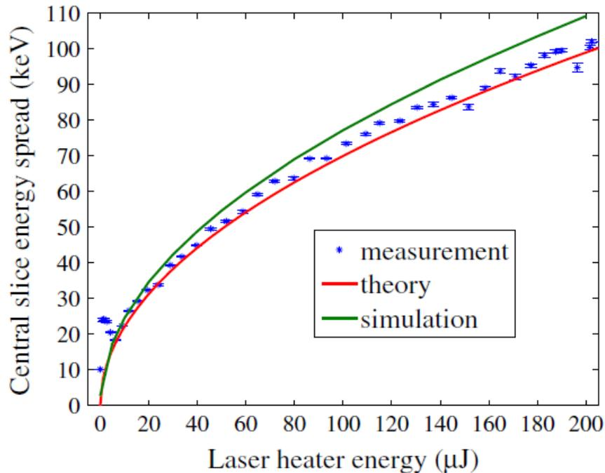
FIG. 8. (Color) Central slice rms energy spread vs LH energy.
