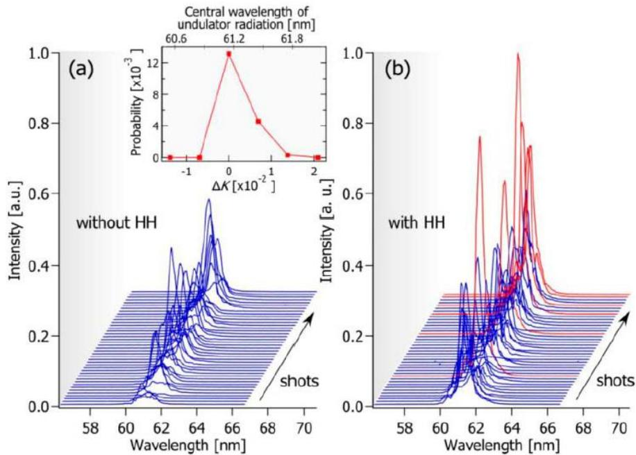
Fig. 2. Spectra of FEL radiation in fifty successive shots without (a) and with (b) HH injection. The red lines in (b) show profiles that have higher intensities above the threshold level. The inset shows an appearance probability of the high-intensity condition as a function of the deviation of K-value,  $\Delta K = K - 1.37944$  (lower axis), and the central wavelength of the undulator radiation (upper axis).
