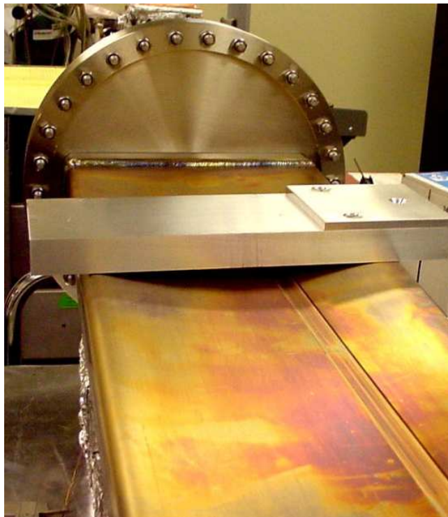
Distorted copper chamber during a bakeout
