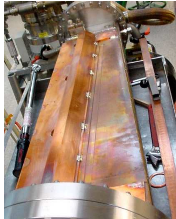
The chamber was saved by pressurizing and stiffening
