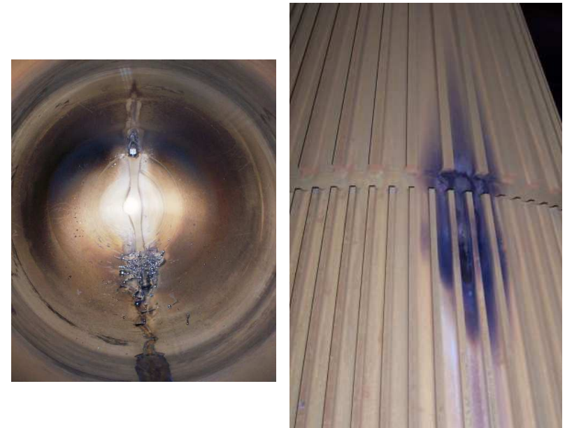
Electron beam melted through aluminum body
