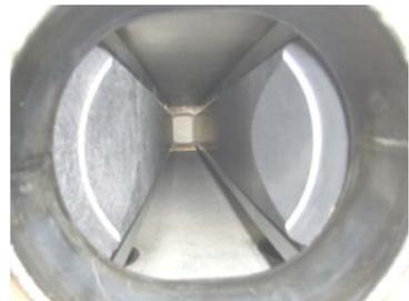
Protective masks. (Picture of an LHC Collimator)
