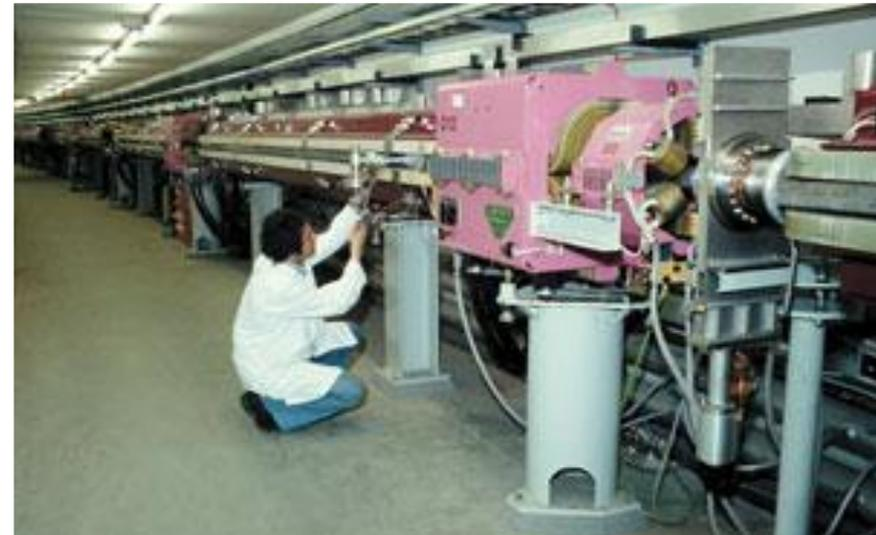
PETRA Tunnel 1980 with bending magnets, quadrupoles and sextupole
