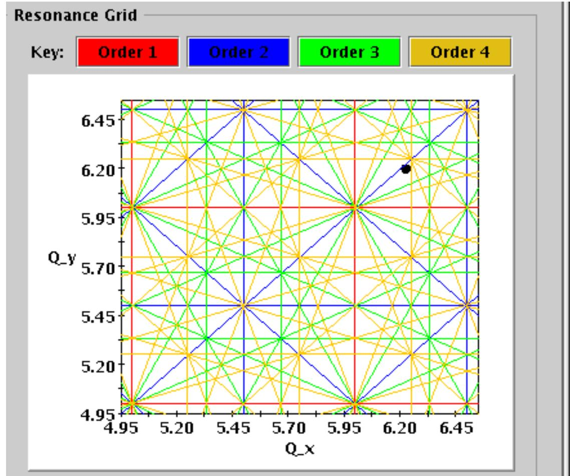
We could populate the diagram endlessly, but since resonances become weaker with increasing order gets, it's not necessary.
