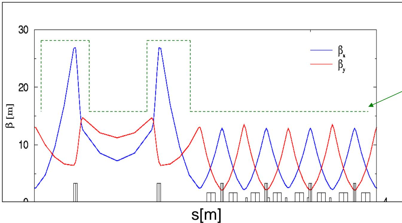
Beam pipe aperture scales with beta function.
