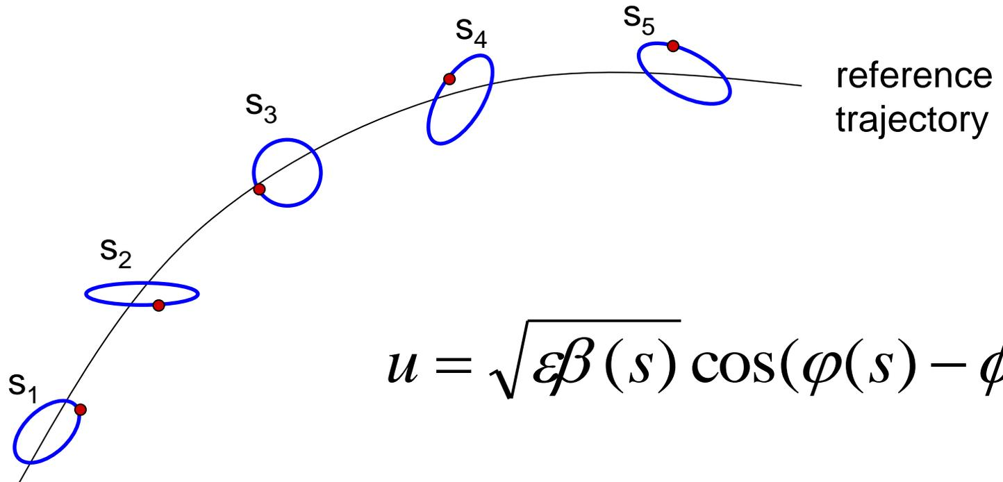
The motion of the particle in real space,  $u$ , is “quasi-harmonic”.
