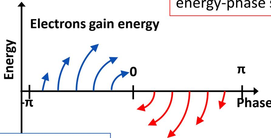
The electrons with phase sums between  $-\pi/2$  and  $0$  continuously gain energy to the electrons, and move up and to the right in energy-phase space.
