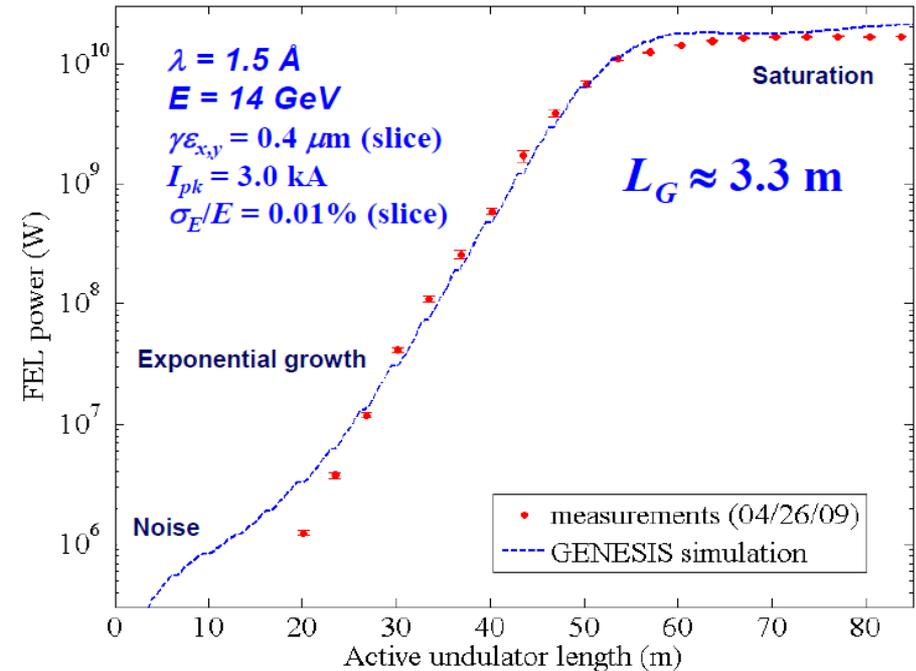
Linac Coherent Light Source first lasing
