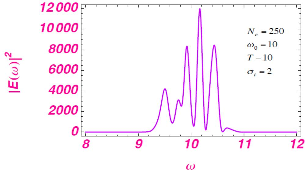
The above example gives an optical pulse that has about 6 coherence lengths
