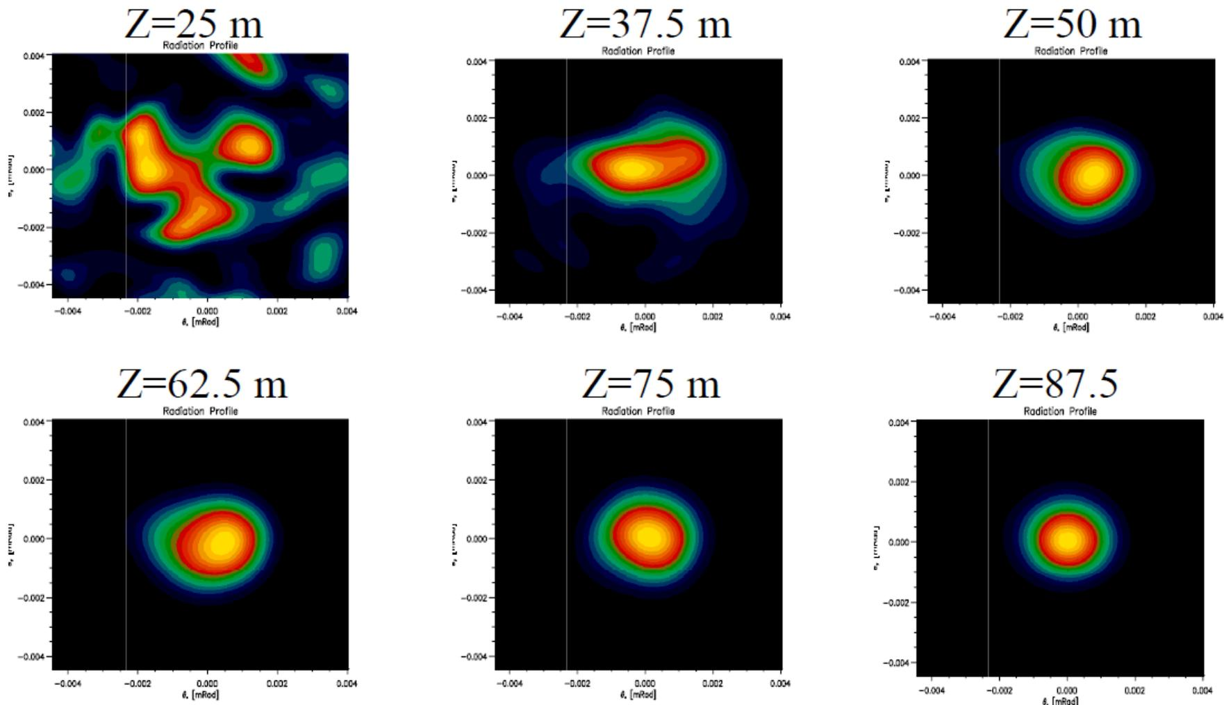
The x-ray beam's spatial profile becomes transversely coherent at  $z > 75$  m
