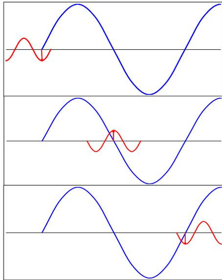
The electrons with phase sums between  $0$  and  $\pi/2$  continuously lose energy to the radiation and move down and to the left in energy-phase space.
