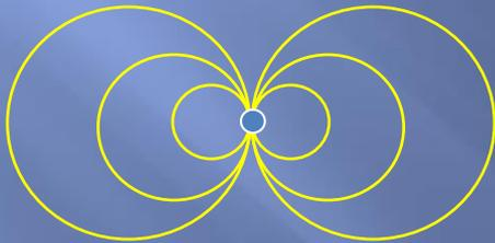
The Lorentz transformed undulator field acts like a traveling electromagnetic wave causing the electron to oscillate in the  $x'$  direction.
