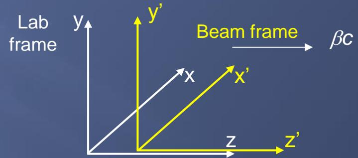
In this diagram, the “Beam frame” is moving at speed  $v_z = \beta c$  with respect to the Lab frame.
