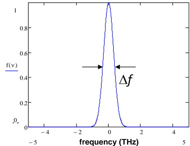
Minimum time-bandwidth product for rms widths in time and angular frequency
