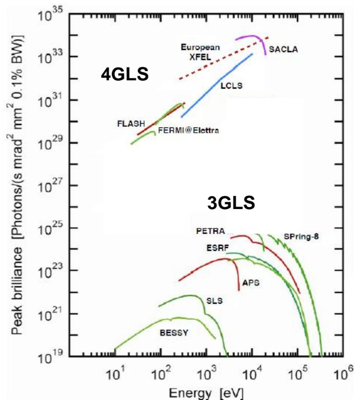
FEL peak brightness is enhanced over SR by the smaller transverse emittance, shorter pulses, and the bunched beam radiation enhancement factor which is equal to the number of electrons in a coherence length.
