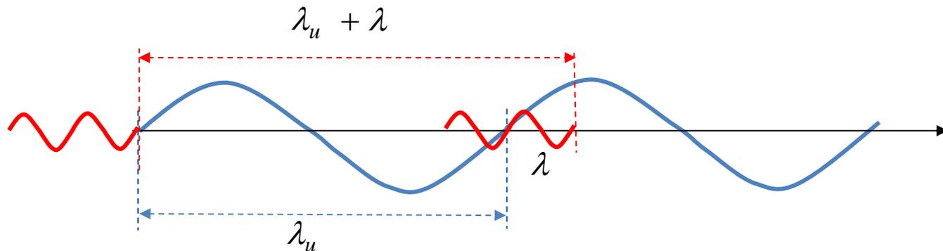
In the time the electron (blue) traverses one undulator period, the light wave (red) traverses one undulator period plus one wavelength.
