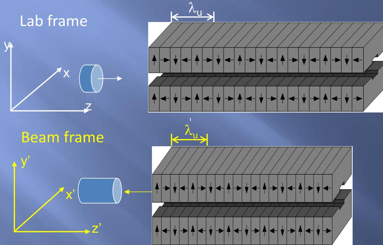
In the beam frame, the undulator period is contracted by  $\gamma^*$
