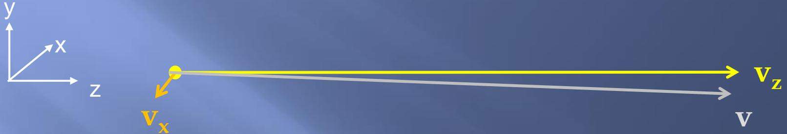
The transverse velocity is derived from the total velocity at the expense of the axial velocity.
