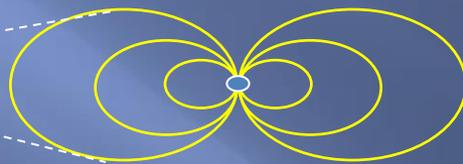
Radiation in the beam frame is isotropic and follows the dipole radiation pattern.
