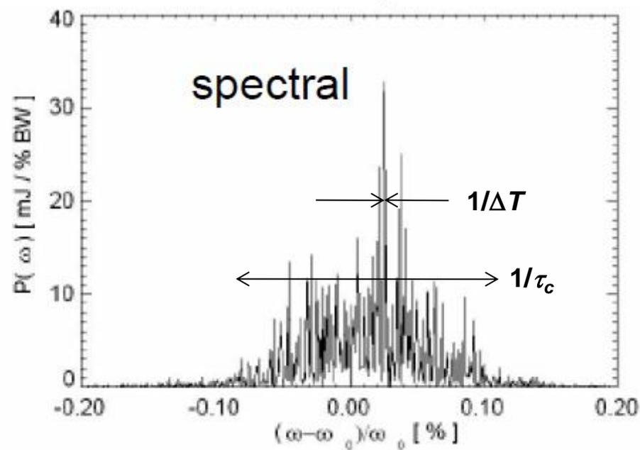
The LCLS output consists of several spikes in both temporal and spectral profiles. The full width of the spectral profile is the Fourier transform of each individual temporal “spike,” also known as a coherence length. The width of each spectral “spikes” is the Fourier transform of the entire x-ray (electron) bunch length.
