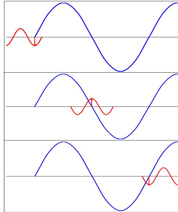
Constant phase sum enables energy exchange to accumulate with time.
