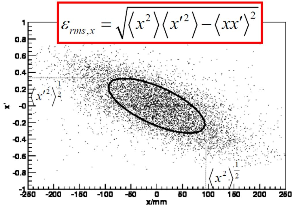
The electron beam emittance also contributes to the spreading of the photon beam in phase space. At the beam waist, the  $x$ - $x'$  correlation vanishes and the beam's rms emittance is simply
