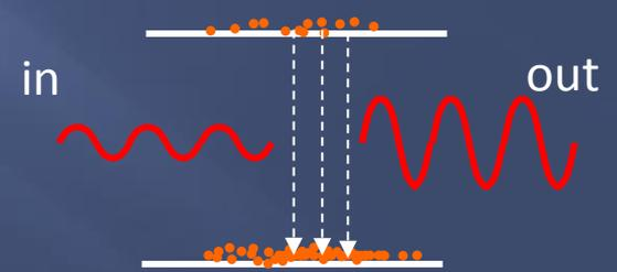
In stimulated emission, the incoming EM wave stimulates transitions from level 2 to level 1. If there are more atoms in 2 than in 1 (population inversion), the EM wave intensity is amplified exponentially along the gain path. The output beam has the same color and phase (temporal coherence) and propagates with very small radius and angular divergence (spatial coherence).
