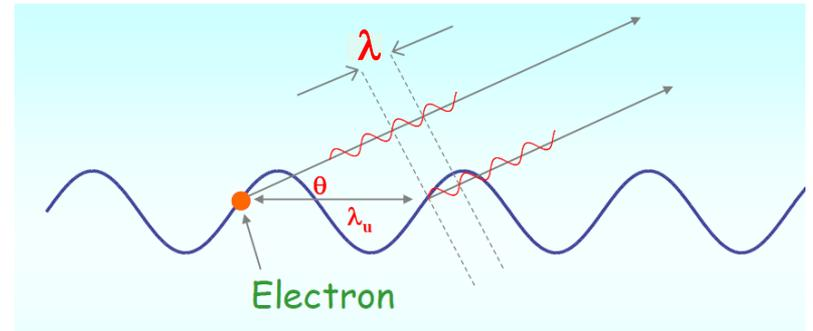
Accelerated charged particles radiate EM waves with power  $P \propto \dot{v}^2$
