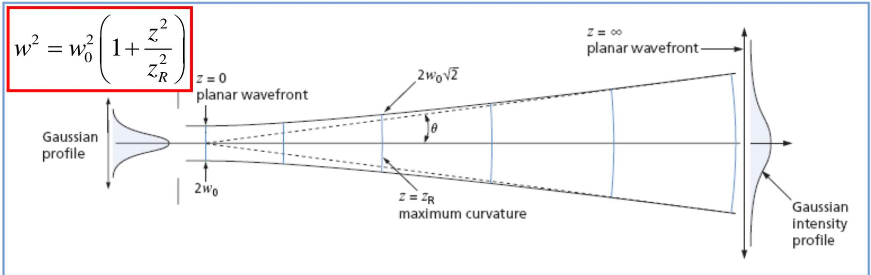
The product of rms radius and angular divergence is equal to the photon beam emittance. The smaller the beam radius at the waist, the larger the divergence angle. Rayleigh length is the length over which the beam area doubles.
