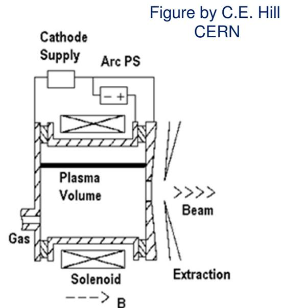
Fig. 4 Axial extraction Magnetron
