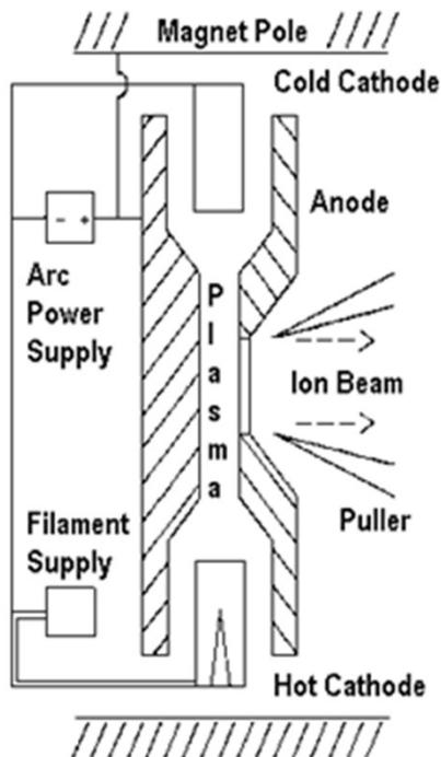
Fig. 3 Schematic hot cathode Penning
