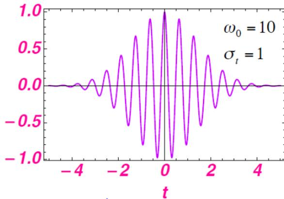
Intensity of a Gaussian wave packet:
