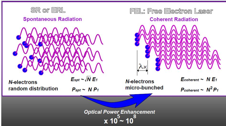
If the electrons are *independently radiating*, then the phase of their electric field are random with respect to one another, like in *SLS*, and we have:  $|\vec{E}| \propto \sqrt{N_e}$ ,  $P_{\gamma,tot} \propto N_e$
