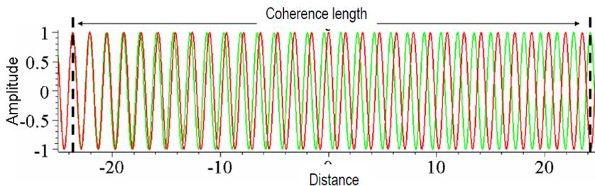
**Transverse coherence** length: the distance over which the e.m. field can be reconstructed from the knowledge of the field at another point, in the same plane (i.e., the field phase information is preserved). A coherent beam generates interference patterns.
