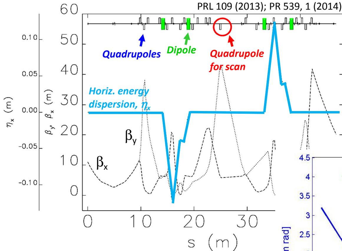
Many quadrupoles ensure  $\pi$ -phase advance between dipoles and proper values of  $\beta_x, \alpha_x$  to cancel the final emittance growth.
