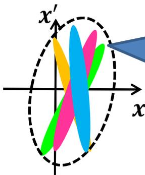
Different bunch slices feel different CSR kicks, thus move on different  $\beta$ -trajectories. If the slice ellipses are not concentric, the **projected** emittance is **larger**, although individual slices may have the **same slice emittance**.
