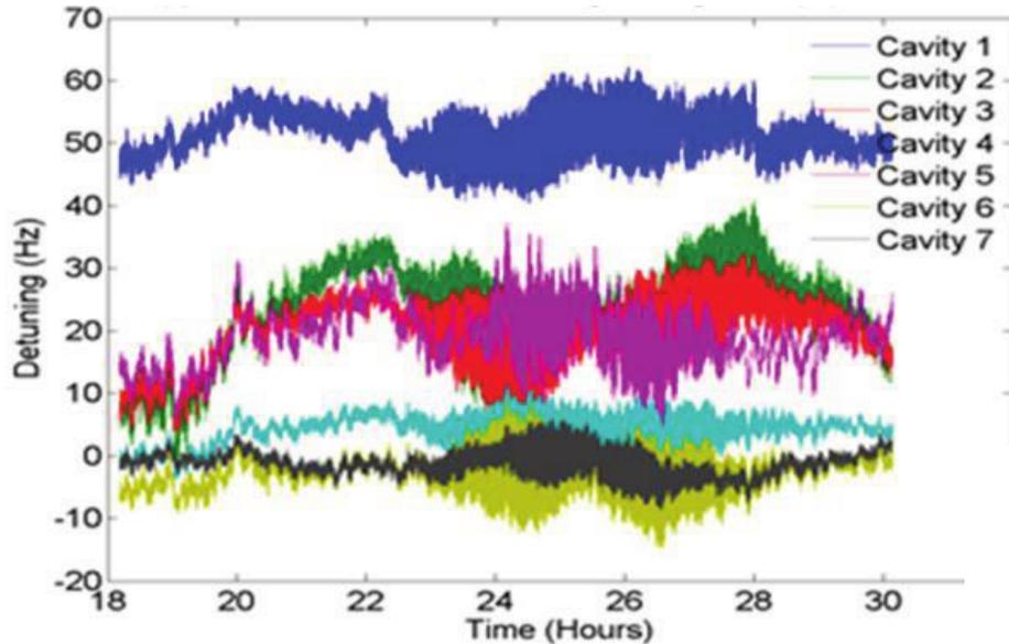
Cavity resonance frequency detuning of several tens of Hz
