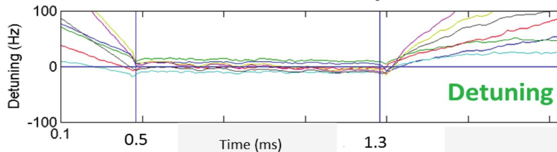
Control limits the detuning to  $\sim 10$  Hz
