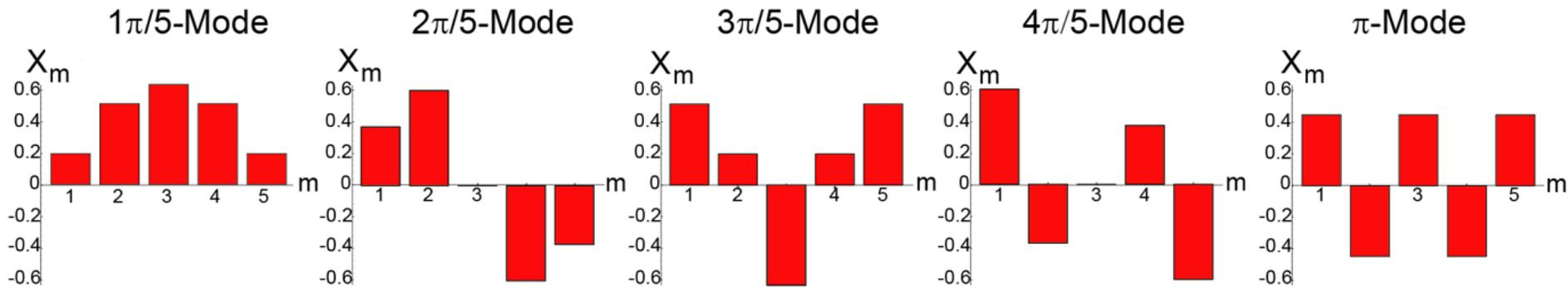
Numerical solution ( $TM_{010}$  passband – electric field contours)
