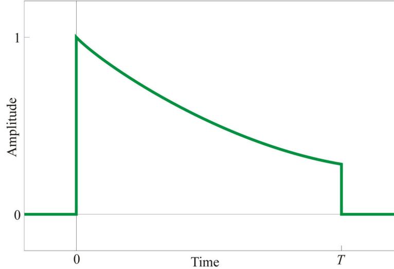
Figure 12 – The normalized filter hold function
