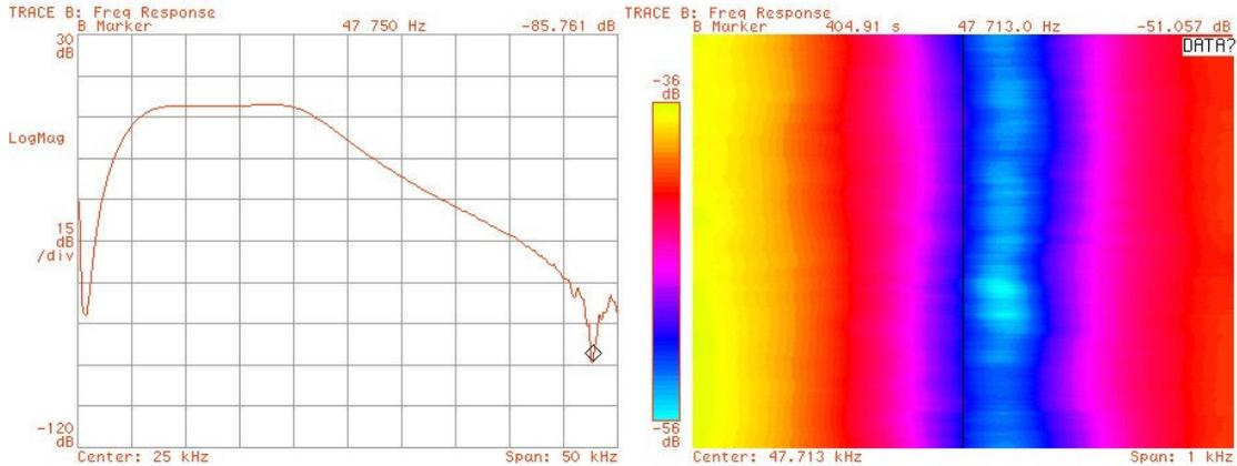
Figure 20 – To the left is a typical frequency response of the BBQ front end with a random noise input from an HP89410A VSA. The tunes in the Tevatron are generally within a couple of kHz of 19.5 kHz, near the edge of the plateau. The revolution frequency, 47.713 kHz, is about 90 dB below the betatron tunes. This attenuation will change to some extent since the band of highest attenuation is slightly higher than 47.713 kHz as shown in the spectrograph to the right.
