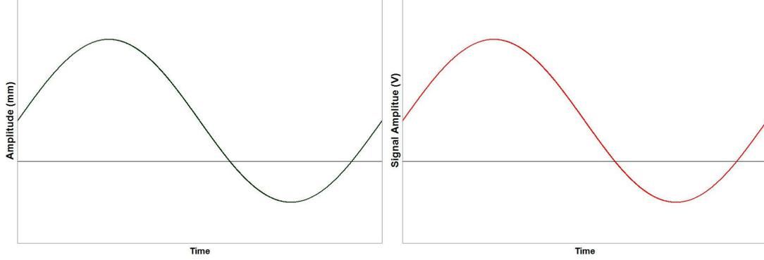
Figure 4 – The motion of a beam of charged particles as it passes a pair of pickups, shown to the left, results in a voltage variation that tracks the position of the beam resulting in a time-dependant potential signal,  $s_e(t)$ , shown to the right.
