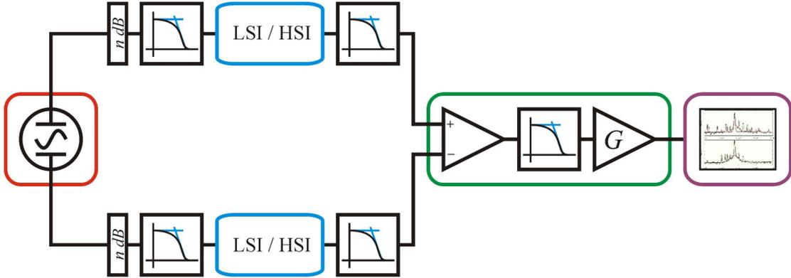
Figure 19 – The BBQ circuit including filters and attenuators. The attenuator is shown as an “ $n$  dB” pad before any pre-diode box filtering. 70 MHz low pass filters were generally employed prior to the diode boxes to maximize the diode bandwidth. As suggested, there may also be filtering between the diode box and front end to further attenuate the revolution frequency, which were not used.
