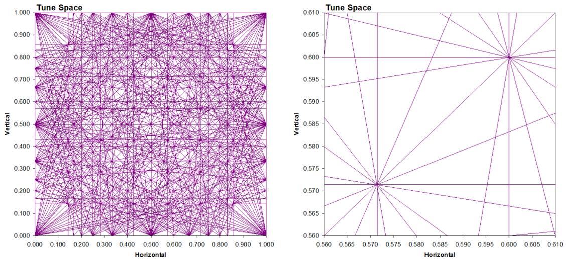
Figure 2 – Tune-space resonance plots showing resonances up to 7<sup>th</sup> order. The plot on the left shows the entire harmonic tune space while the plot on the right shows a detail the typical tune space of the tunes in the Tevatron, from 0.575 to 0.595 in each plane. The lines on the plot represent potential points of instability with lower order resonances being most likely to result in an instability.
