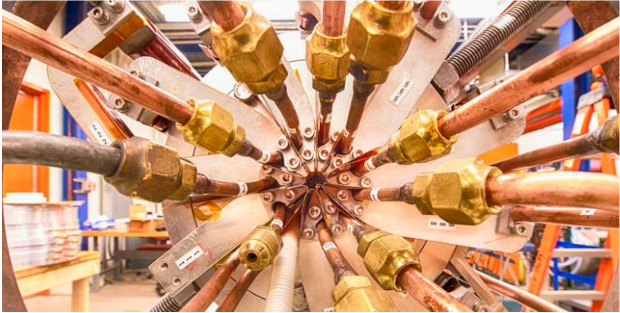
Figure 2-8 Photograph of a tuner's water cooled inner-package bus bars. Photo credit: Fermilab.gov
