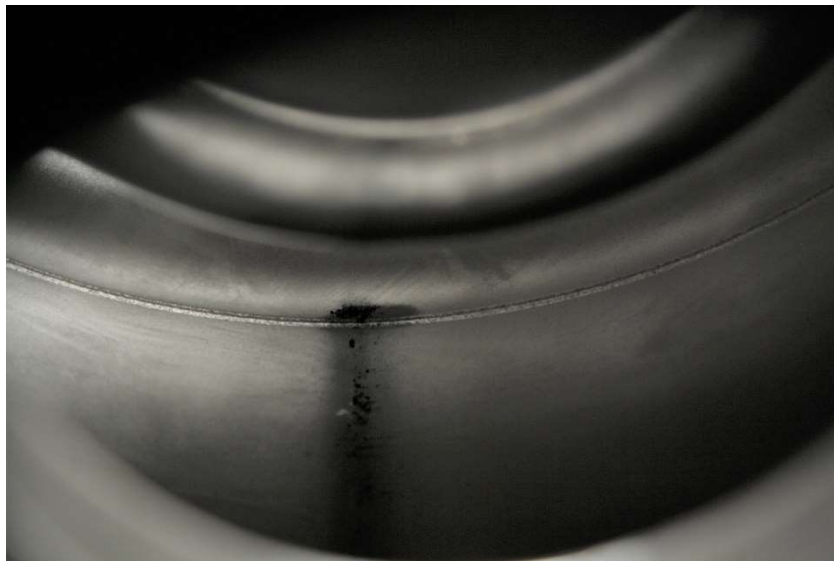
Figure 37. Photograph of contamination on the bottom of the WIFEL SRF cavity (image taken looking into beamport).
