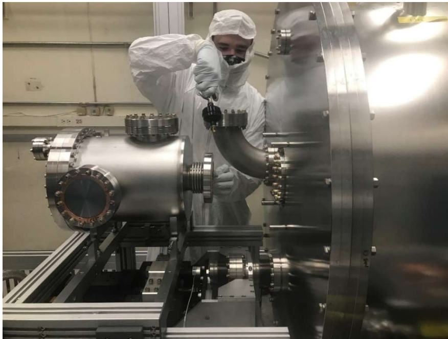
Figure 13. The coupling cavity (with damage beamline bellows) being removed in the clean room.
