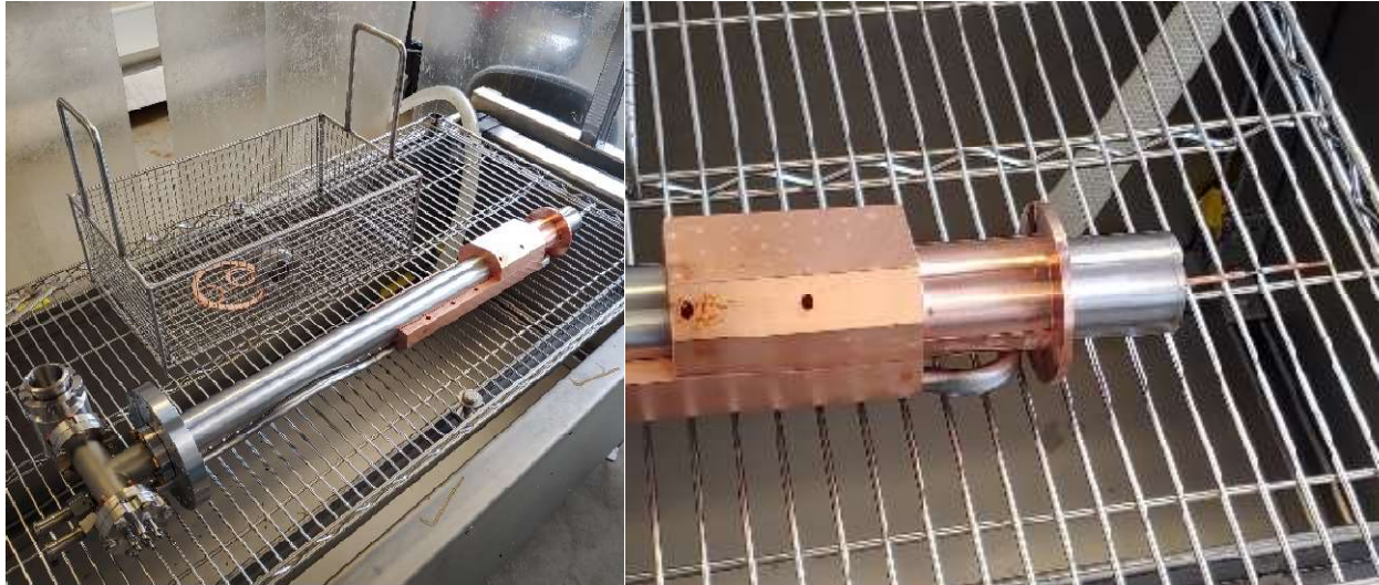
Figure 17. RF field probe assembly post-cleaning (left), close up of antenna at the end of the assembly (right)
