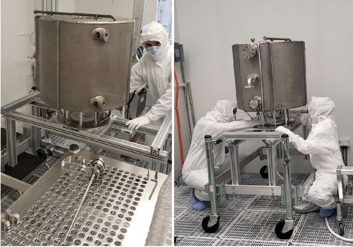
Figure 67. WIFEL cavity, beamport down, on a turntable in the clean room before rinsing with the short HPR wand used for this cleaning visible in the foreground (left). Wand placement and alignment in cavity (right).
