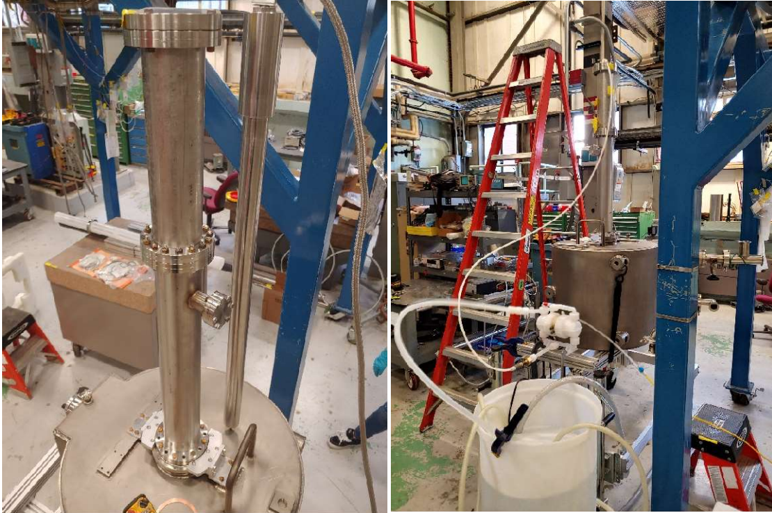
Figure 66. Ultrasonic cleaning setup for the WIFEL cavity, with the transducer suspended from an overhead crane (left). The ultrasonic transducer is suspended by a crane while submerged into the water, and a pumping setup was used to transfer DI water into and out of the cavity (right).
