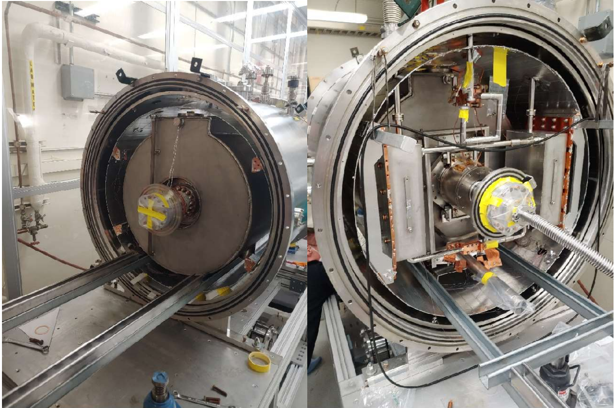
Figure 72. The WIFEL cavity in the process of being slid into the cryostat just outside of the cleanroom.
