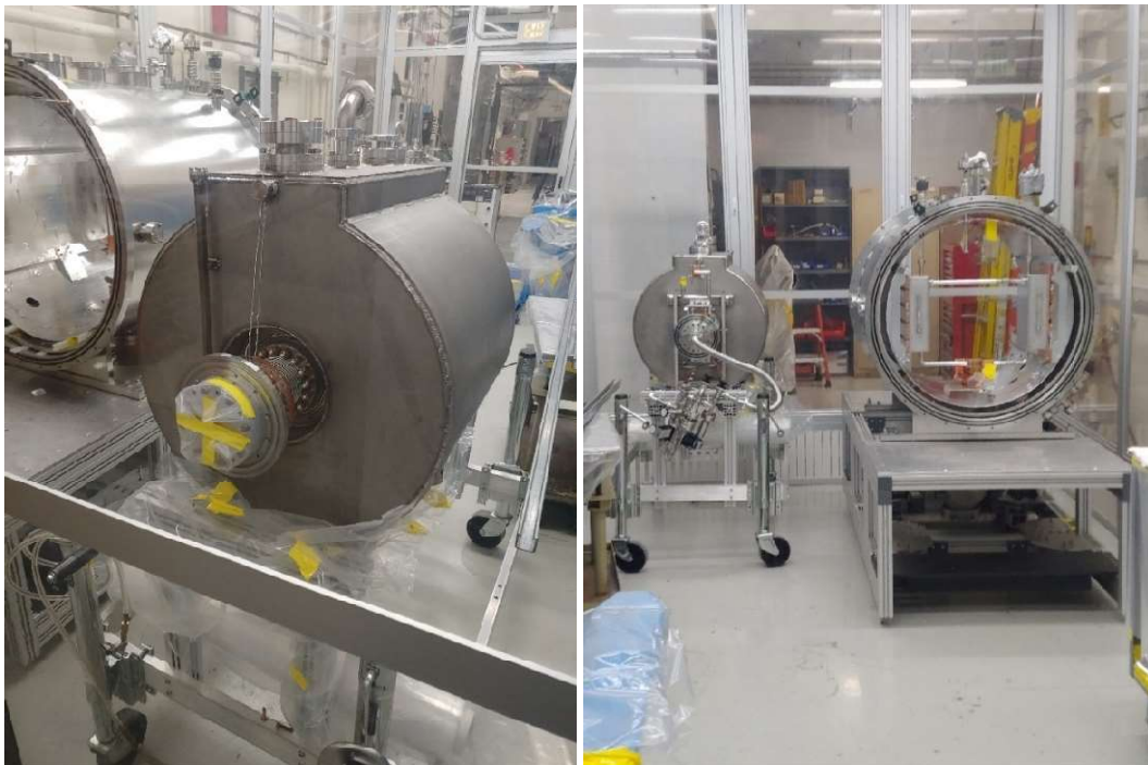
Figure 70. WiFEL cavity with cathode and anode side flanges (along with superconducting solenoid) prepped for assembly into the cryostat.
