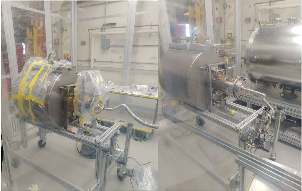
Figure 68. WiFEL cavity on its cart in the ATLAS clean room. RF space is sealed with the flexible hose connected to the “up-to-air” system (left). Cavity with solenoid support removed and “up-to-air” system tied to the cart (right).
