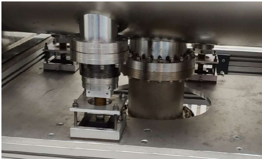
Figure 72. The WIFEL cavity in the process of being slid into the cryostat just outside of the cleanroom.
