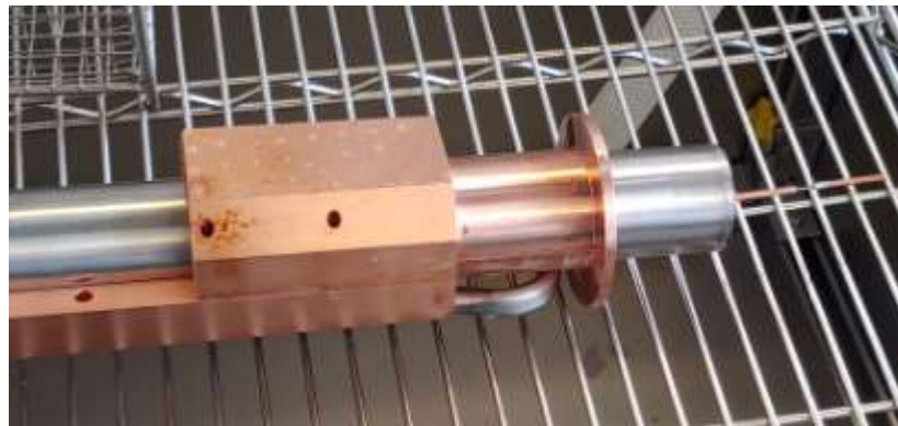
Figure 30. Close-up of RF pickup structure with potentially suspect features.
