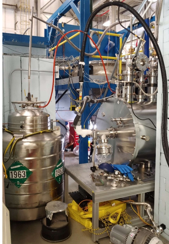
Figure 40. WiFEL cryostat in cave during cooldown post-cleaning. A helium dewar was used to help during the cooldown process.
