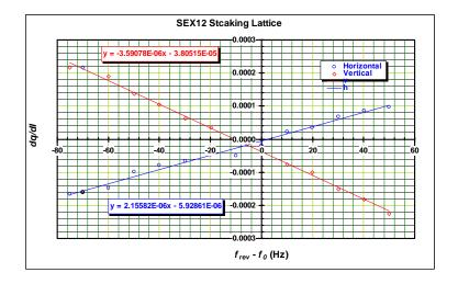
Figure 4.2. Fits to  $\frac{dq}{dI}$  curves for the sextupoles in the Ax12 locations on the stacking lattice.
