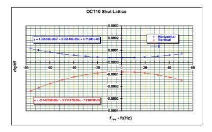
Figure 4.16. Fits to  $\frac{dq}{dI}$  curves predicted by the model for the octupoles in the Ax10 locations on the shot lattice.
