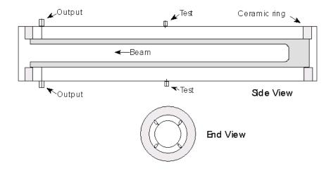
Figure 1.7. Diagram of a Schottky detector.
