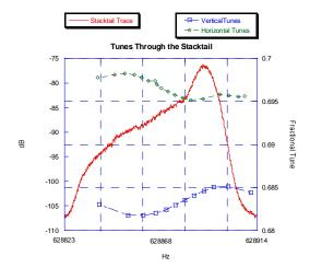
Figure 3.4. The red trace is the longitudinal Schottky stack signal. The stacktail extends from the core region to  $^{\circ}628830Hz$ , near the central orbit. The green trace is the calculated horizontal tunes. The blue trace is the calculated vertical tunes.
