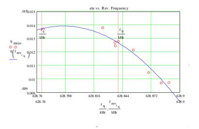
Figure 4.5. Calculated fit to the measured  $\eta$  at various revolution frequencies on the stacking lattice.
