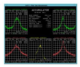
Figure 1.9. Spectrum analyzer display of a core revolution frequency fractional tune measurement.
