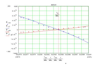
Figure 4.6. Model predictions compared to measured  $\frac{dq}{dI}$  data for sextupoles in the Ax10 locations on the stacking lattice.
