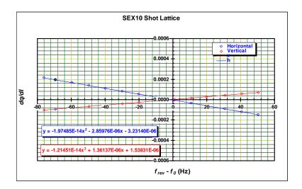
Figure 4.14. Fits to  $\frac{dq}{dI}$  curves predicted by the model for the sextupoles in the Ax10 locations on the shot lattice.
