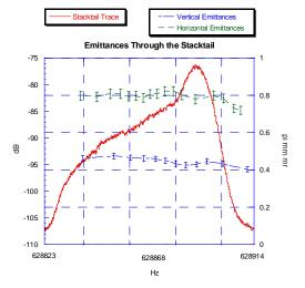
Figure 3.5. The red trace is the longitudinal Schottky stack signal. The green trace is the calculated horizintal emittances. The blue trace is the calculated vertical emittances.
