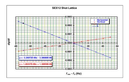
Figure 4.15. Fits to  $\frac{dq}{dI}$  curves predicted by the model for the sextupoles in the Ax12 locations on the shot lattice.
