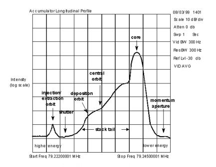
Figure 1.1. Spectrum Analyzer trace of a signal from a longitudinal Schottky detector showing the Accumulator momentum aperture during atiproton stacking.
