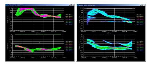
Figure 2.4. The plot on the left is the measured tunes before the corrections were applied. The plot on the right is the tunes after the corrections were applied. The algorithms predicted that the horizontal tunes should be lower by ~0.005 units near the core and injection frequencies. The algorithms predicted that the vertical tunes should be higher by ~0.010 units near the core and by ~0.010 near the injection frequencies. The measurements agree with the predictions.
