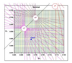
Figure 1.10. The horizontal and vertical fractional tune with respect to resonance lines. The x axis is the fractional horizontal tune. The y axis is the fractional vertical tune.
