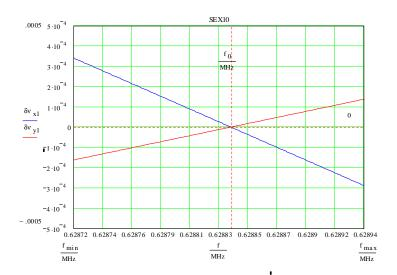
Figure 4.10. Model prediction  $\frac{dq}{dI}$  curves for sextupoles in the Ax10 locations on the shot lattice.
