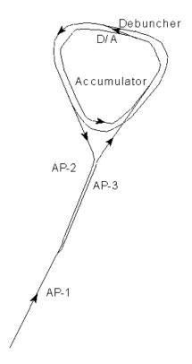
Figure 1.5. Path of protons in reverse proton mode.
