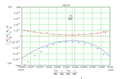
Figure 4.8. Model predictions compared to measured  $\frac{dq}{dI}$  data for octupoles in the Ax10 locations on the stacking lattice.
