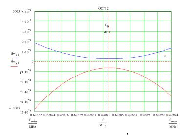
Figure 4.13. Model prediction  $\frac{dq}{dI}$  curves for octupoles in the Ax12 locations on the shot lattice.
