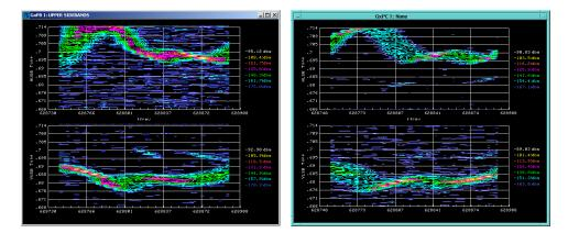
Figure 2.1. Horizontal and vertical sideband tunes. The vertical axis show the fractional tune value between the two-thirds and five-sevenths resonances. The horizontal axis shows the Accumulator revolution frequency. The injection frequency is 628765 Hz and the core revolution frequency is 628888 Hz. 90% of the peak signal strength and 20 contours are plotted. The plot on the left are the upper sidebands. The plot on the right are the lower sidebands.
