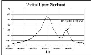
Figure 3.1. Coupling at the core revolution frequency. The plot on the left shows the vertical sideband as seen on the horizontal Schottky detector display. The plot on the left shows the horizontal sideband as seen on the vertical Schottky detector display.
