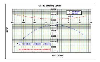
Figure 4.3. Fits to  $\frac{dq}{dI}$  curves for the octupoles in the Ax10 locations on the stacking lattice.
