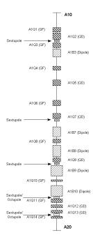
Figure 1.2. Accumulator lattice for the A10 sector. This represents one-sixth of the ring. The A20 sector is mirror symmetric.
