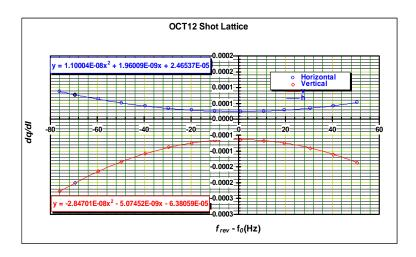
Figure 4.17. Fits to  $\frac{dq}{dI}$  curves predicted by the model for the octupoles in the Ax12 locations on the shot lattice.
