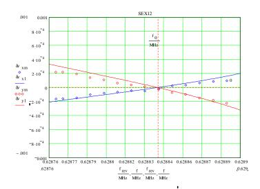
Figure 4.7. Model predictions compared to measured  $\frac{dq}{dI}$  data for sextupoles in the Ax12 locations on the stacking lattice.
