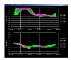
Figure 2.2. Upper horizontal and vertical sideband tunes. 70% of the peak signal strength and 50 contours are plotted.
