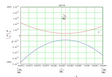
Figure 4.12. Model prediction  $\frac{dq}{dI}$  curves for octupoles in the Ax10 locations on the shot lattice.
