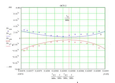
Figure 4.9. Model predictions compared to measured  $\frac{dq}{dI}$  data for octupoles in the Ax12 locations on the stacking lattice.
