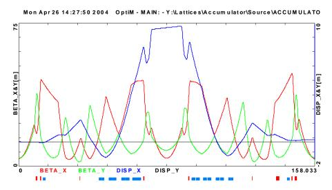
Figure 1.3. Plot of the beta and dispersion funtions for 2 sectors of the Accumulator. The red trace is  $\beta_x$ . The green trace is  $\beta_y$  and the blue trace is  $D_x$ .
