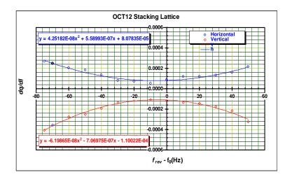
Figure 4.4. Fits to  $\frac{dq}{dI}$  curves for the octupoles in the Ax12 locations on the stacking lattice.
