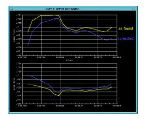
Figure 2.3. Tune measurements and correction predictions. The yellow trace shows the measured peak tune values for each scan point. The blue curve shows the change to the tunes predicted by the correction algorithms.
