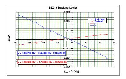
Figure 4.1. Fits to  $\frac{dq}{dI}$  curves for the sextupoles in the Ax10 locations on the stacking lattice.
