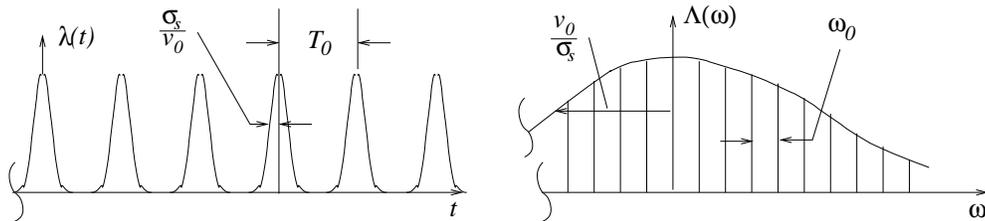
FIGURE 4.3. Time domain and frequency domain signals from an on-axis Gaussian-distributed, bunch of length  $\sigma_s$ .
