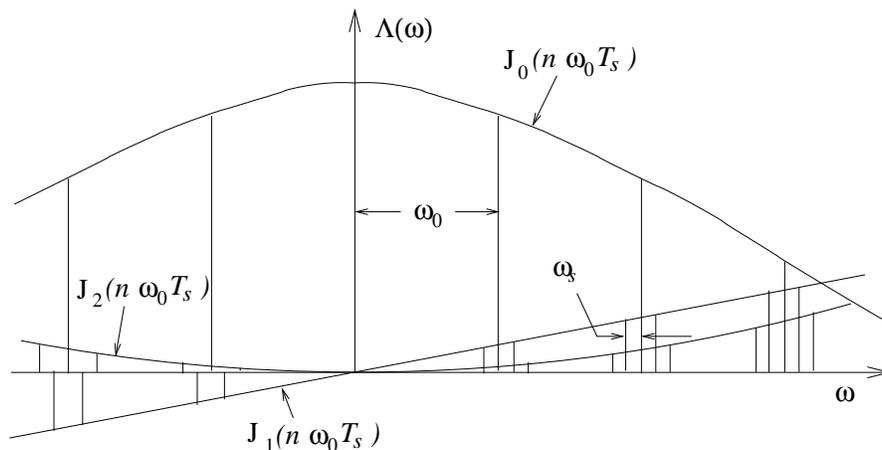
FIGURE 4.4. Spectrum of BCM signal due to a single particle executing longitudinal oscillations.
