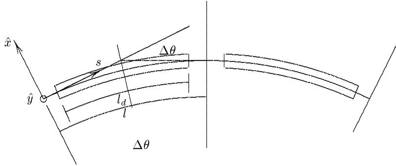
FIGURE 6.2. Geometry for transition gamma calculation.
