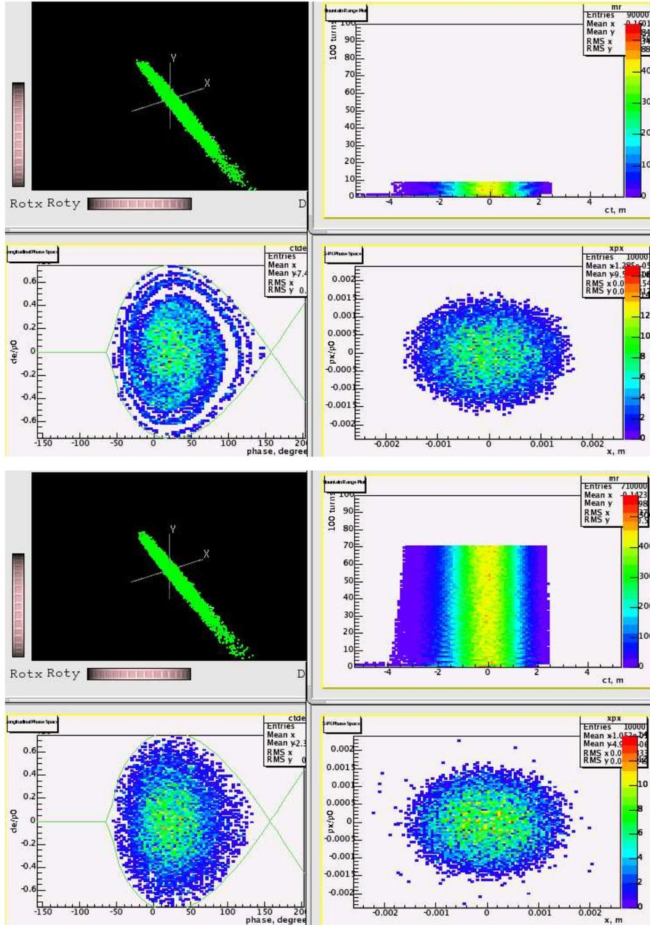
FIGURE 6.5. Top: Particle distribution 800 turns after injection of the same beam. Bottom: Particle distributions 7000 turns after injection of the same beam.
