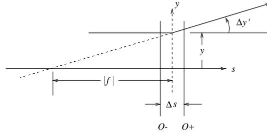
FIGURE 2.4. Focusing action of a thin lens for which the focusing strength-length product is  $K\Delta s$  and fields outside the range  $O_- < s < O_+$  can be neglected. The “focal length” is  $f = -(K\Delta s)^{-1} \equiv -q^{-1}$ .
