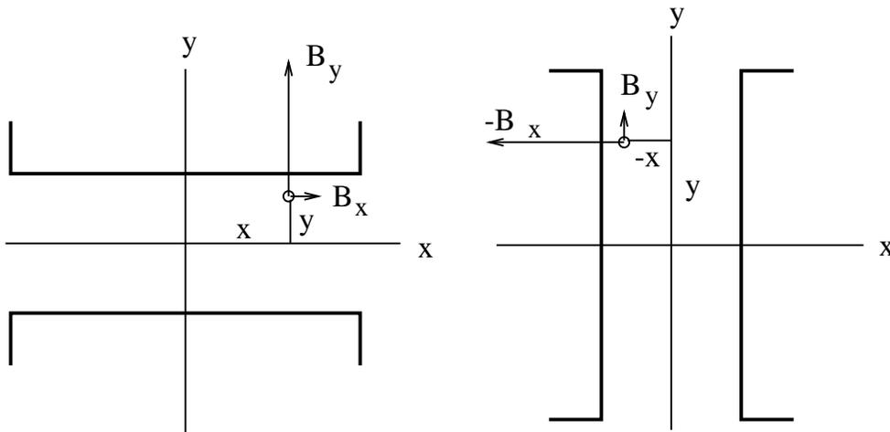
FIGURE 8.1. A horizontal steering dipole and the same magnet rotated so that it steers vertically. The median-plane field and its multipole approximation is shown in FIG 8.2. The analytic description of the rotated fields is given in the text.
