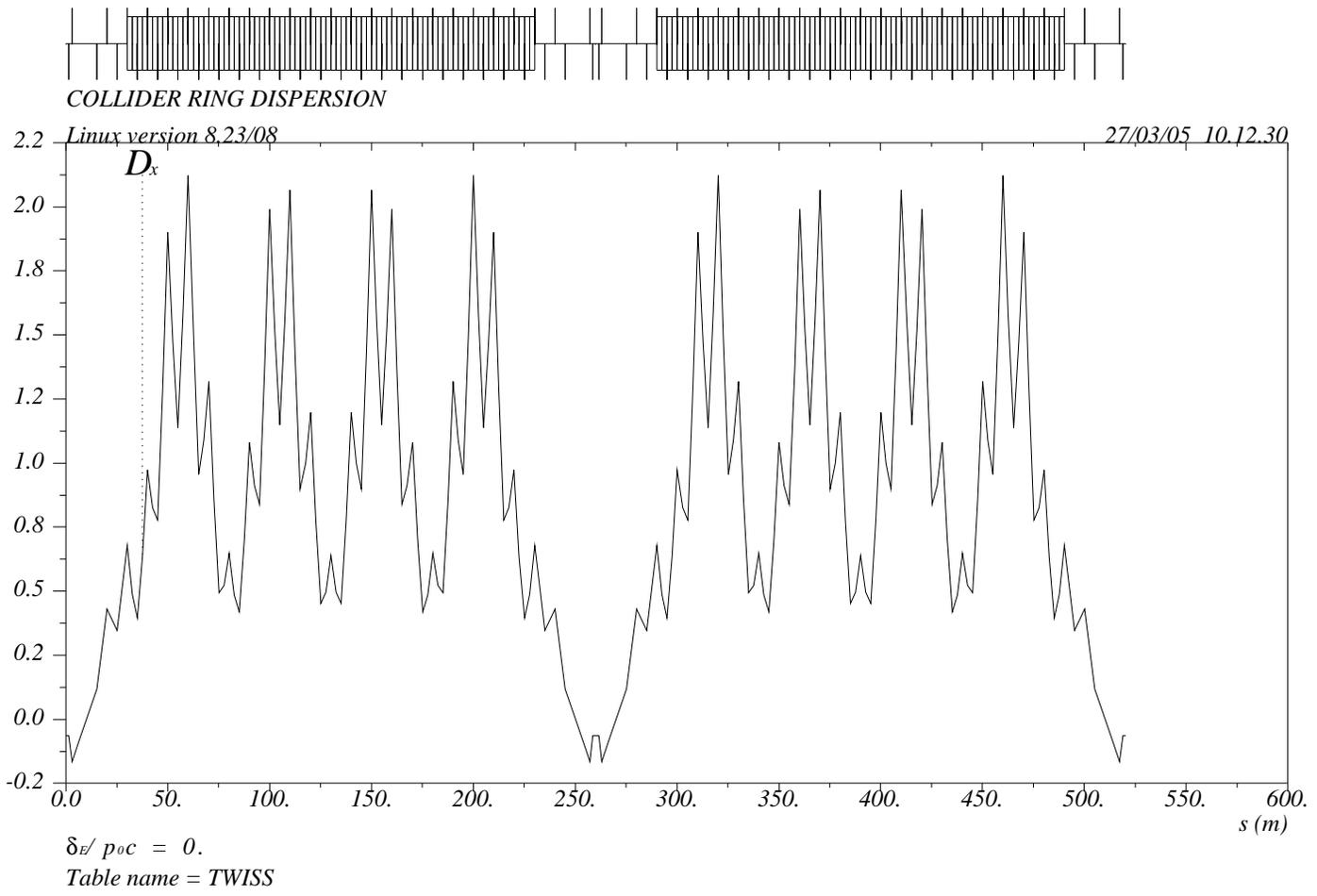
FIGURE 9.3. Dispersion function for the collider lattice.
