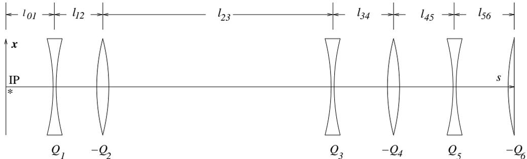
FIGURE 9.1. Lengths and strengths of intersection region optical elements. Lens symbols and quad strengths appropriate for horizontal (convex is focusing) are shown and all  $Q_i$  are positive.
