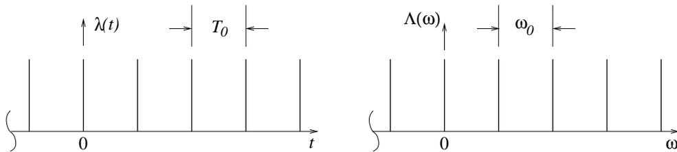
FIGURE 4.2. Time domain and frequency domain signals from a point reference particle.
