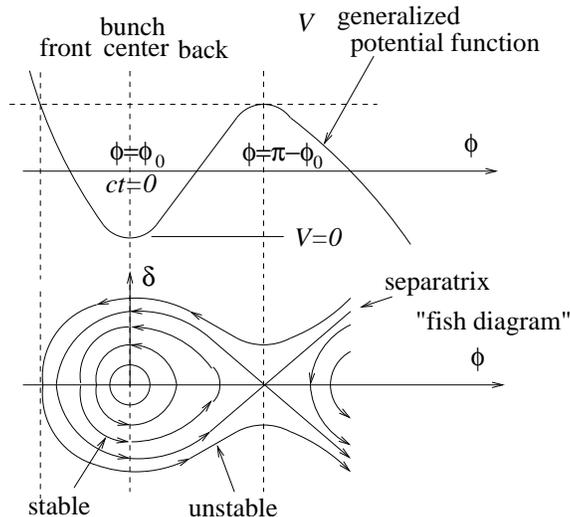
FIGURE 6.1. "Fish diagram" of longitudinal phase space motion. On passing through transition the pattern is right-left reflected. i.e. the fish points in the opposite direction.
