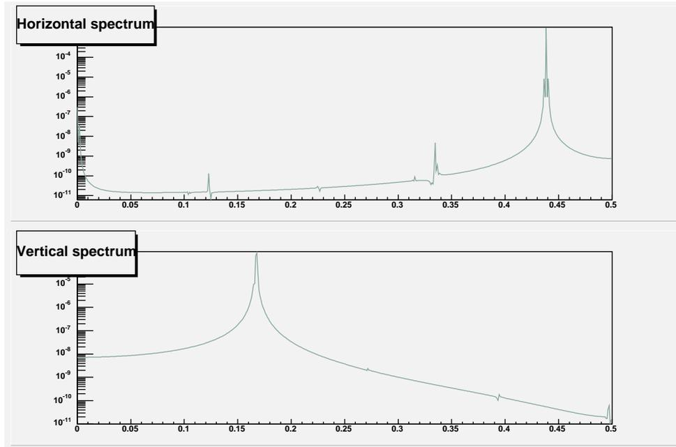
FIGURE 4.6. Horizontal and vertical tune spectra for the `collider_mon` lattice.
