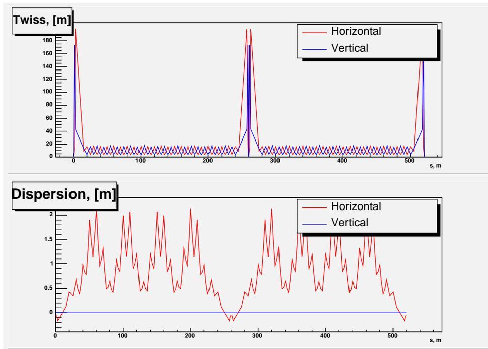
FIGURE 4.1. Lattice functions for the `collider_mon` lattice, obtained using the matrix method of Chapter 2.
