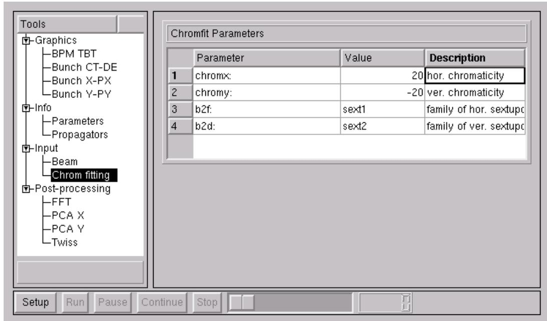
FIGURE 7.7. Simulator window used for adjusting chromaticities.
