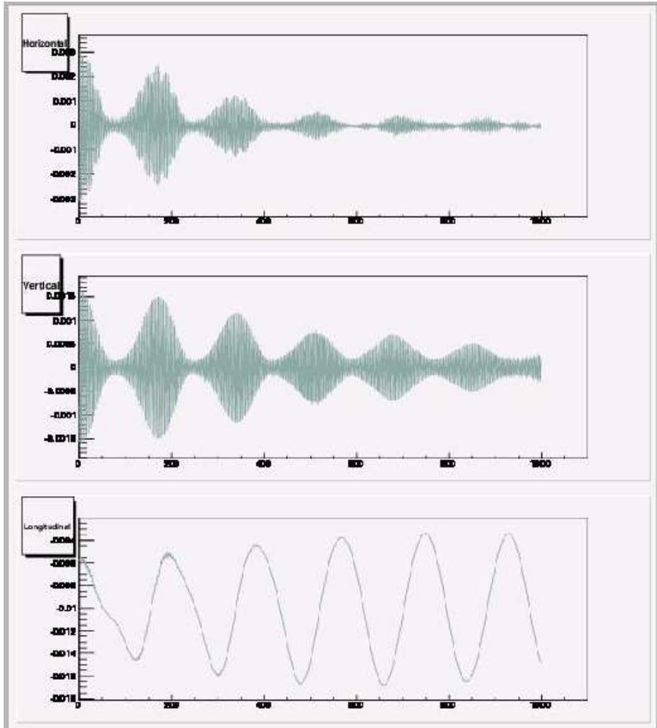
FIGURE 7.6. Beam echos observed one synchrotron period (and multiples thereof) after a beam is kicked both horizontally and vertically in the racetrack lattice.  $Q'_x = 20$ ,  $Q'_y = -20$ .
