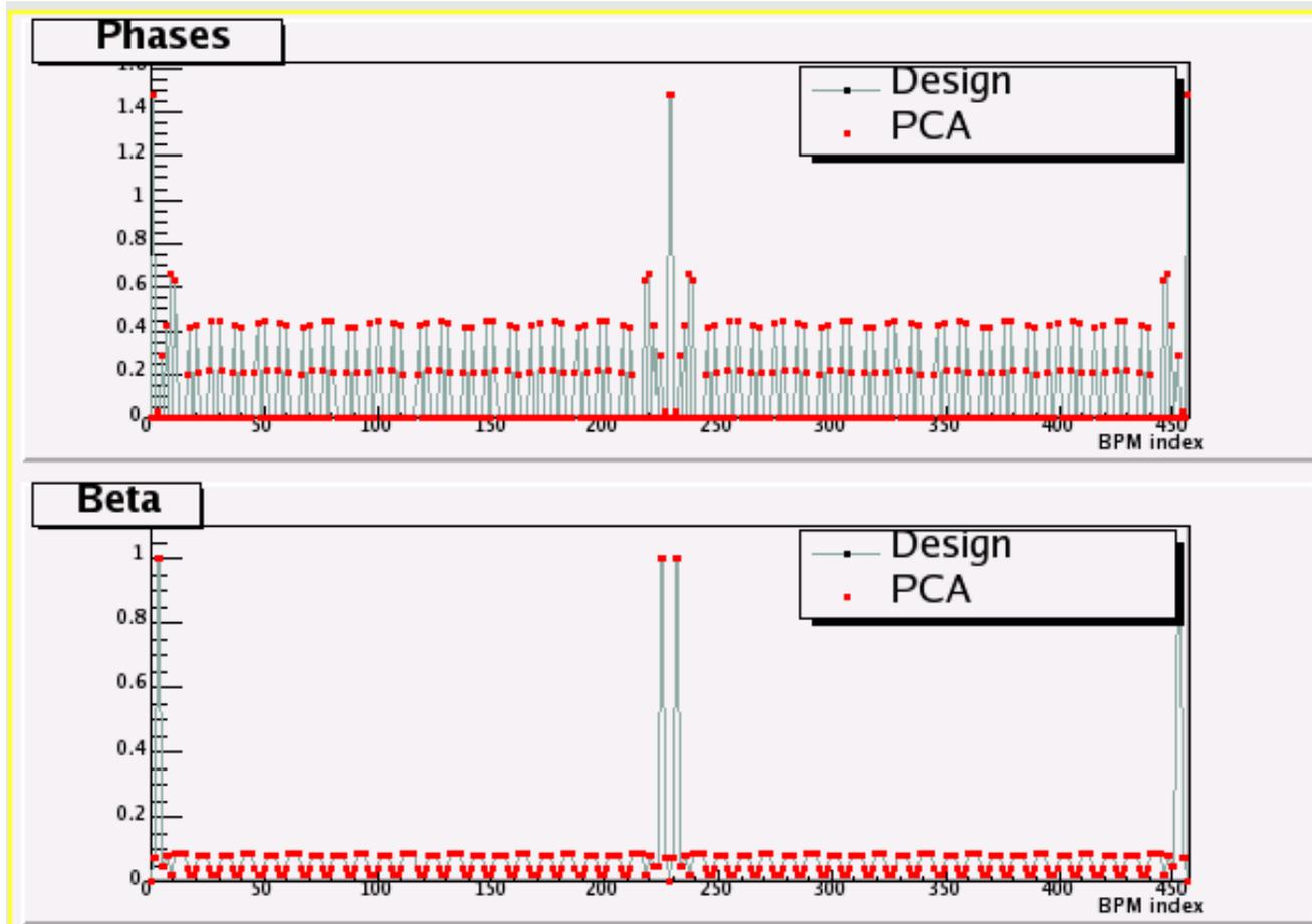
FIGURE 4.9. Twiss function and phase advances derived for the `collider_mon` lattice using the PCA simulator. Bold dots superimposed on curves indicate agreement between model-independent and model-based determinations.
