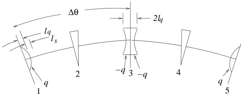
FIGURE 8.3. Labeling of points in a full cell of the `eq_tune_fodo` lattice.
