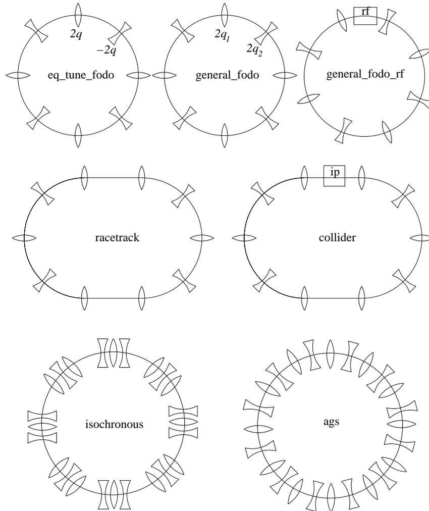
FIGURE 1.1. "Toy lattices" to be used as starting points for accelerator simulations. Note: "ags" is *not* a "toy".
