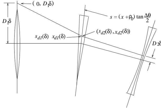
FIGURE 6.3. Geometry for calculation of off-momentum, polygonal path length. The on-momentum and off-momentum orbits are shown. The bending magnet is represented by a prism symbol.
