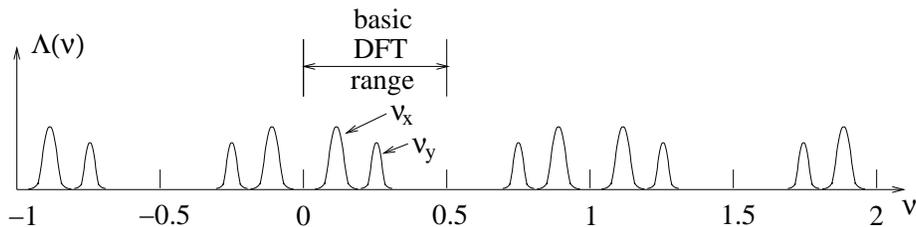
FIGURE 4.5. Cartoon showing spectrum extracted from single plane BPM. Due to coupling both horizontal and vertical tune lines are visible. There is aliasing to all integer tune ranges as well as reflection above and below integers.
