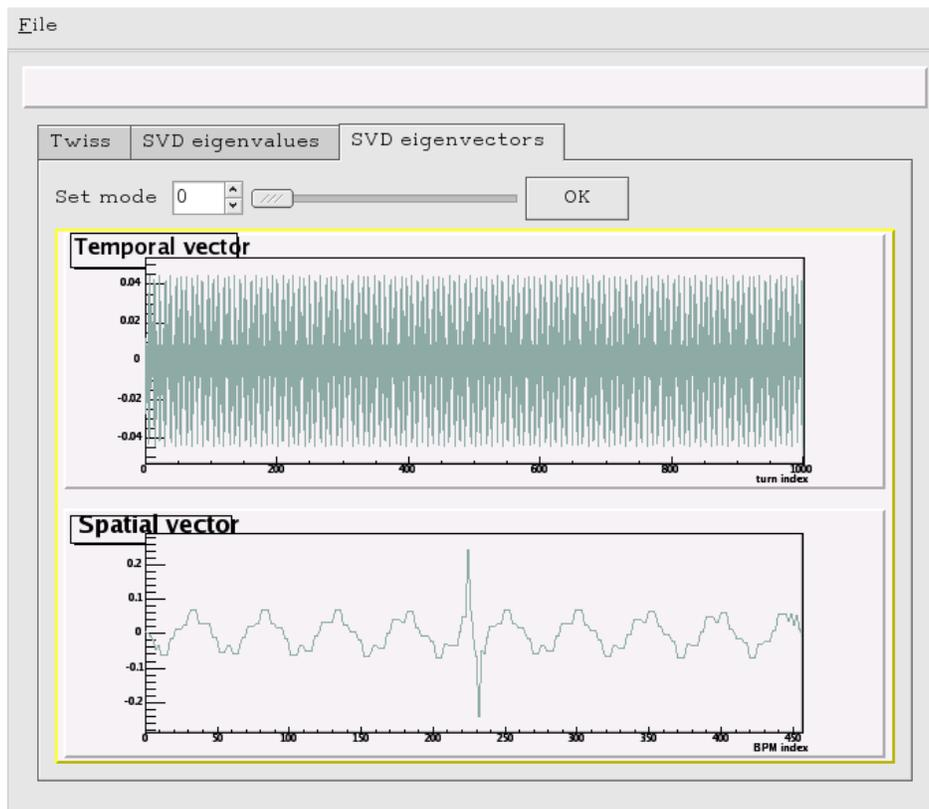
FIGURE 4.8. Spatial and temporal SVD eigenvectors derived from the PCA simulation of the collider\_mon lattice are exhibited.
