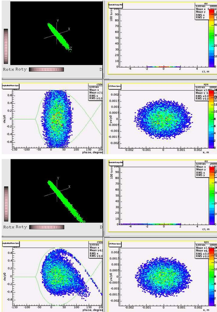
FIGURE 6.4. Top: Particle distribution just after injection of slightly over-sized 10000 particle beam. Bottom: Particle distributions 100 turns after injection of the same beam. Counterclockwise, starting at upper left, the figures are 3D space, longitudinal phase space, transverse phase space, and turn number vs. longitudinal.
