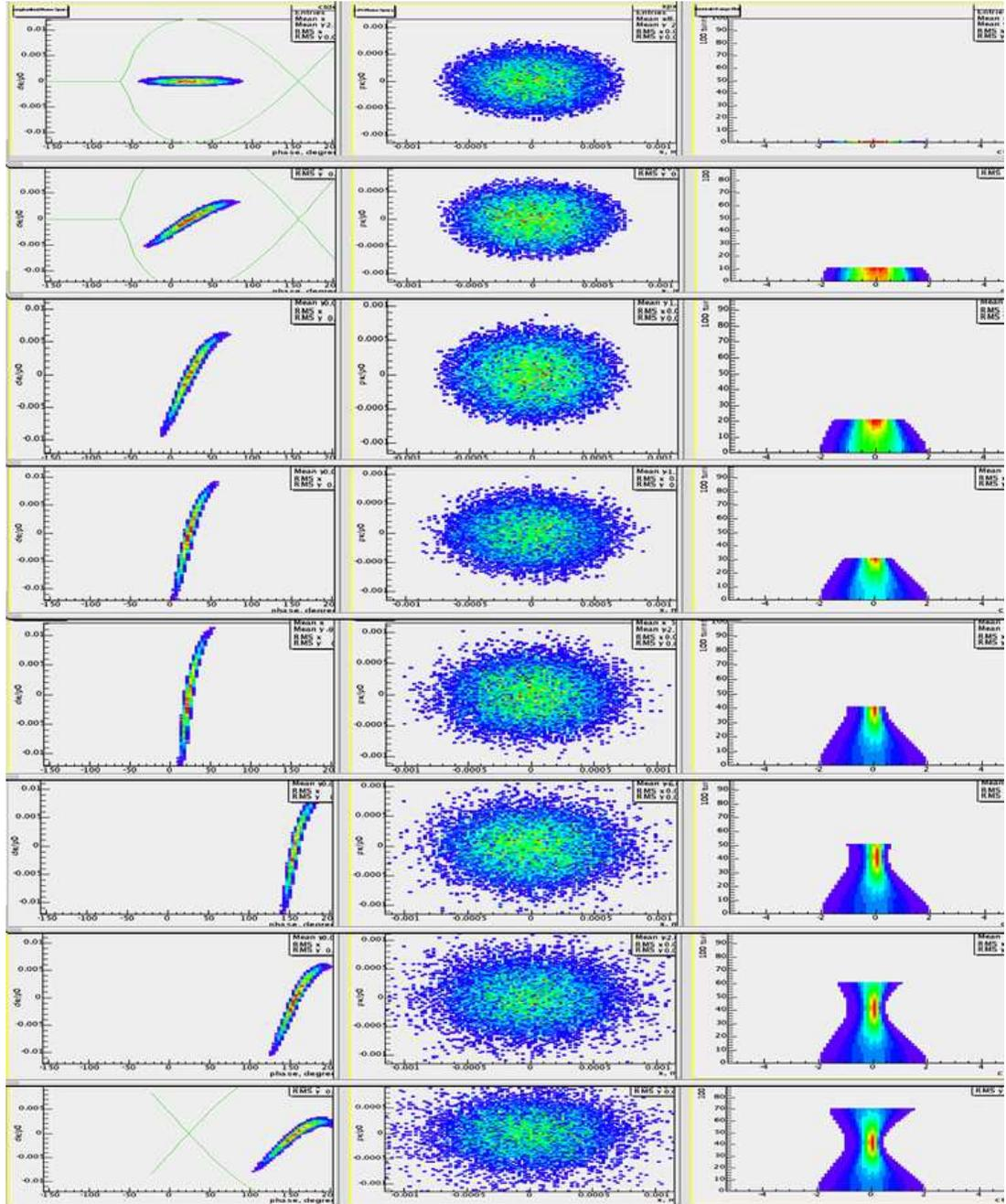
FIGURE 6.6. Series of distribution snapshots (every 1000 turns for a beam of 10000 particles) starting just before, and ending just after transition. The RF phase is jumped at the instant of transition crossing.
