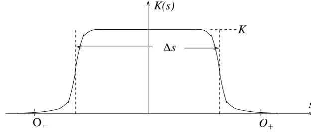
FIGURE 2.3. Realistic thin lens focusing profiles are more or less constant with value  $K$  over a central region and become negligible outside points  $O_-$  and  $O_+$ . Effective length  $\Delta s$  is determined by matching  $K\Delta s$  to the “field integral”.
