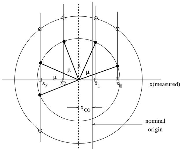
FIGURE 5.1. Geometric construction indicating how tune and closed orbit can be found from measuring the transverse displacement for several successive turns. Open square symbols are measured. Solid circle symbols lie on and define the correct phase space circle. Open circles lie on a candidate, but wrong, phase space circle.
