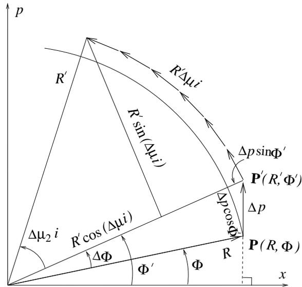
FIGURE 7.3. Evolution with turn number  $i$  of a point  $\mathbf{P}$  in betatron (horizontal) phase space, as viewed from a frame rotating at nominal phase advance per turn  $\mu_0$ . The trigonometry of this figure only makes sense for small perturbations ( $\Delta p \ll R$ ) which is assumed.
