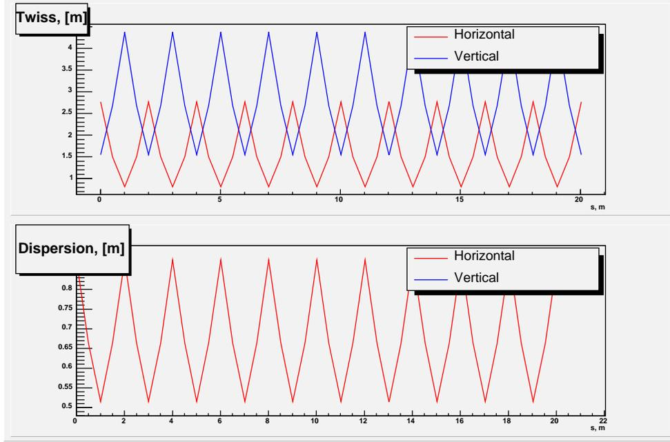
FIGURE 3.3. Lattice functions for the `general_fodo` lattice, with `nhalf=20`, `celltnxi=0.2`, `celltnyi=0.1`.
