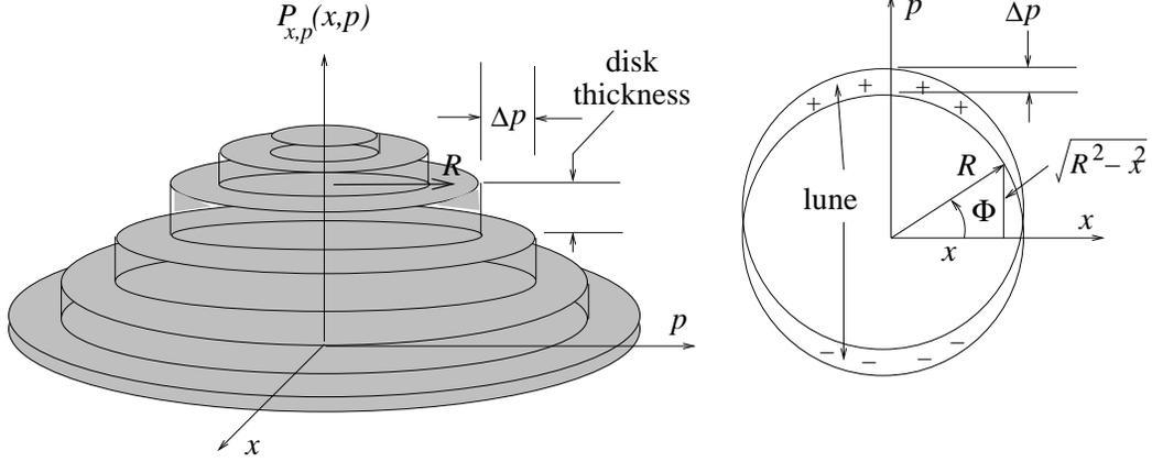
FIGURE 7.4. On the left the betatron phase space distribution is visualized as a sum of distributions, uniform over disks of radii successively changing in steps of  $\Delta p$ . This permits deviations from the unkicked distribution to be represented by positive and negative distributions uniform over the “lunes” shown on the right.
