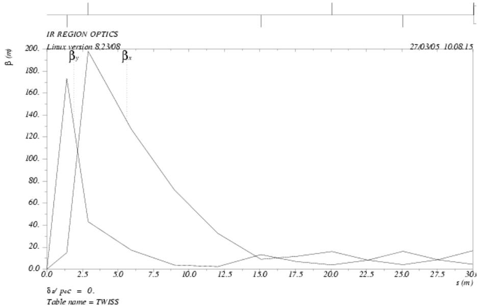
FIGURE 9.4. Twiss functions for the IR region of the collider lattice.
