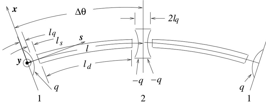
FIGURE 3.1. An idealized, thin lens, FODO lattice, showing dimensioning and element strength parameters.
