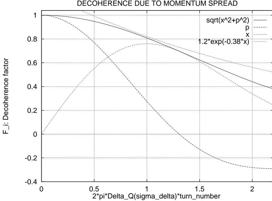
FIGURE 7.5. Time evolution of (fractional) centroid position  $x/\Delta p$ , slope  $p/\Delta p$ , and  $\sqrt{x^2 + p^2}/\Delta p$  after initial deflection  $\Delta p$ , viewed in a frame of reference rotating at the small amplitude tune, as given by Eqs. (7.23-7.25). An exponentially decaying function  $1.2 \exp(-0.38d_1\sigma_\delta i)$  is also shown for comparison.
