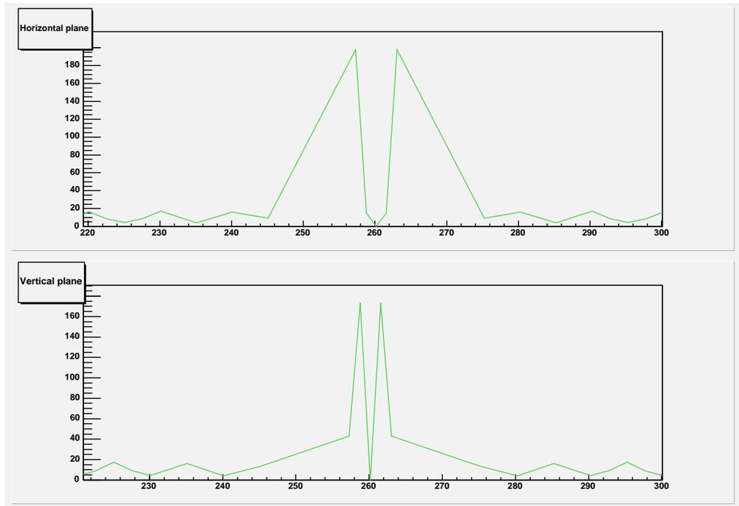
FIGURE 9.5. UAL-generated Twiss functions for the IR region of the collider lattice.
