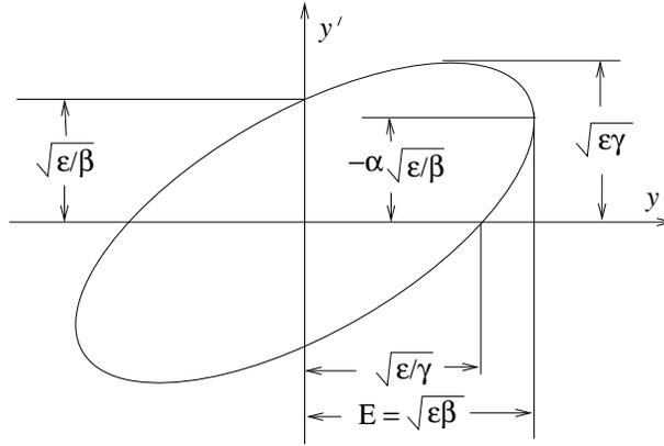
FIGURE 2.2. An elliptical beam in vertical phase space, showing the geometric configuration of a beam ellipse matched to the local Twiss parameters  $\alpha$ ,  $\beta$  and  $\gamma$ . Except for a factor of order 1, depending on the detailed beam distribution, the area of the ellipse is the emittance  $\epsilon$ . The skew orientation depends primarily on Twiss parameter  $\alpha$ .  $E$  is the “beam envelope”.
