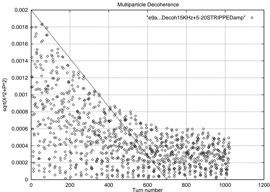
FIGURE 7.1. Multiparticle decoherence. Using the modeling program TEAPOT, an appropriately distributed “beam” consisting of 200 macroparticles,  $\sigma_E/E = 0.0006$ , is tracked for 1024 turns and the horizontal centroid coordinate is plotted each turn.
