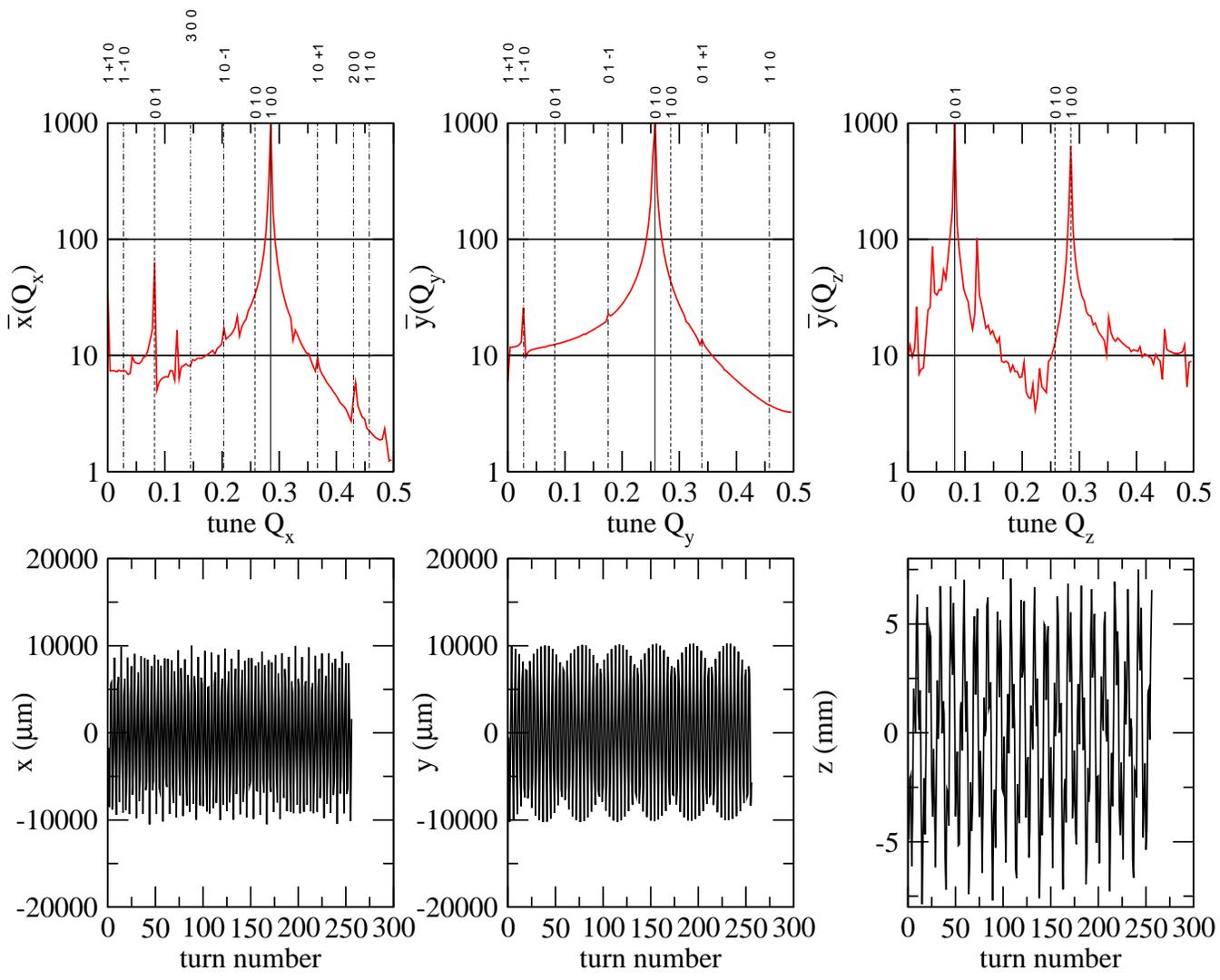
FIGURE 8.5. Turn-by-turn data, spectrum analysed, for collider rf lattice. Fractional tunes are  $Q_x = 0.26$ ,  $Q_y = 0.28$ ,  $Q_z = 0.08$ . Low order tune lines are labeled with  $m_x$ ,  $m_y$ , and  $m_z$  indices.
