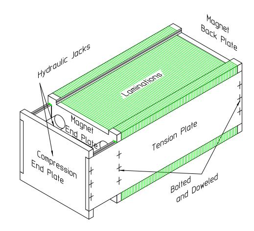
• After the compression, bolting and doweling, the Devcon, steel loaded epoxy is extruded in the v-groove space between the tension plates and the laminations.
