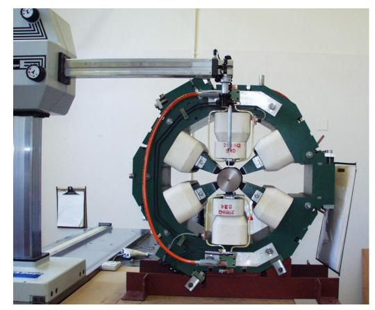
• The second photograph shows a quadrupole mounted on the CMM. The plate at the end of the poles is placed in contact with flats machined on the poles to establish the longitudinal end of the magnet. A mating plate is mounted at the opposite end of the magnet.
