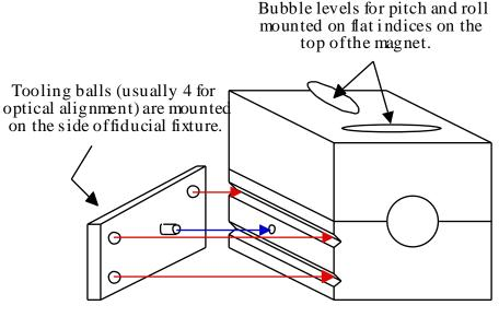
Three balls register in magnet v-grooves established by the lamination design.
