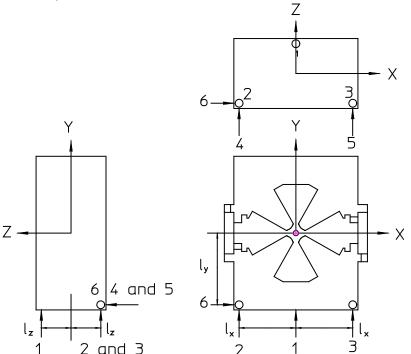
Each strut consists of a  $\bullet$ barrel, two rod ends and two locking collars. The rod ends are both right hand thread, but one is fine and the other is coarse. Therefore, each rotation of the barrel provides an adjustment equal to the difference in the pitches of the two threads.
